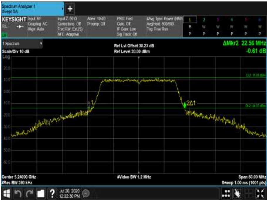
Figure 214 - 5240 MHz - 26 dB Emission Bandwidth
