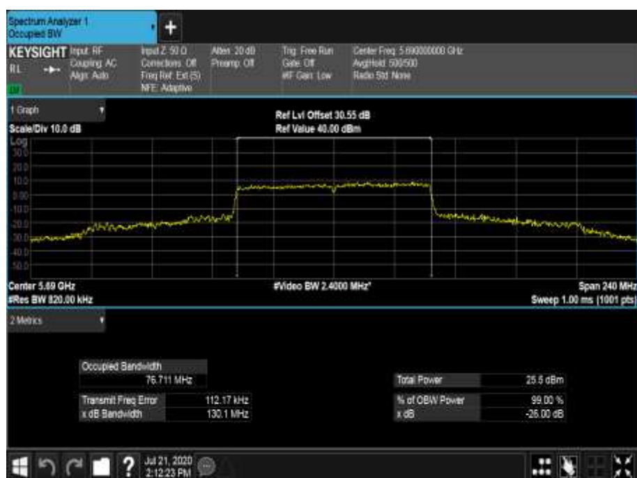
Figure 697 - 5690 MHz - 99% Occupied Bandwidth
