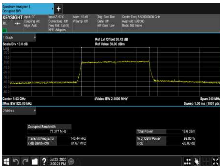
Figure 699 - 5530 MHz - 99% Occupied Bandwidth
