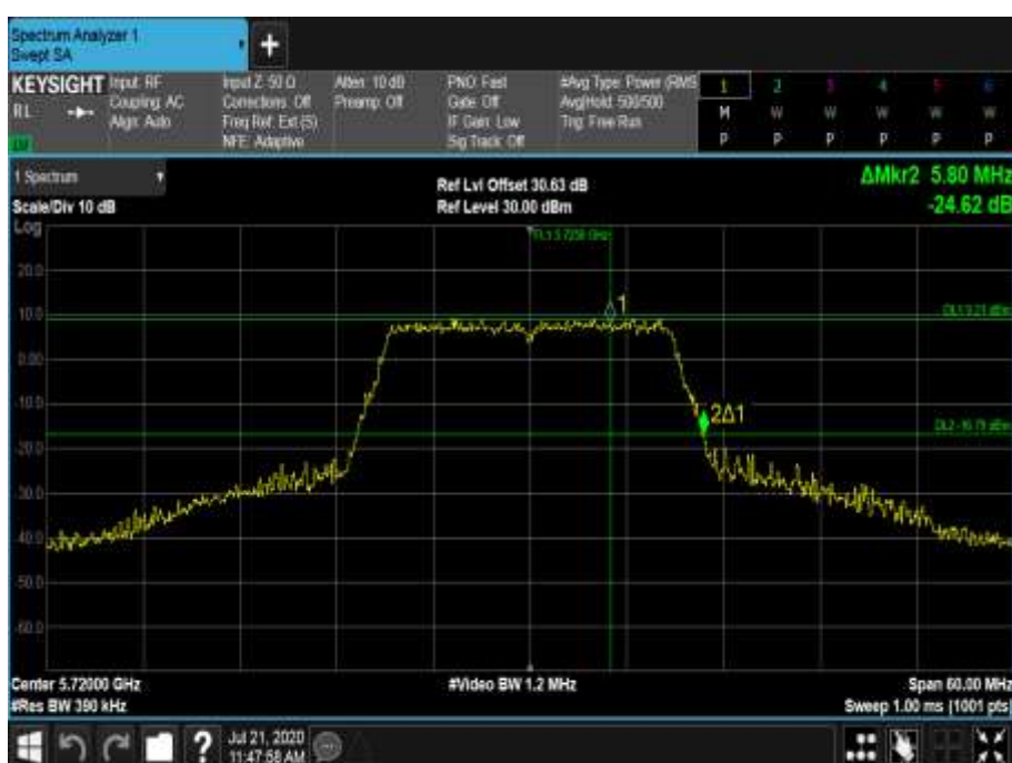
Figure 741 - 5720 MHz - 26 dB Emission Bandwidth
