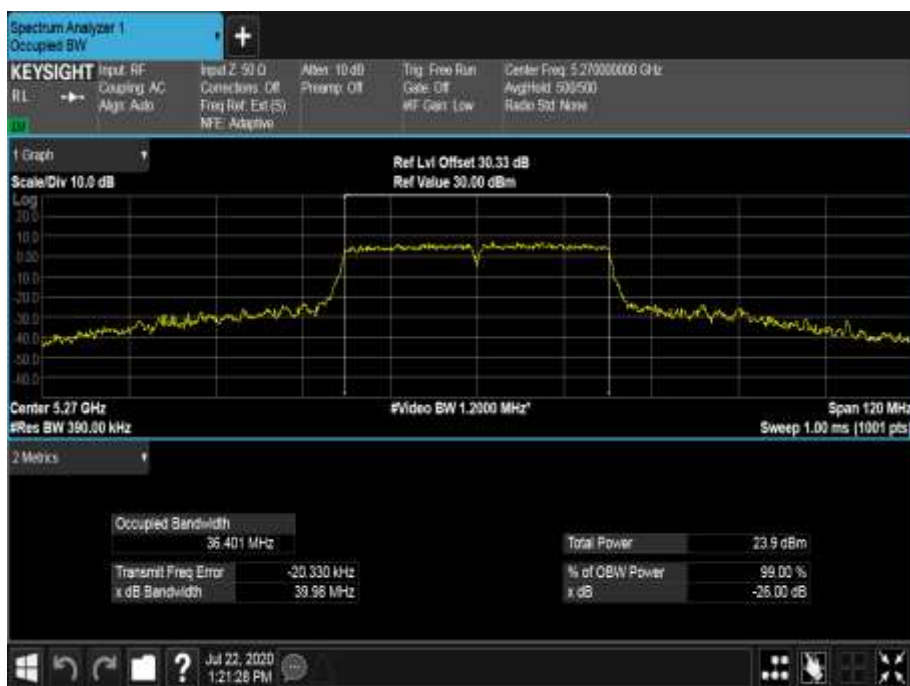
Figure 545 - 5270 MHz - 99% Occupied Bandwidth
