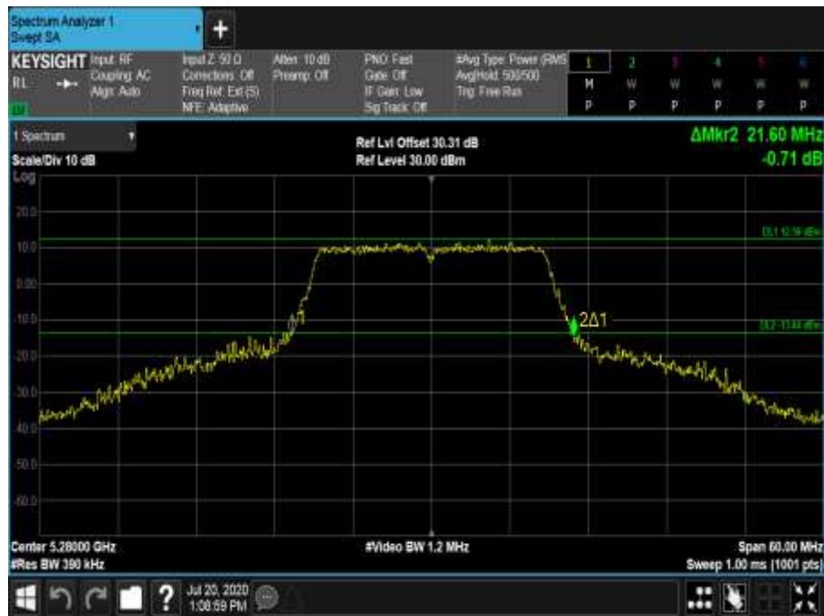
Figure 506 - 5280 MHz - 26 dB Emission Bandwidth
