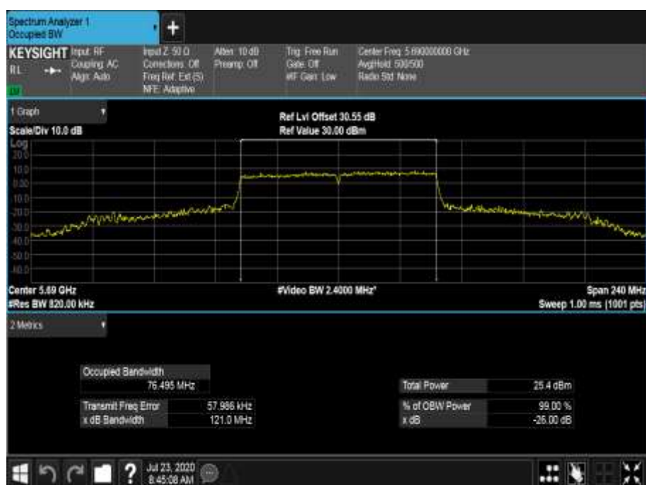
Figure 685 - 5690 MHz - 99% Occupied Bandwidth
