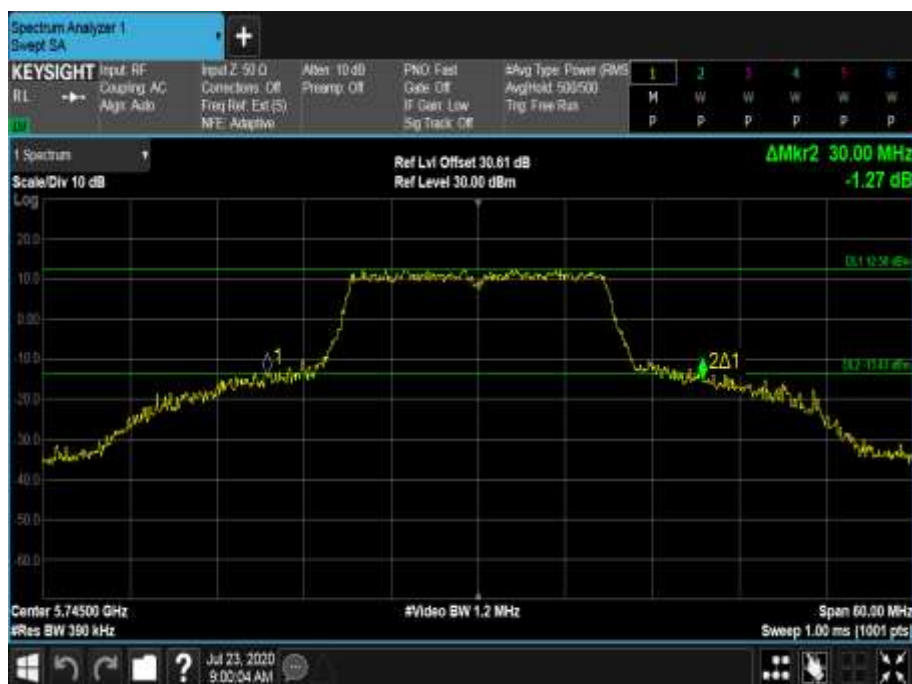
Figure 732 - 5745 MHz - 26 dB Emission Bandwidth
