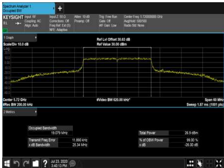
Figure 615 - 5720 MHz - 99% Occupied Bandwidth
