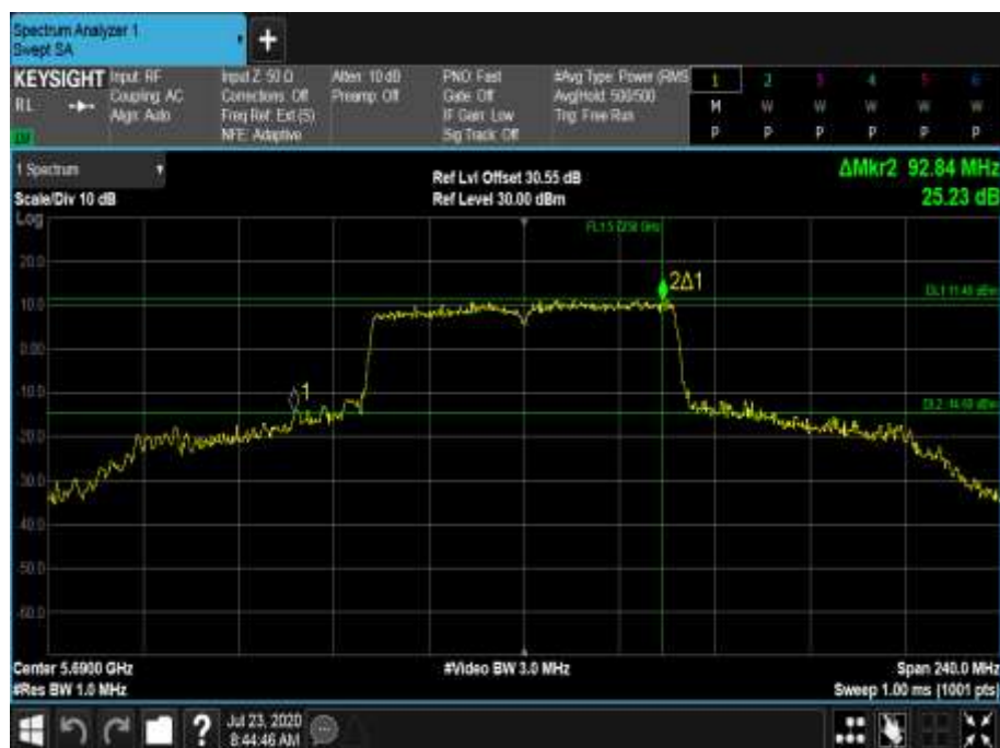
Figure 684 - 5690 MHz - 26 dB Emission Bandwidth
