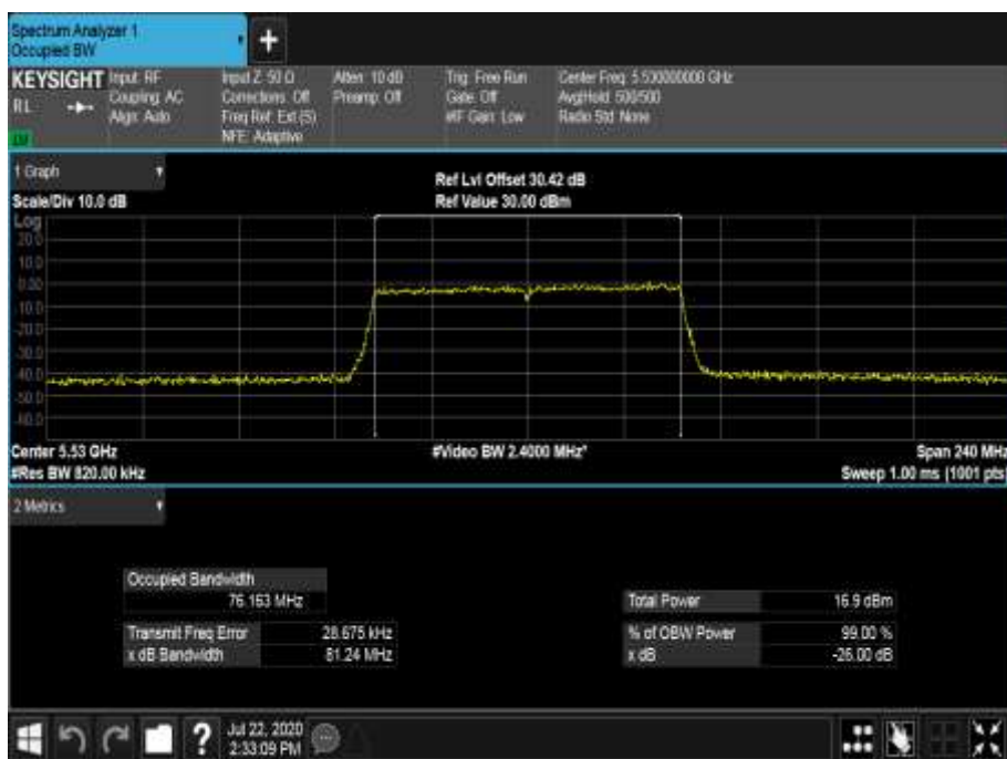
Figure 687 - 5530 MHz - 99% Occupied Bandwidth
