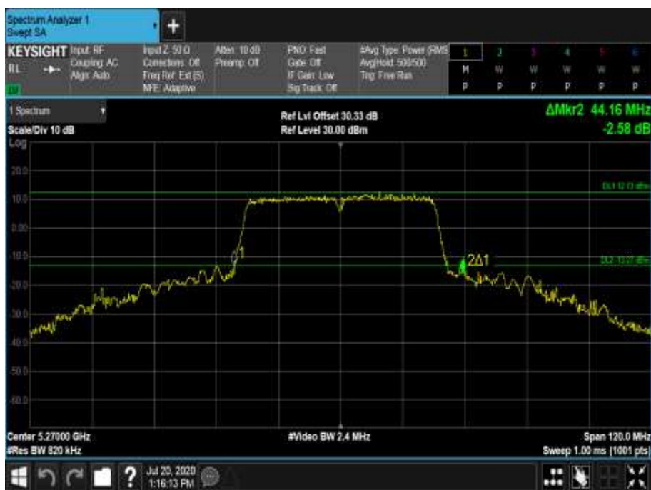
Figure 540 - 5270 MHz - 26 dB Emission Bandwidth
