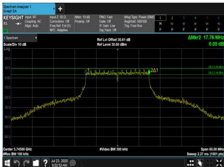
Figure 743 - 5745 MHz - 6 dB DTS Bandwidth
