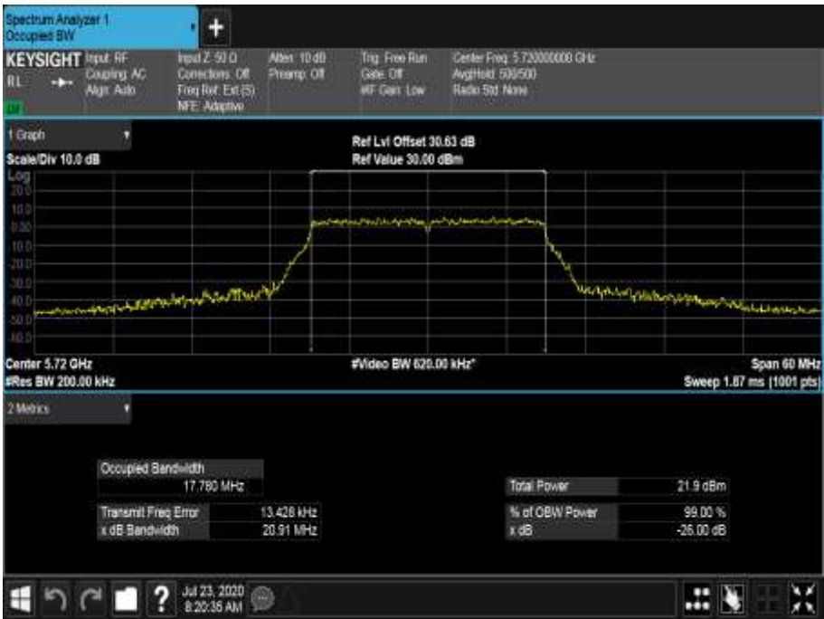
Figure 599 - 5720 MHz - 99% Occupied Bandwidth
