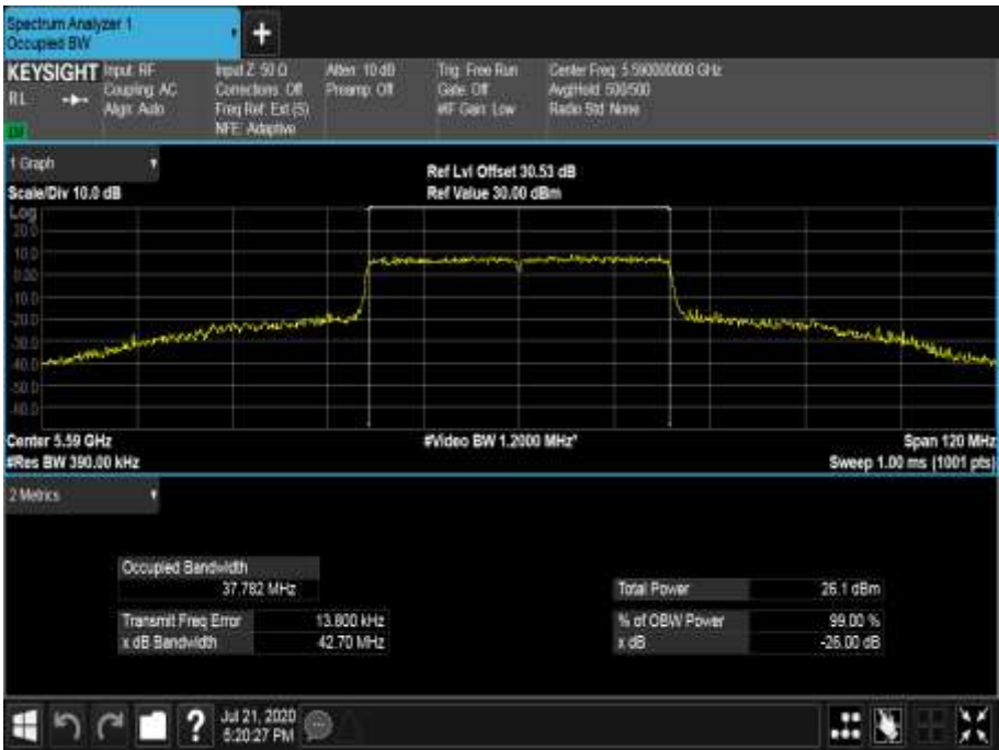
Figure 675 - 5590 MHz - 99% Occupied Bandwidth
