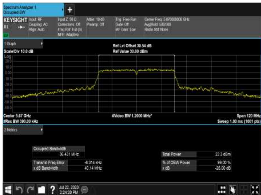
Figure 637 - 5670 MHz - 99% Occupied Bandwidth
