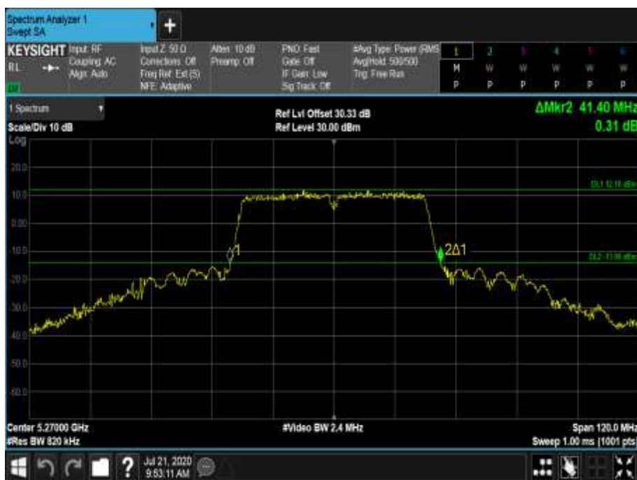
Figure 548 - 5270 MHz - 26 dB Emission Bandwidth
