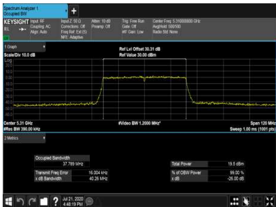
Figure 563 - 5310 MHz - 99% Occupied Bandwidth
