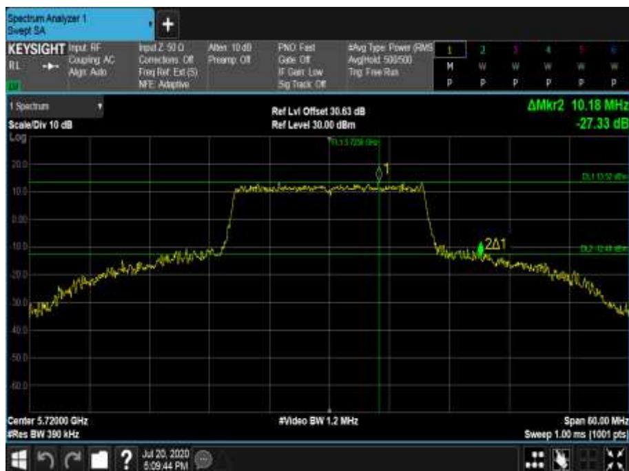
Figure 753 - 5720 MHz - 26 dB Emission Bandwidth
