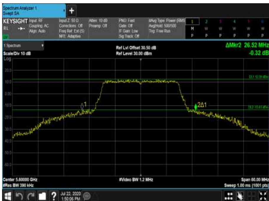
Figure 586 - 5600 MHz - 26 dB Emission Bandwidth
