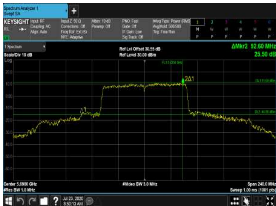
Figure 696 - 5690 MHz - 26 dB Emission Bandwidth
