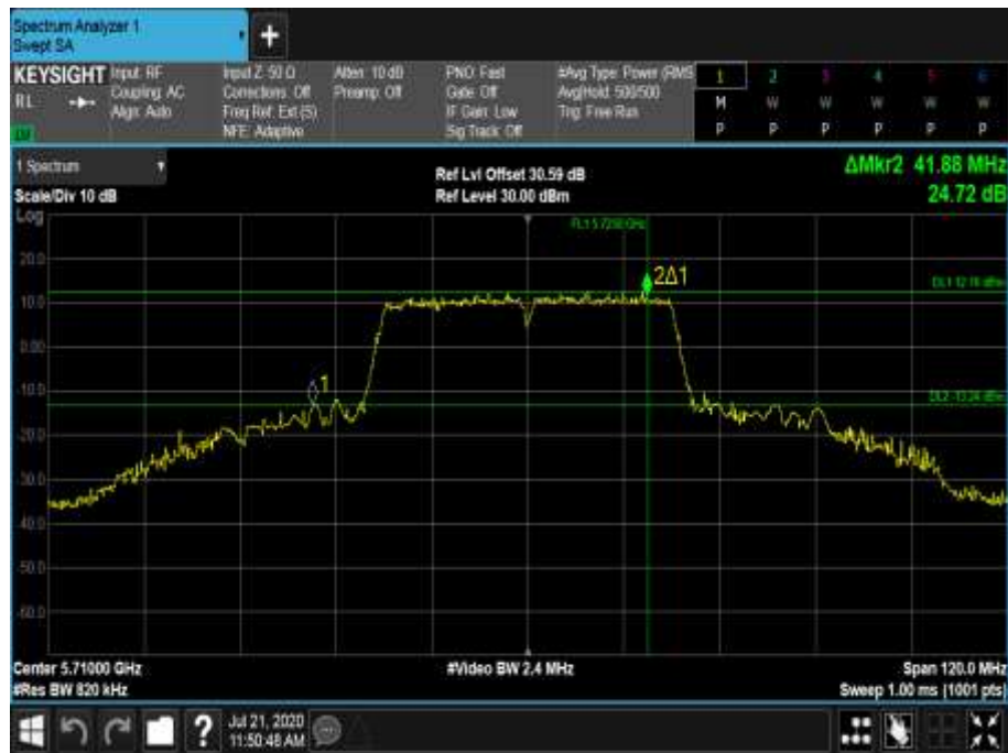
Figure 646 - 5710 MHz - 26 dB Emission Bandwidth
