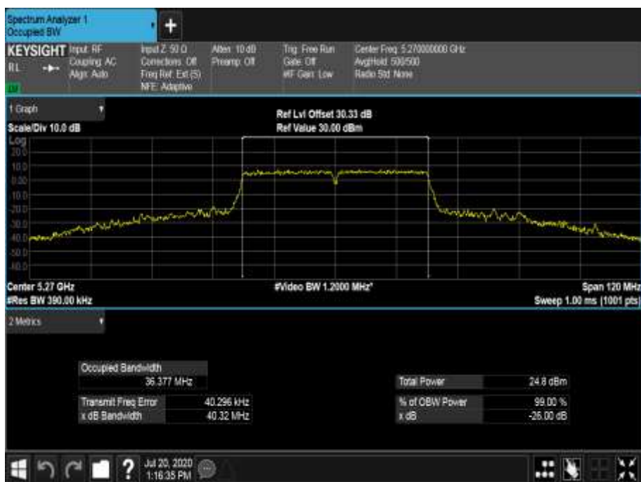
Figure 541 - 5270 MHz - 99% Occupied Bandwidth
