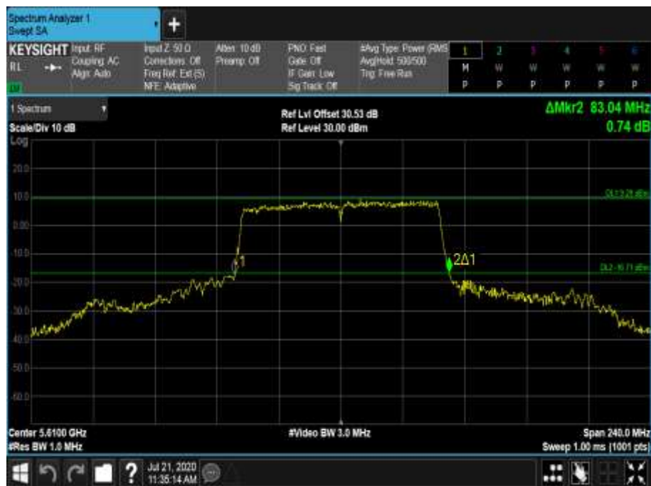
Figure 688 - 5610 MHz - 26 dB Emission Bandwidth
