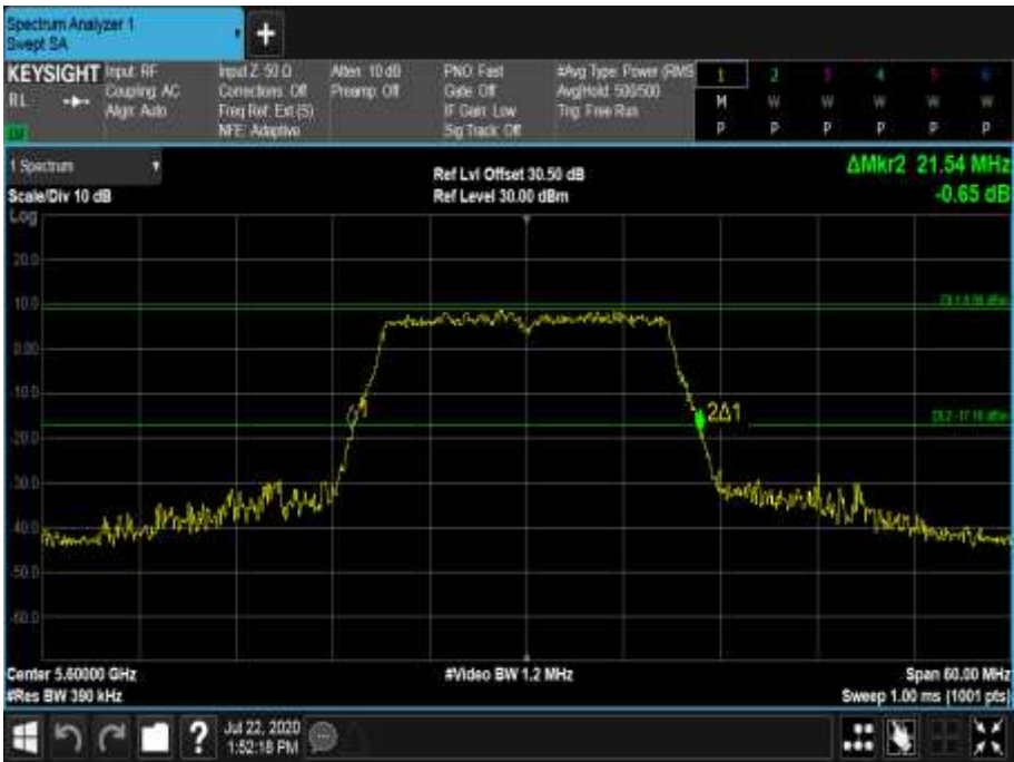
Figure 594 - 5600 MHz - 26 dB Emission Bandwidth
