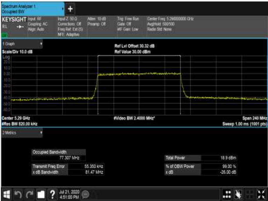
Figure 573 - 5290 MHz - 99% Occupied Bandwidth
