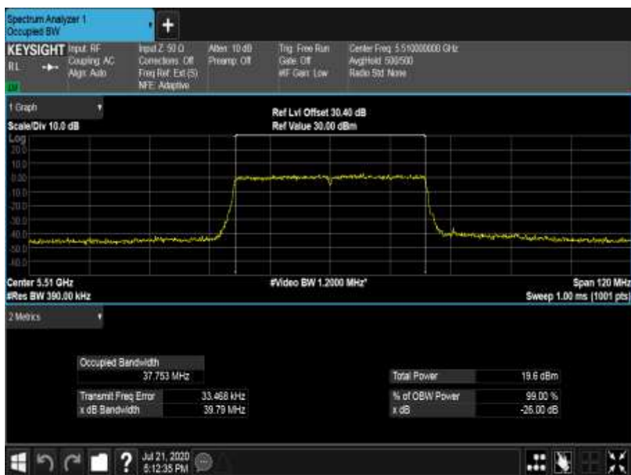
Figure 665 - 5510 MHz - 99% Occupied Bandwidth
