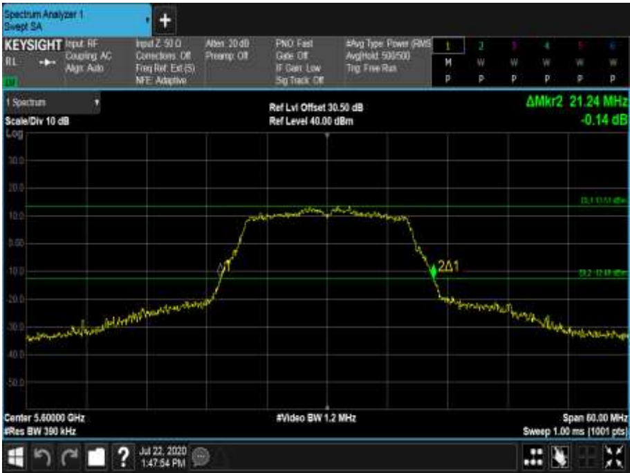
Figure 578 - 5600 MHz - 26 dB Emission Bandwidth
