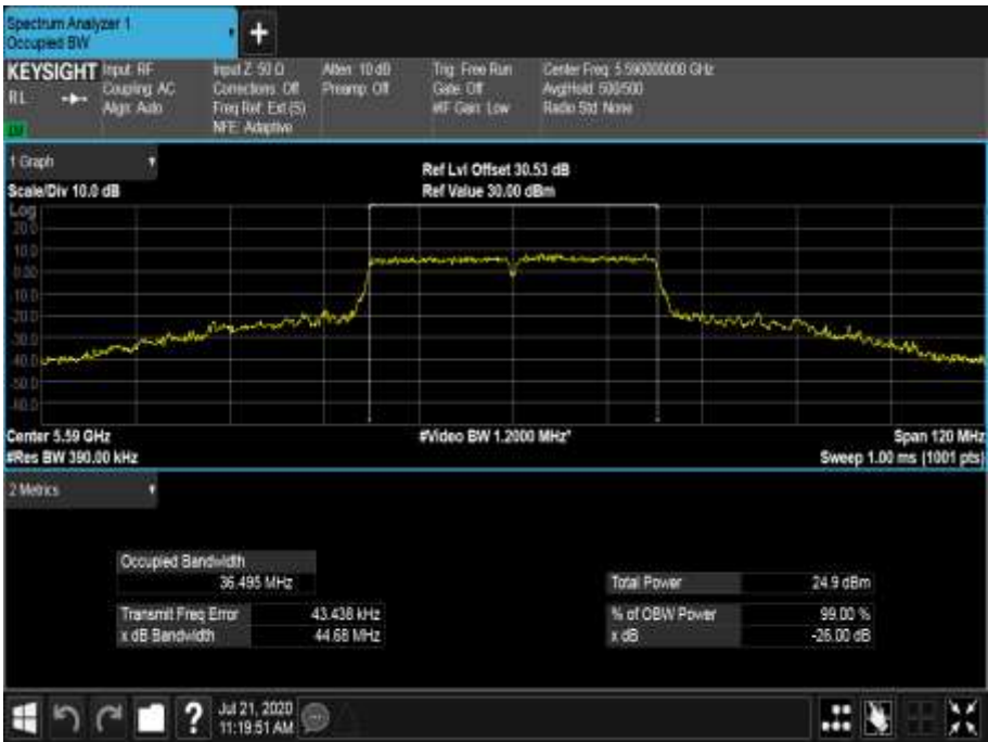
Figure 643 - 5590 MHz - 99% Occupied Bandwidth
