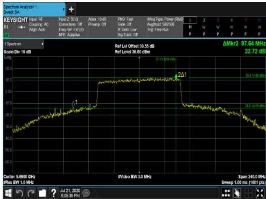
Figure 714 - 5690 MHz - 26 dB Emission Bandwidth
