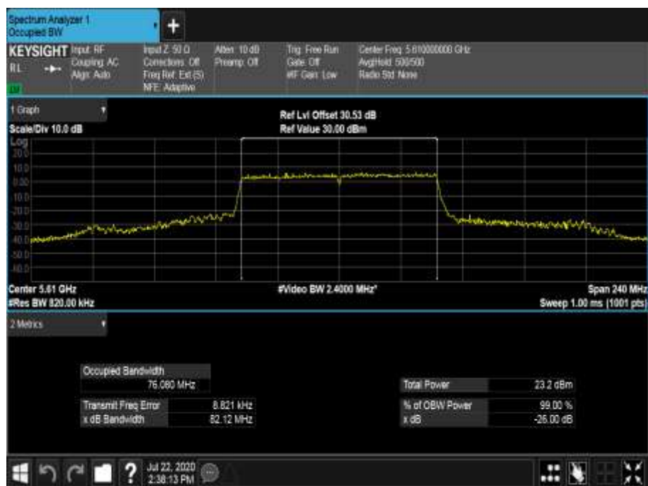
Figure 683 - 5610 MHz - 99% Occupied Bandwidth
