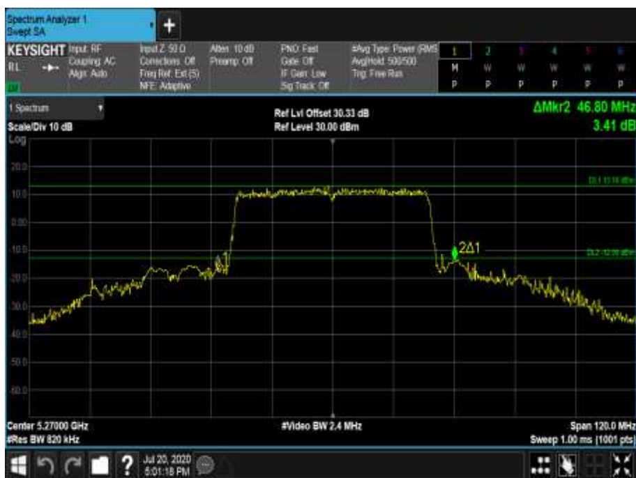
Figure 552 - 5270 MHz - 26 dB Emission Bandwidth
