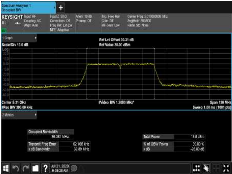
Figure 551 - 5310 MHz - 99% Occupied Bandwidth
