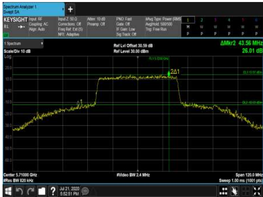
Figure 678 - 5710 MHz - 26 dB Emission Bandwidth
