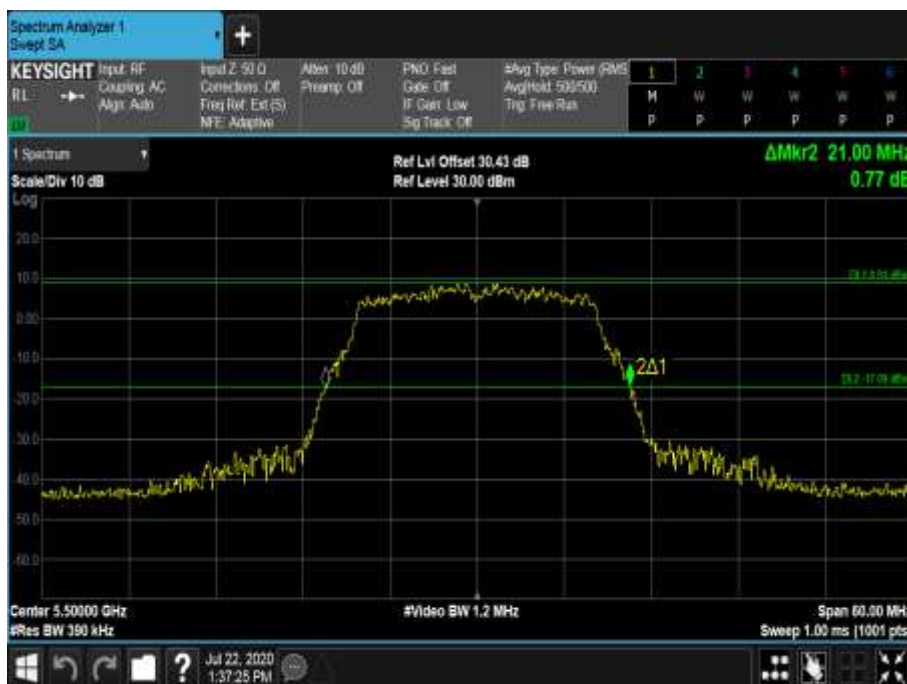
Figure 576 - 5500 MHz - 26 dB Emission Bandwidth
