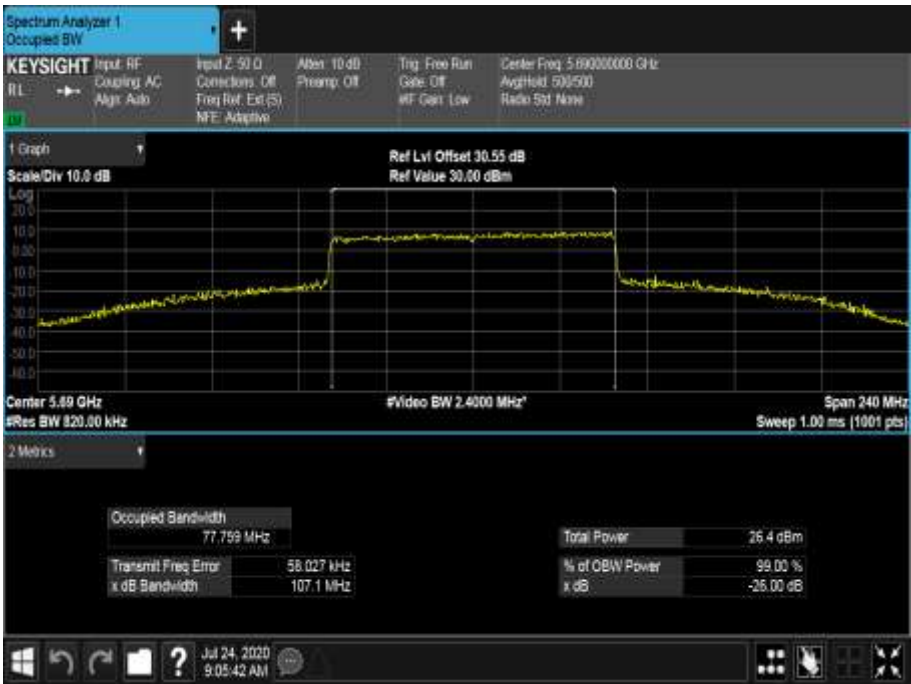
Figure 703 - 5690 MHz - 99% Occupied Bandwidth
