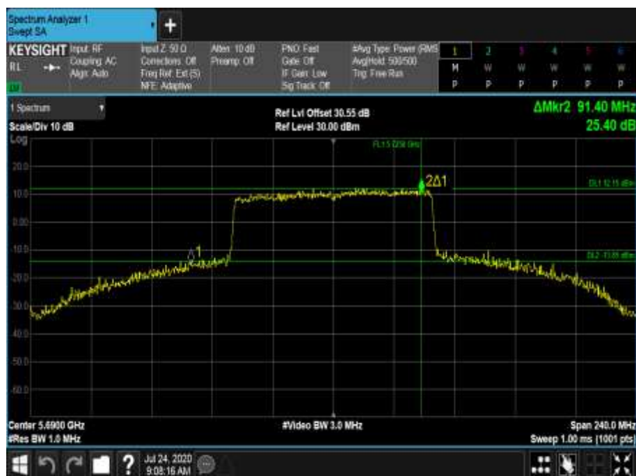
Figure 708 - 5690 MHz - 26 dB Emission Bandwidth
