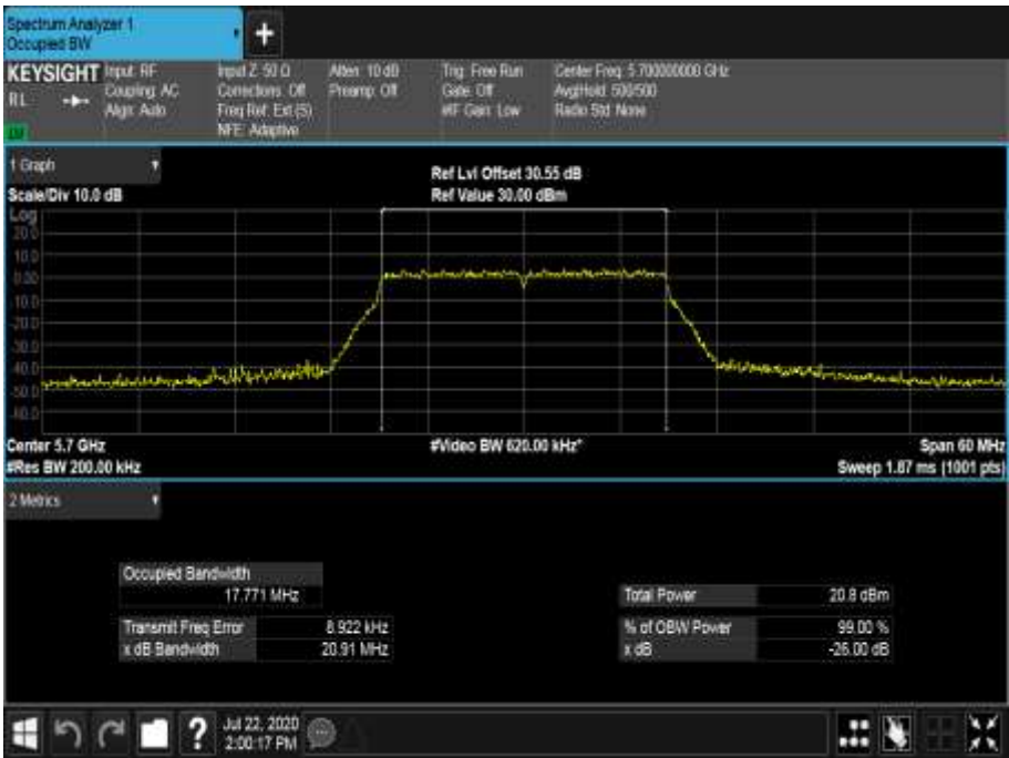
Figure 589 - 5700 MHz - 99% Occupied Bandwidth
