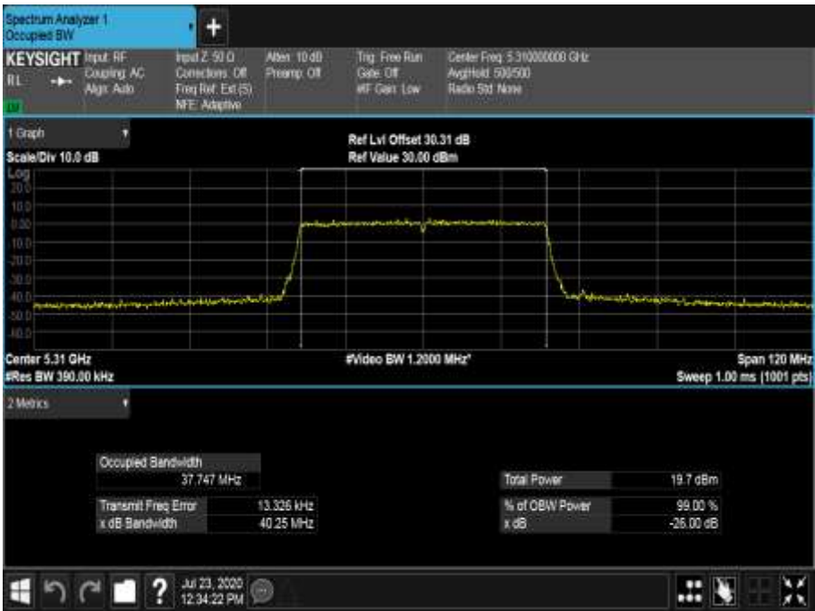
Figure 559 - 5310 MHz - 99% Occupied Bandwidth
