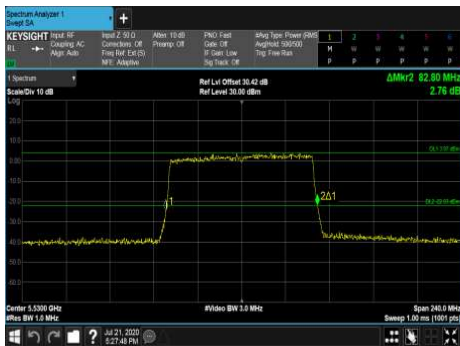
Figure 704 - 5530 MHz - 26 dB Emission Bandwidth
