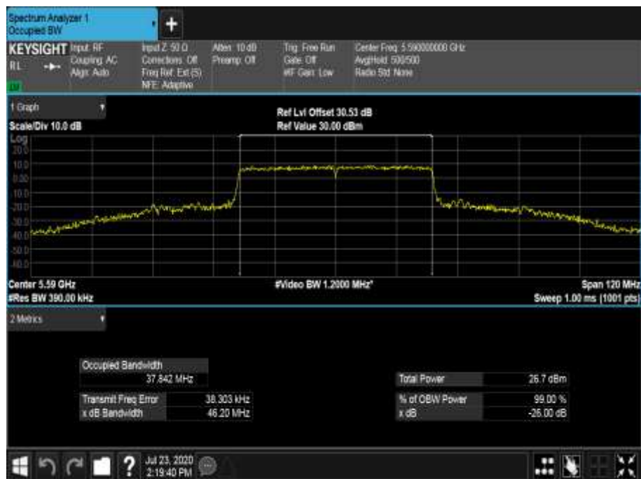
Figure 659 - 5590 MHz - 99% Occupied Bandwidth
