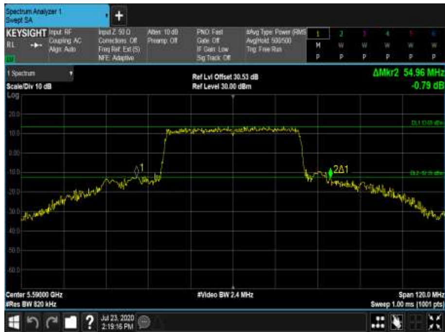
Figure 658 - 5590 MHz - 26 dB Emission Bandwidth
