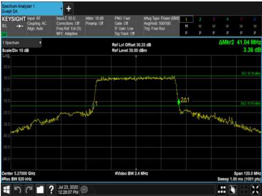
Figure 556 - 5270 MHz - 26 dB Emission Bandwidth
