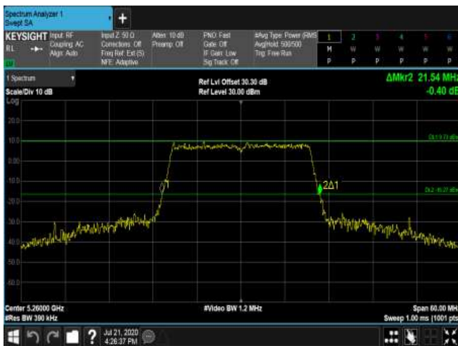
Figure 534 - 5260 MHz - 26 dB Emission Bandwidth
