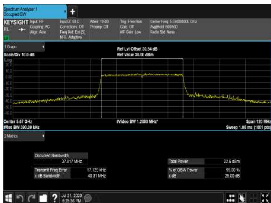
Figure 677 - 5670 MHz - 99% Occupied Bandwidth
