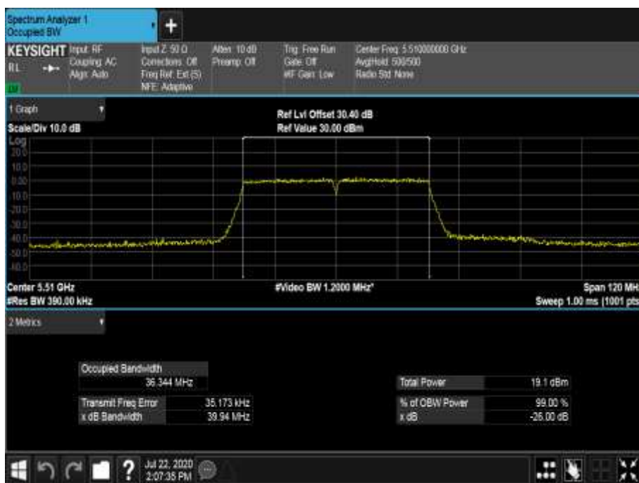
Figure 633 - 5510 MHz - 99% Occupied Bandwidth
