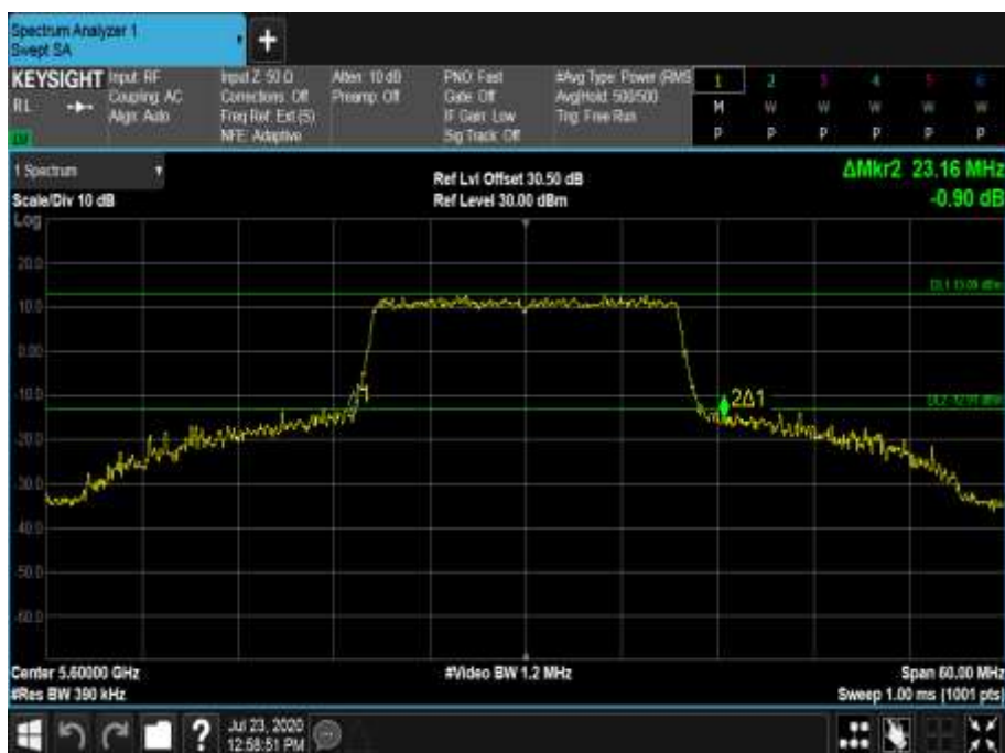
Figure 610 - 5600 MHz - 26 dB Emission Bandwidth
