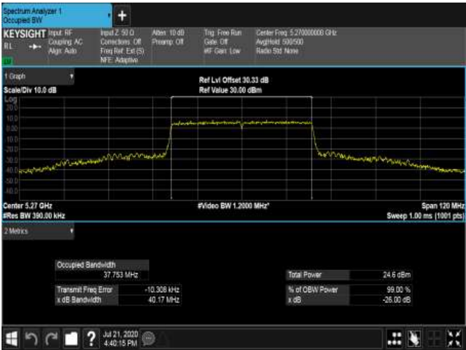
Figure 557 - 5270 MHz - 99% Occupied Bandwidth
