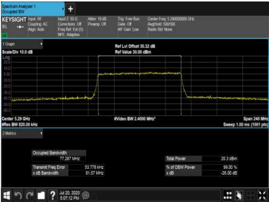
Figure 571 - 5290 MHz - 99% Occupied Bandwidth
