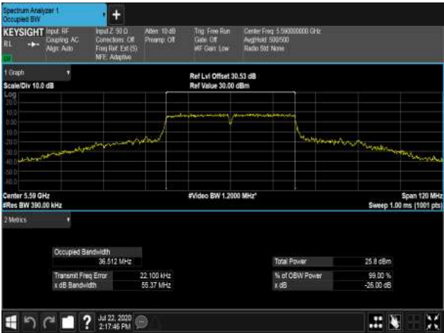
Figure 635 - 5590 MHz - 99% Occupied Bandwidth
