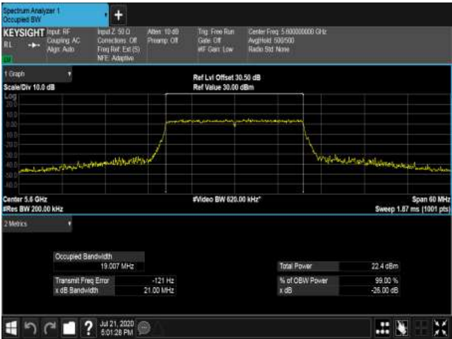
Figure 619 - 5600 MHz - 99% Occupied Bandwidth
