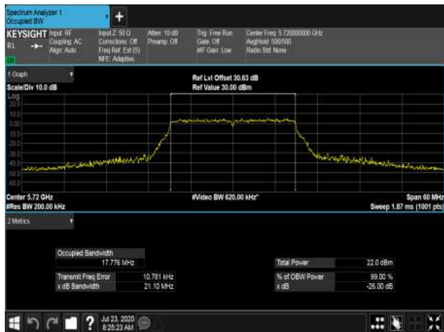
Figure 730 - 5720 MHz - 99% Occupied Bandwidth
