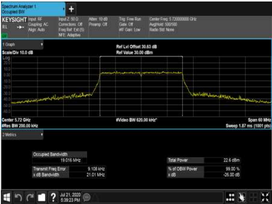
Figure 623 - 5720 MHz - 99% Occupied Bandwidth
