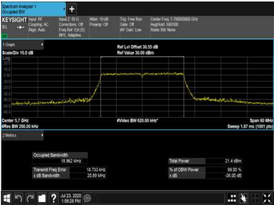
Figure 613 - 5700 MHz - 99% Occupied Bandwidth
