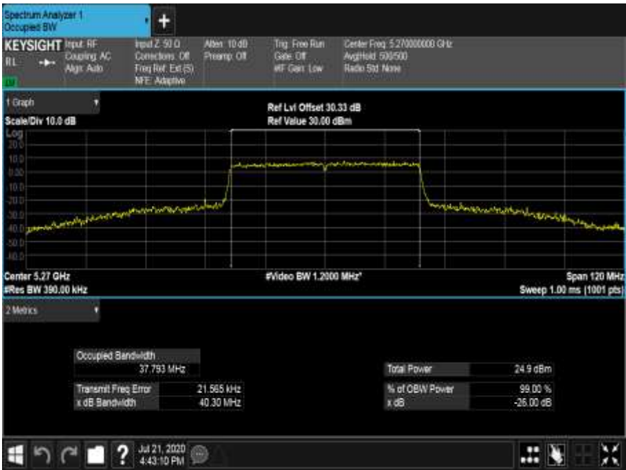
Figure 561 - 5270 MHz - 99% Occupied Bandwidth
