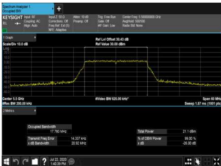
Figure 585 - 5500 MHz - 99% Occupied Bandwidth
