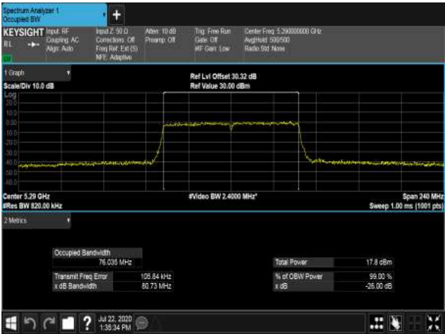
Figure 569 - 5290 MHz - 99% Occupied Bandwidth
