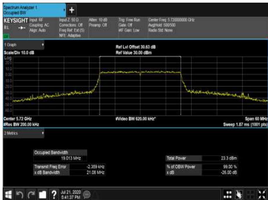
Figure 631 - 5720 MHz - 99% Occupied Bandwidth
