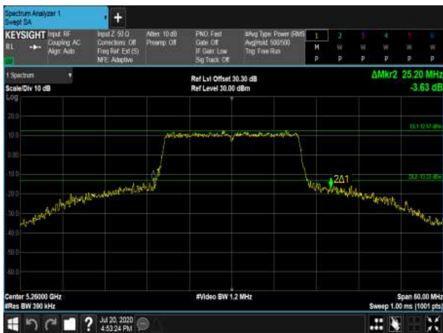
Figure 522 - 5260 MHz - 26 dB Emission Bandwidth
