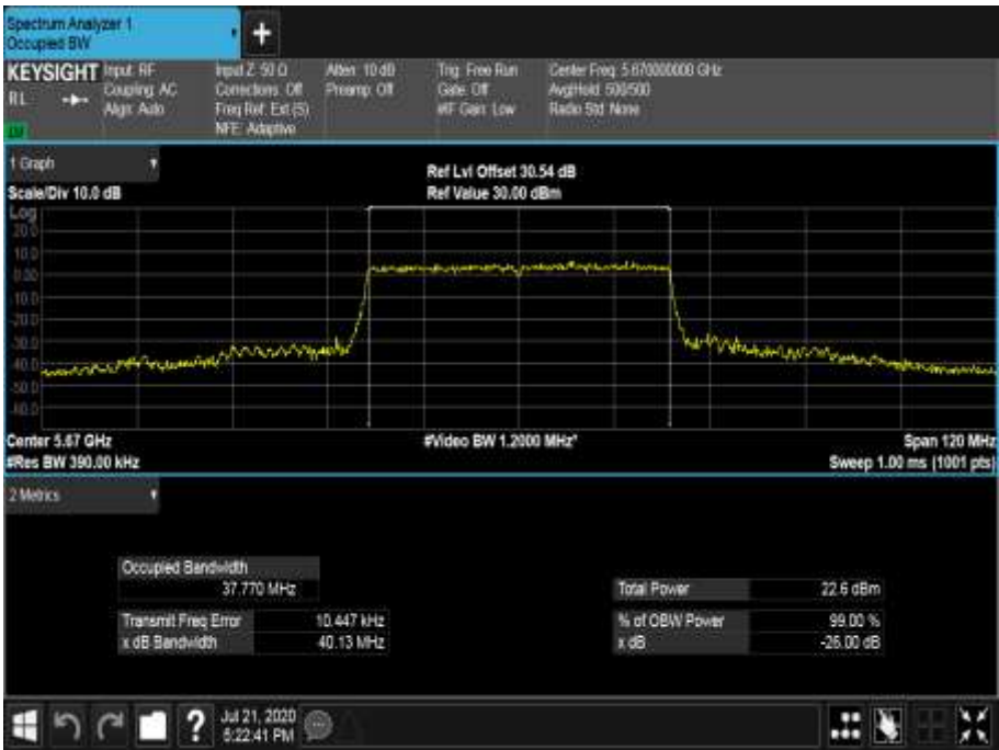
Figure 669 - 5670 MHz - 99% Occupied Bandwidth
