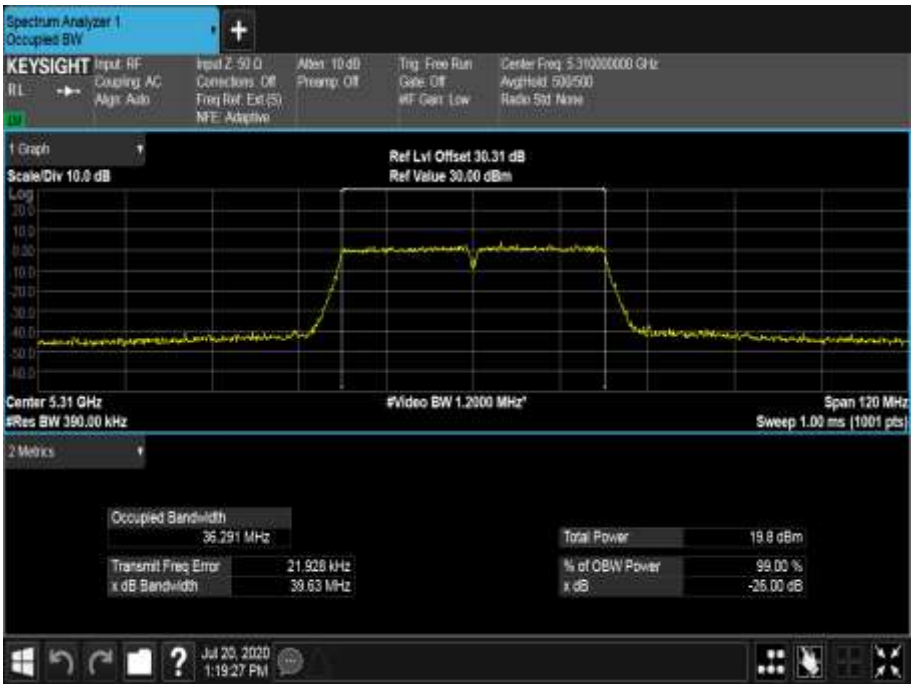
Figure 543 - 5310 MHz - 99% Occupied Bandwidth
