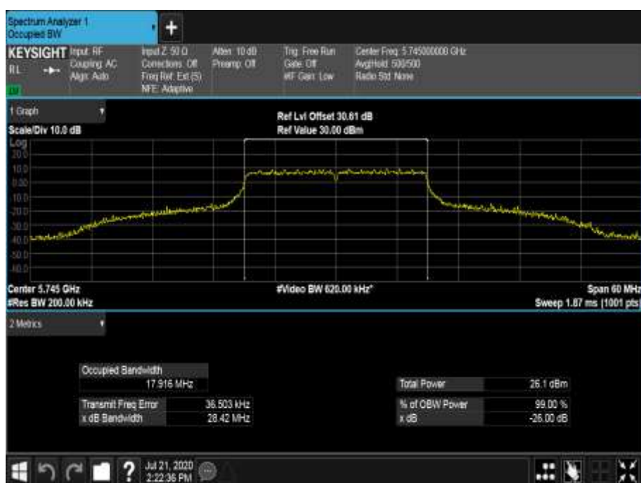
Figure 733 - 5745 MHz - 99% Occupied Bandwidth
