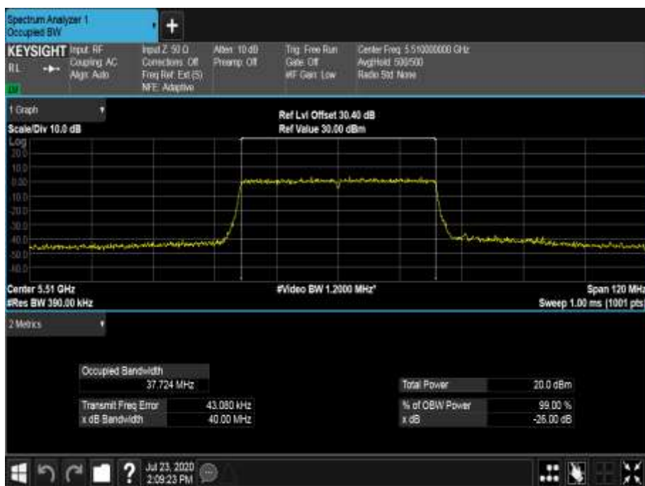
Figure 657 - 5510 MHz - 99% Occupied Bandwidth
