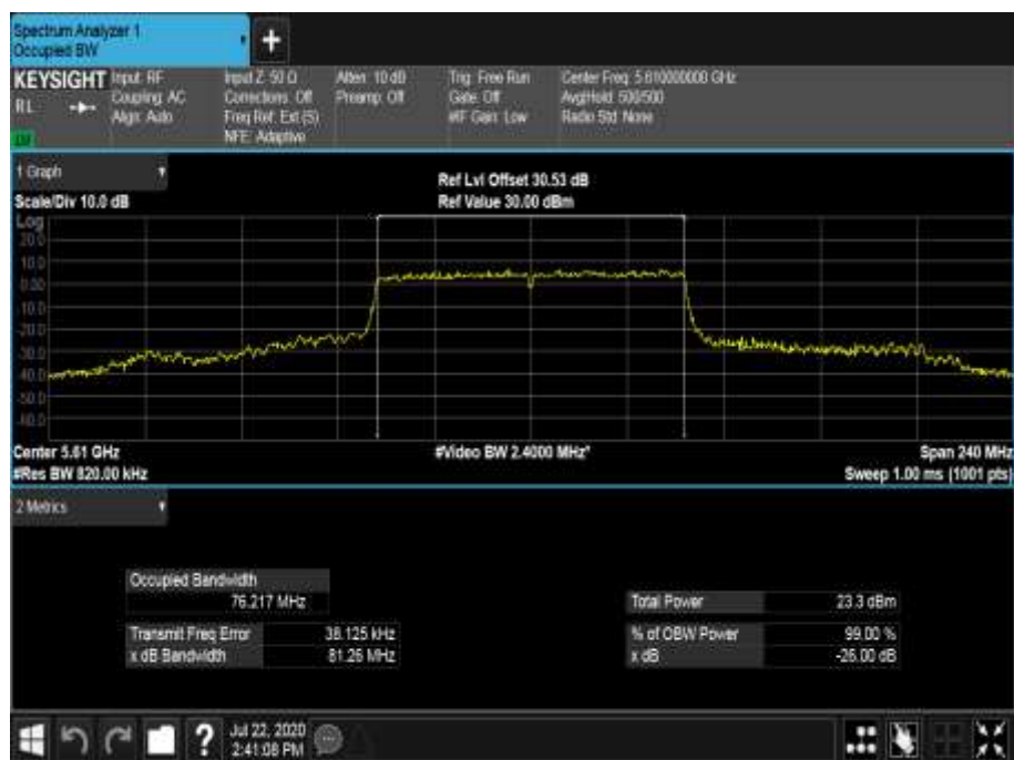
Figure 689 - 5610 MHz - 99% Occupied Bandwidth
