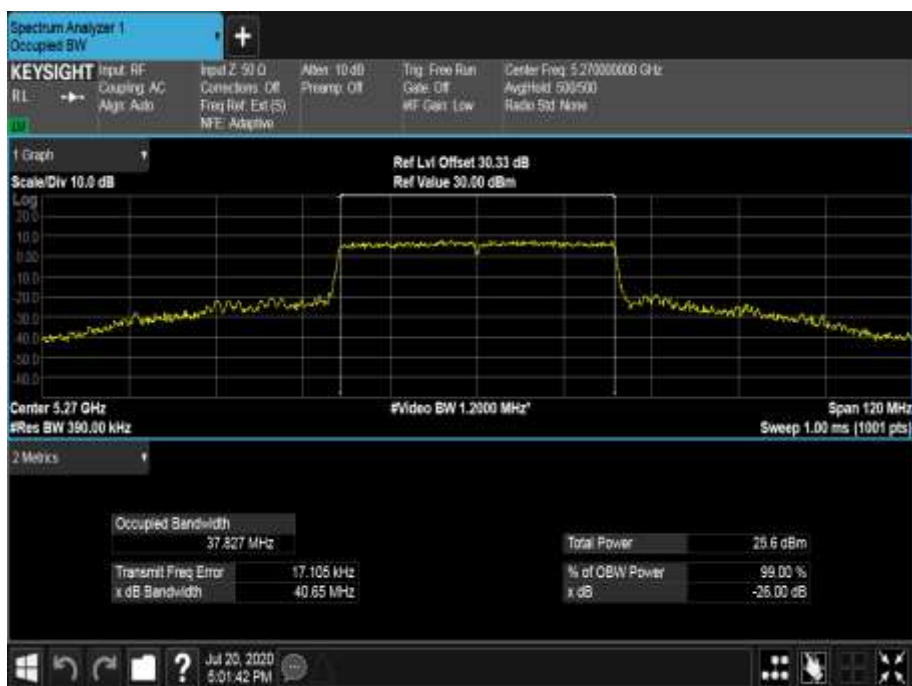
Figure 553 - 5270 MHz - 99% Occupied Bandwidth
