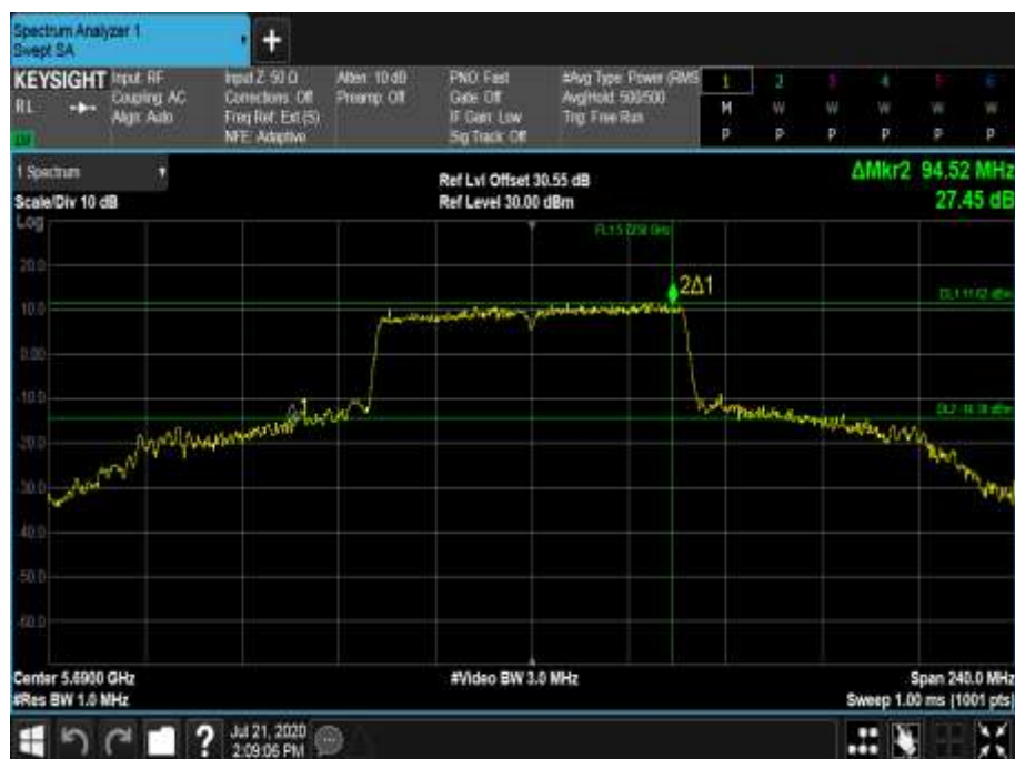
Figure 690 - 5690 MHz - 26 dB Emission Bandwidth
