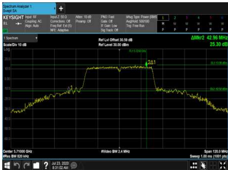
Figure 638 - 5710 MHz - 26 dB Emission Bandwidth
