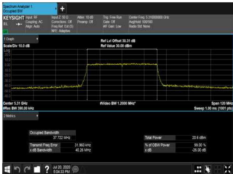
Figure 555 - 5310 MHz - 99% Occupied Bandwidth
