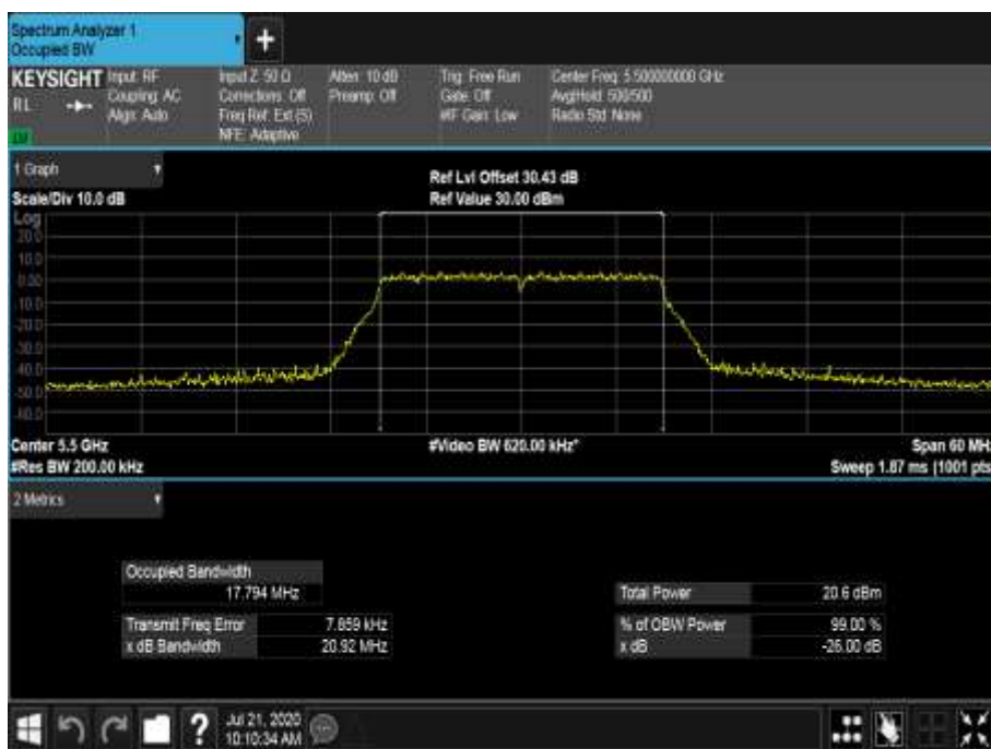
Figure 601 - 5500 MHz - 99% Occupied Bandwidth
