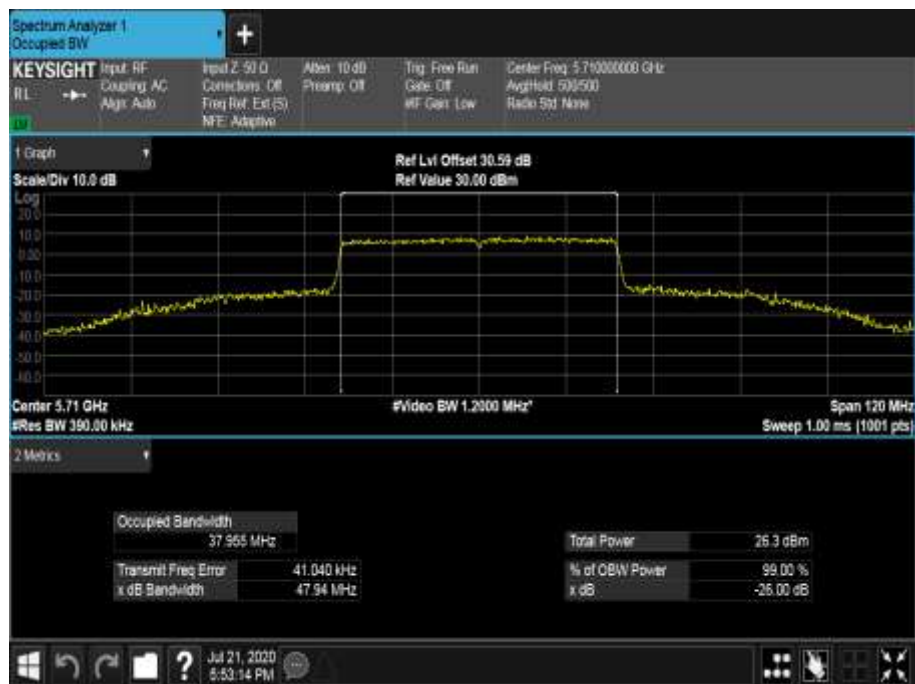
Figure 679 - 5710 MHz - 99% Occupied Bandwidth
