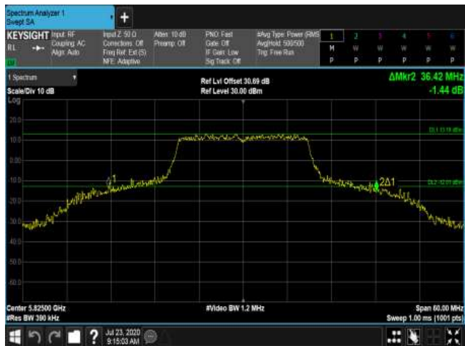
Figure 738 - 5825 MHz - 26 dB Emission Bandwidth
