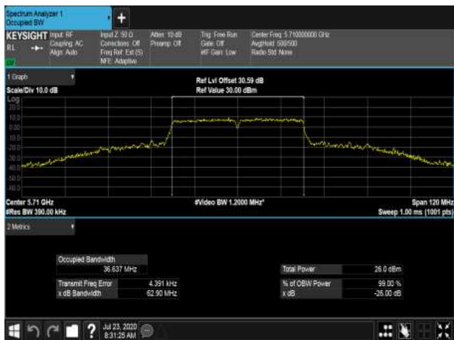
Figure 639 - 5710 MHz - 99% Occupied Bandwidth
