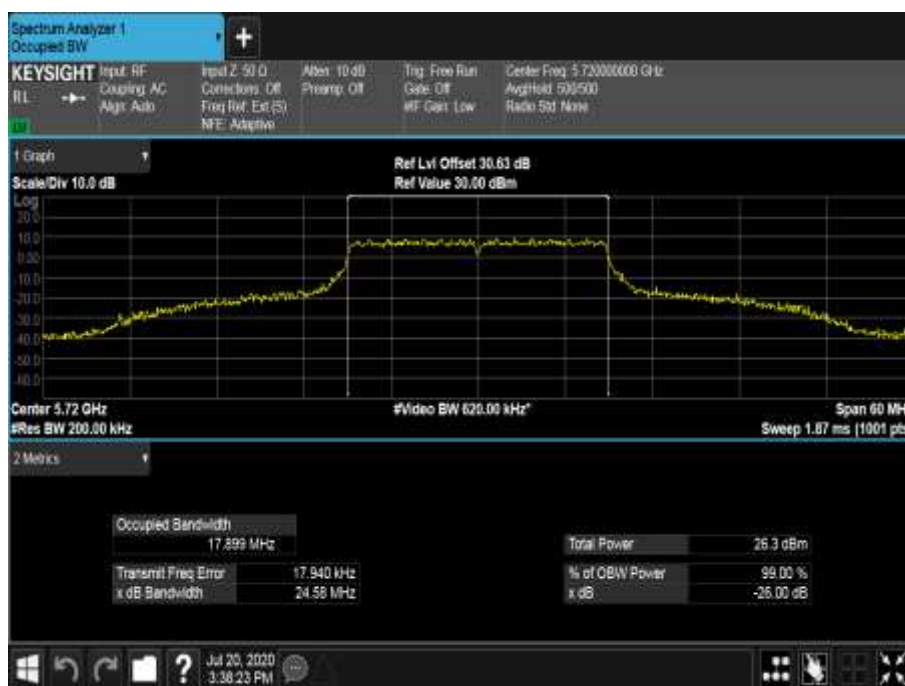
Figure 718 - 5720 MHz - 99% Occupied Bandwidth
