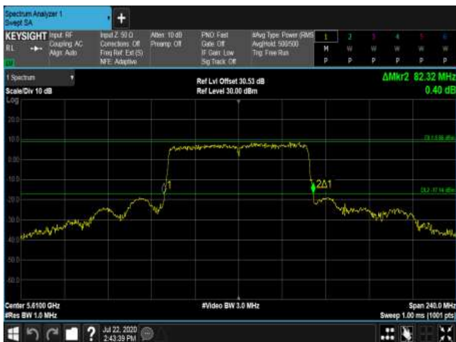
Figure 694 - 5610 MHz - 26 dB Emission Bandwidth
