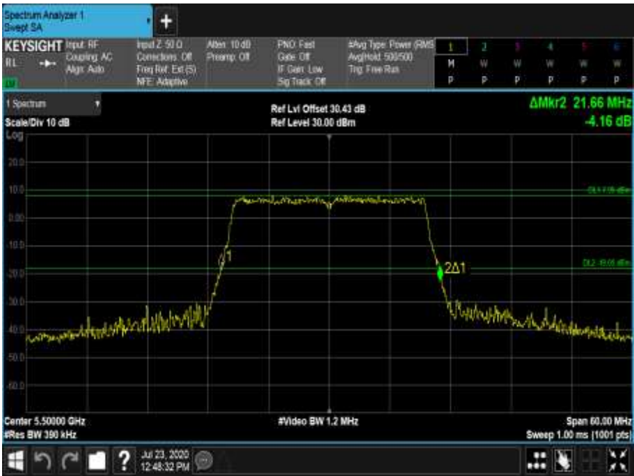
Figure 608 - 5500 MHz - 26 dB Emission Bandwidth
