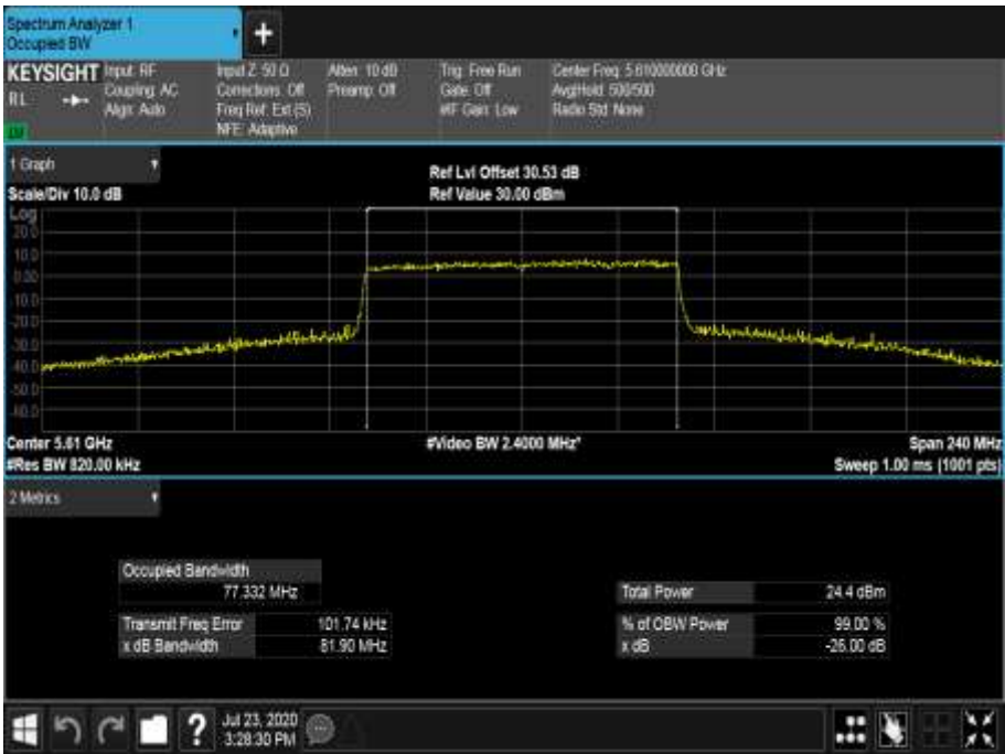
Figure 701 - 5610 MHz - 99% Occupied Bandwidth
