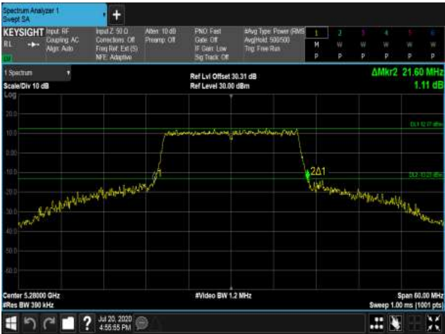
Figure 524 - 5280 MHz - 26 dB Emission Bandwidth
