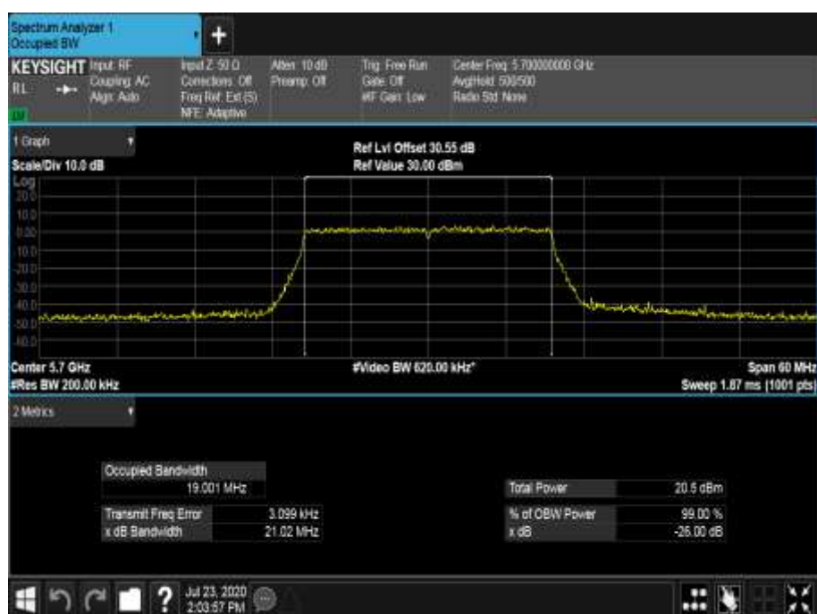
Figure 629 - 5700 MHz - 99% Occupied Bandwidth
