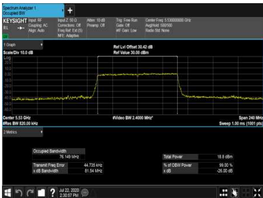
Figure 681 - 5530 MHz - 99% Occupied Bandwidth
