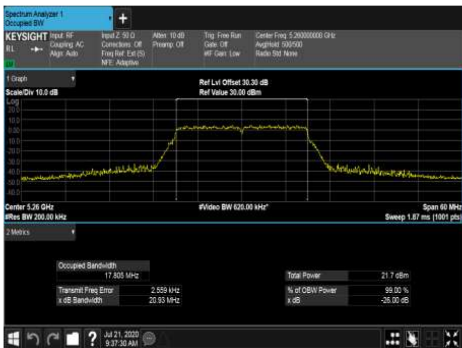
Figure 517 - 5260 MHz - 99% Occupied Bandwidth
