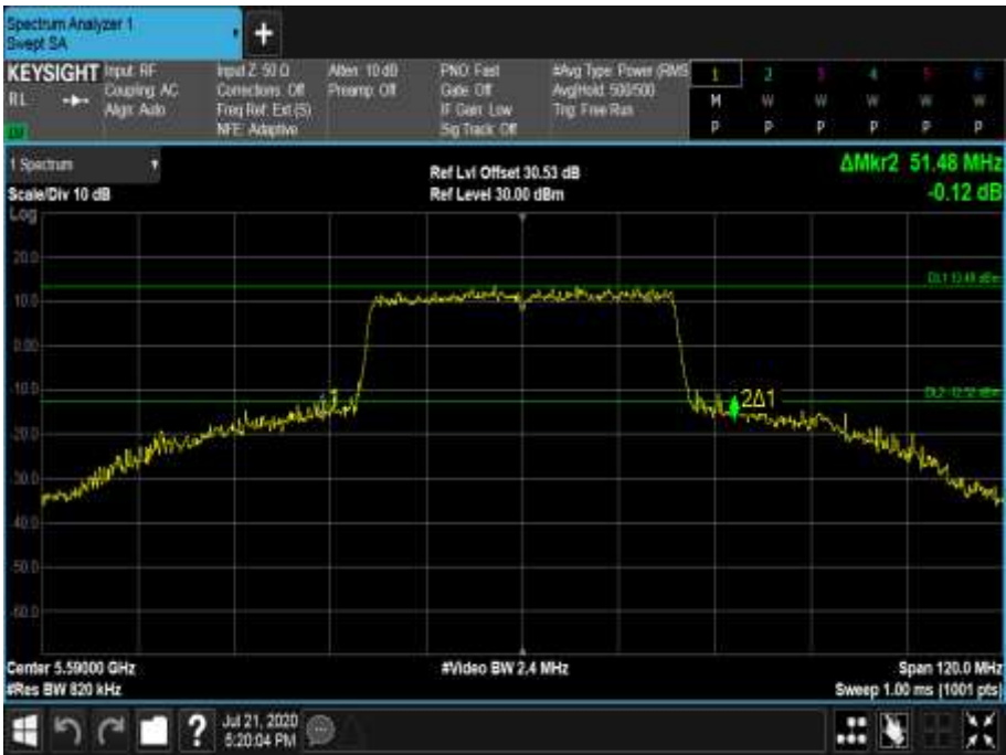
Figure 674 - 5590 MHz - 26 dB Emission Bandwidth
