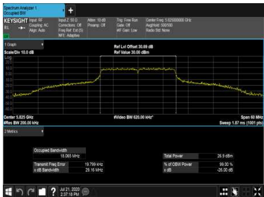
Figure 739 - 5825 MHz - 99% Occupied Bandwidth
