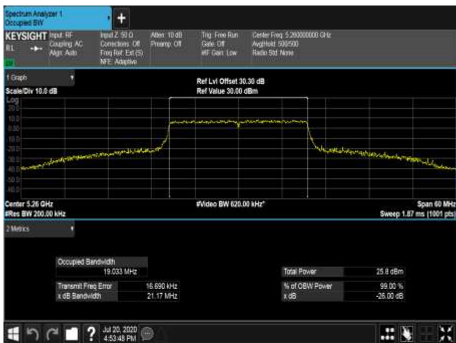
Figure 523 - 5260 MHz - 99% Occupied Bandwidth
