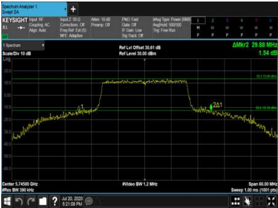
Figure 756 - 5745 MHz - 26 dB Emission Bandwidth
