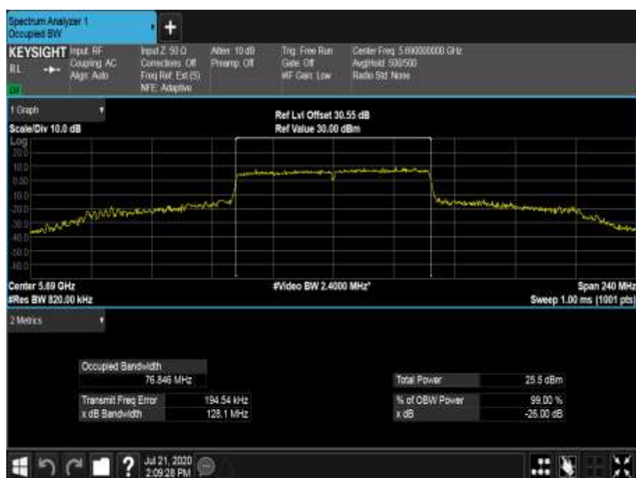
Figure 691 - 5690 MHz - 99% Occupied Bandwidth
