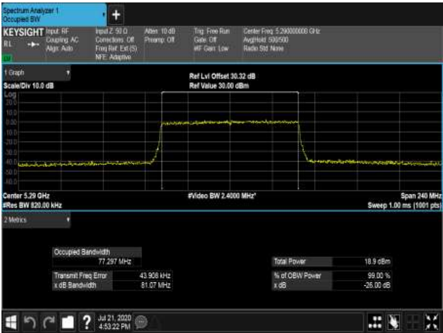
Figure 575 - 5290 MHz - 99% Occupied Bandwidth
