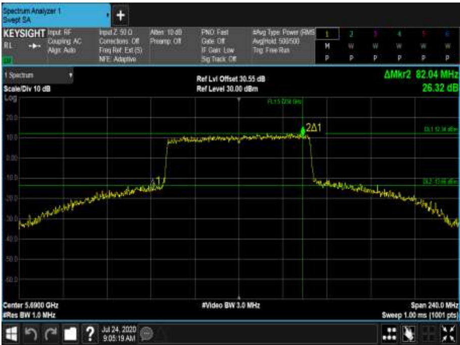
Figure 702 - 5690 MHz - 26 dB Emission Bandwidth
