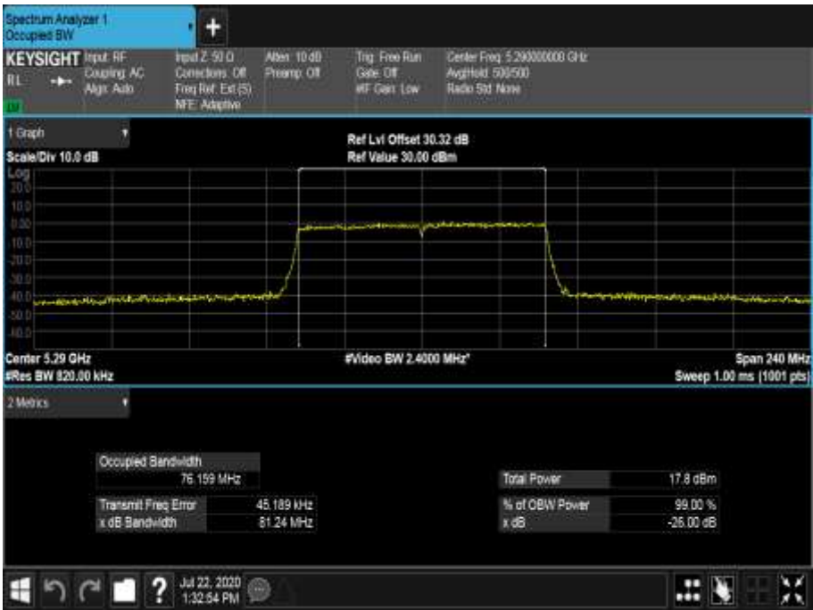
Figure 567 - 5290 MHz - 99% Occupied Bandwidth
