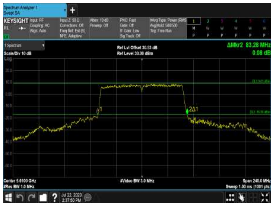
Figure 682 - 5610 MHz - 26 dB Emission Bandwidth
