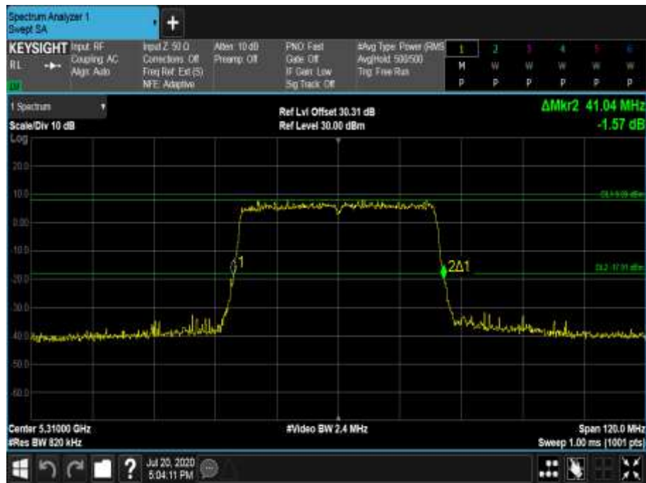
Figure 554 - 5310 MHz - 26 dB Emission Bandwidth
