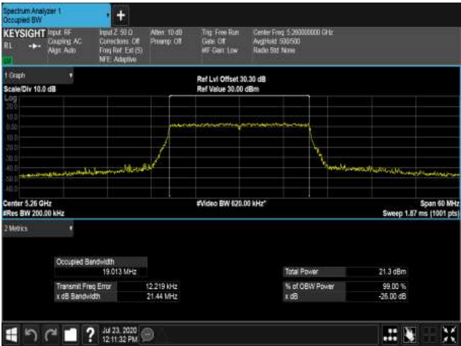
Figure 529 - 5260 MHz - 99% Occupied Bandwidth
