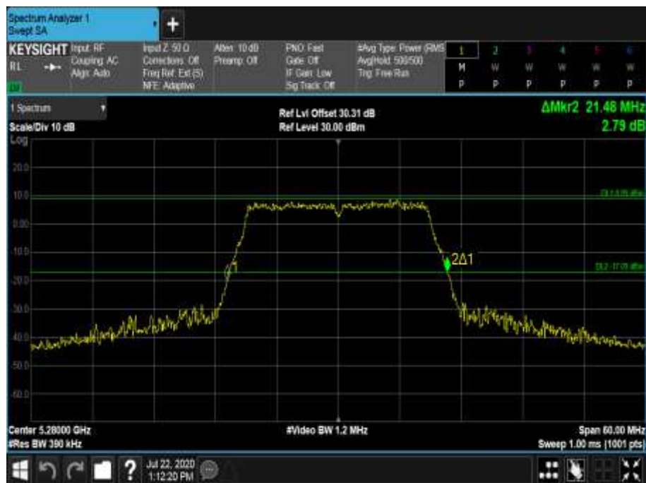
Figure 518 - 5280 MHz - 26 dB Emission Bandwidth
