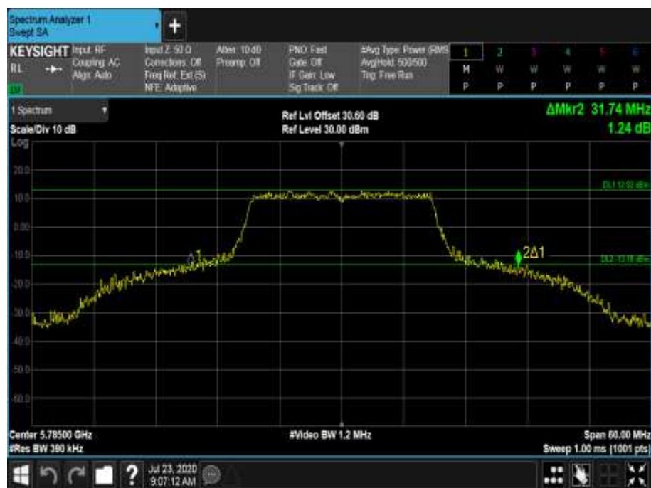
Figure 735 - 5785 MHz - 26 dB Emission Bandwidth
