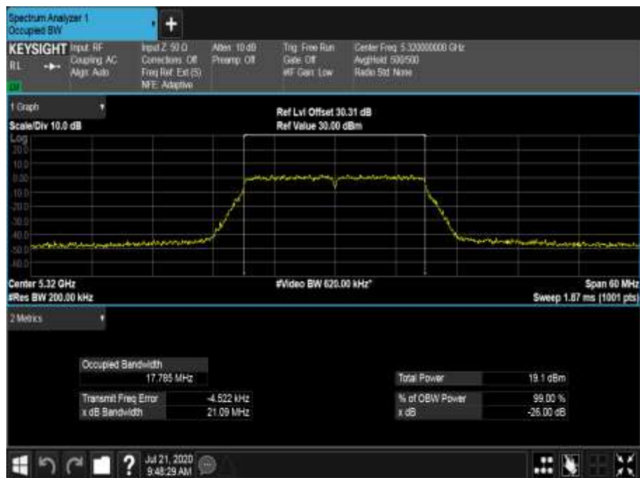
Figure 521 - 5320 MHz - 99% Occupied Bandwidth
