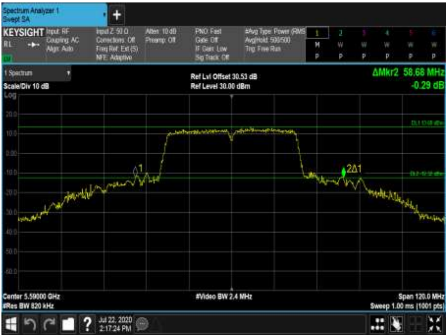
Figure 634 - 5590 MHz - 26 dB Emission Bandwidth
