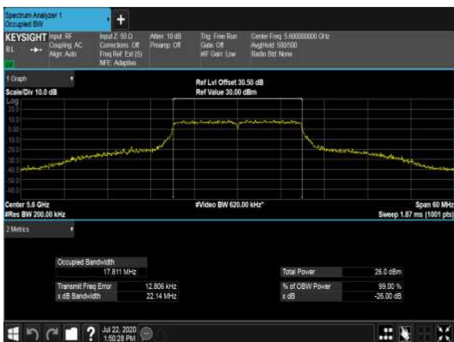
Figure 587 - 5600 MHz - 99% Occupied Bandwidth
