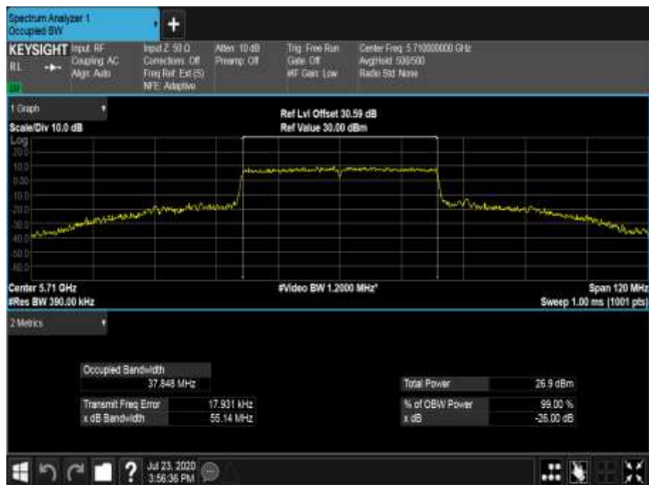
Figure 663 - 5710 MHz - 99% Occupied Bandwidth
