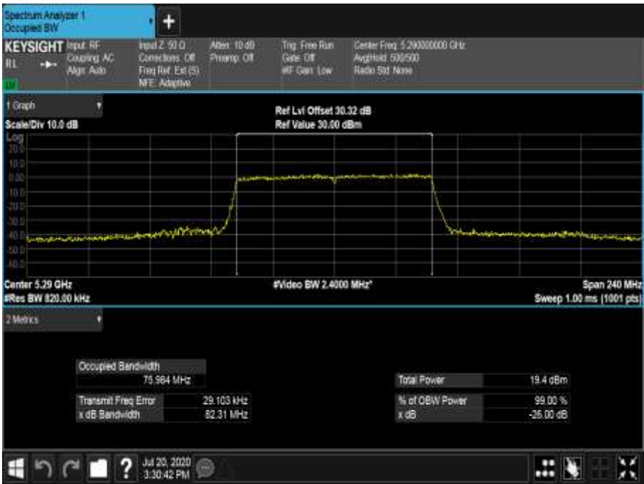
Figure 565 - 5290 MHz - 99% Occupied Bandwidth
