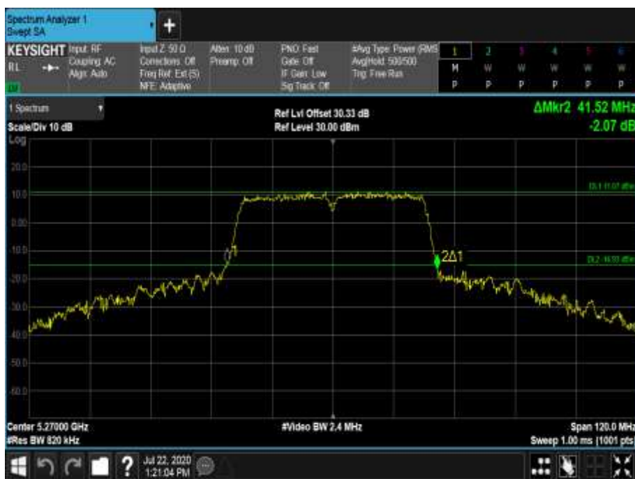
Figure 544 - 5270 MHz - 26 dB Emission Bandwidth
