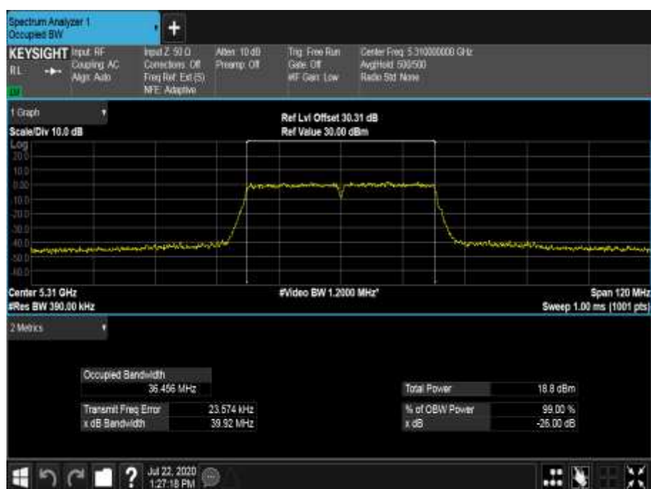
Figure 547 - 5310 MHz - 99% Occupied Bandwidth
