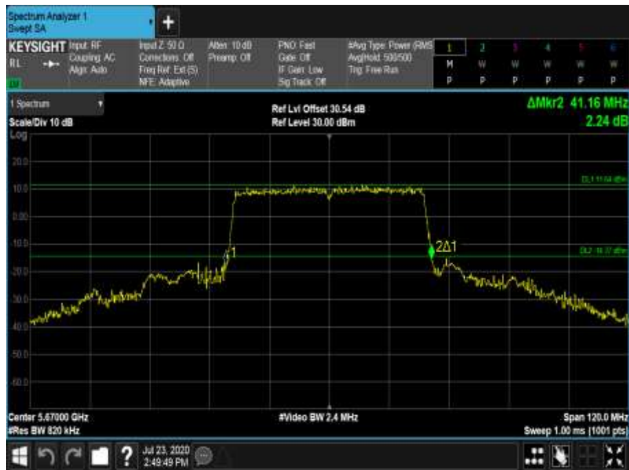
Figure 660 - 5670 MHz - 26 dB Emission Bandwidth
