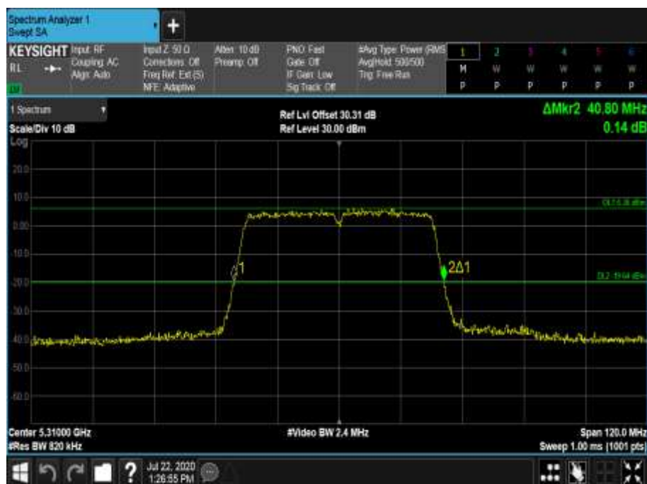
Figure 546 - 5310 MHz - 26 dB Emission Bandwidth
