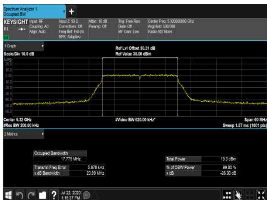
Figure 515 - 5320 MHz - 99% Occupied Bandwidth
