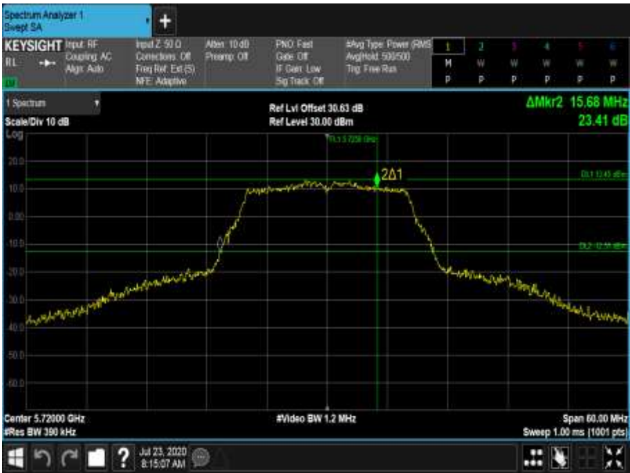
Figure 582 - 5720 MHz - 26 dB Emission Bandwidth
