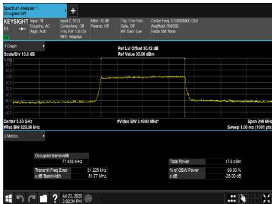
Figure 705 - 5530 MHz - 99% Occupied Bandwidth
