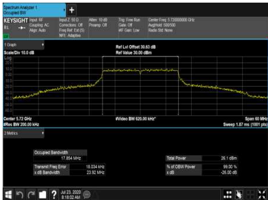
Figure 591 - 5720 MHz - 99% Occupied Bandwidth
