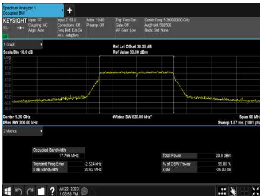
Figure 511 - 5260 MHz - 99% Occupied Bandwidth
