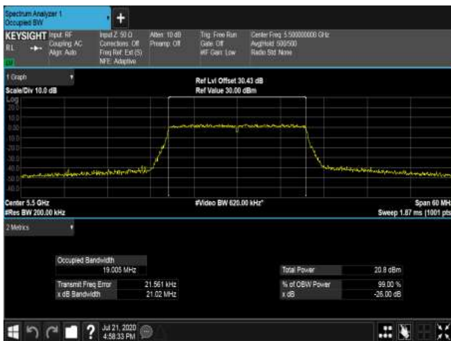
Figure 625 - 5500 MHz - 99% Occupied Bandwidth
