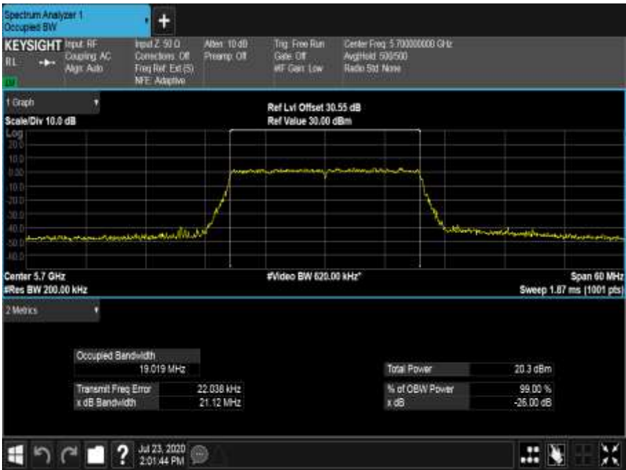
Figure 621 - 5700 MHz - 99% Occupied Bandwidth
