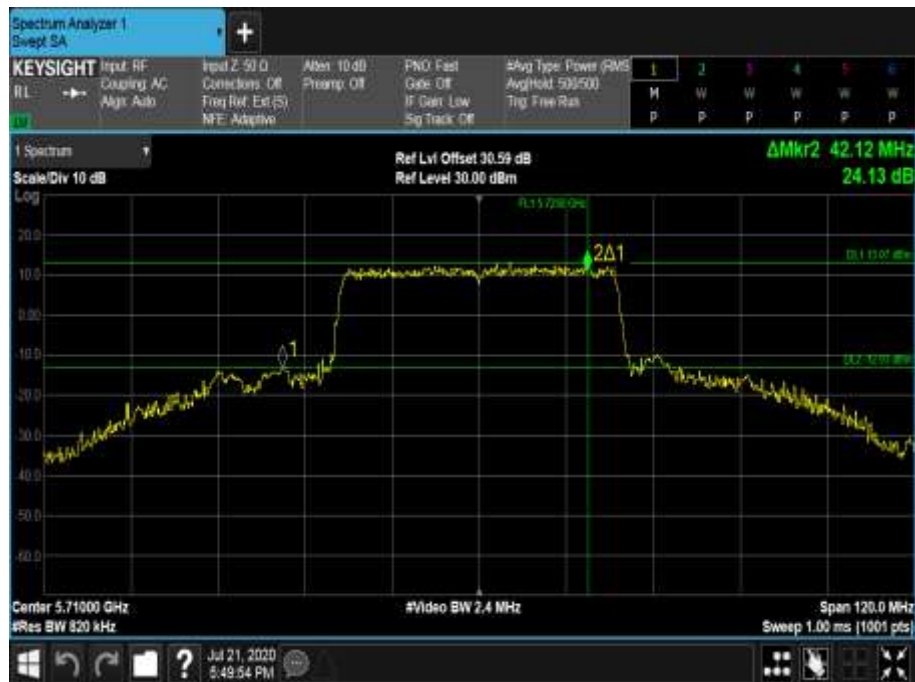
Figure 670 - 5710 MHz - 26 dB Emission Bandwidth
