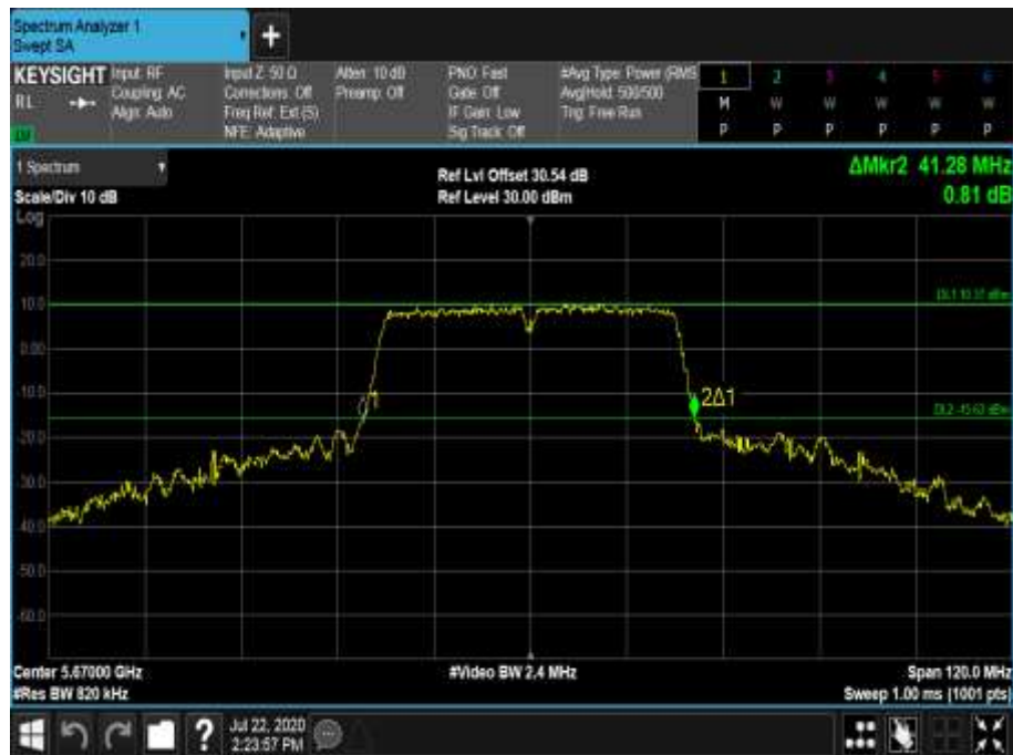
Figure 636 - 5670 MHz - 26 dB Emission Bandwidth
