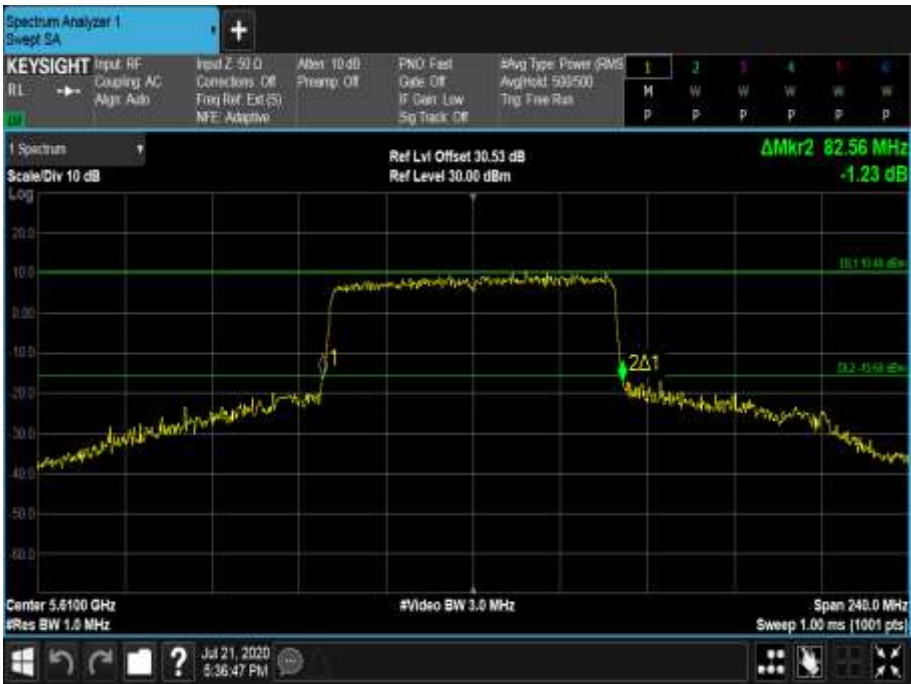
Figure 712 - 5610 MHz - 26 dB Emission Bandwidth
