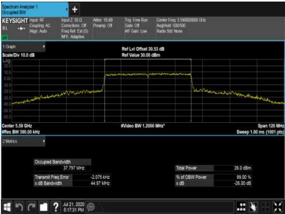
Figure 667 - 5590 MHz - 99% Occupied Bandwidth
