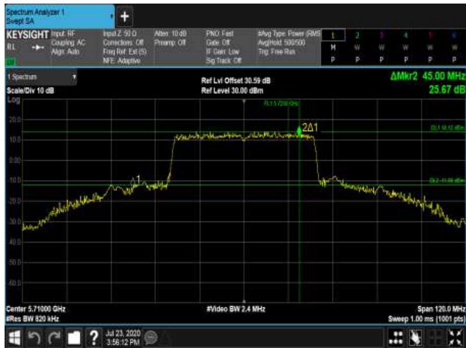
Figure 662 - 5710 MHz - 26 dB Emission Bandwidth
