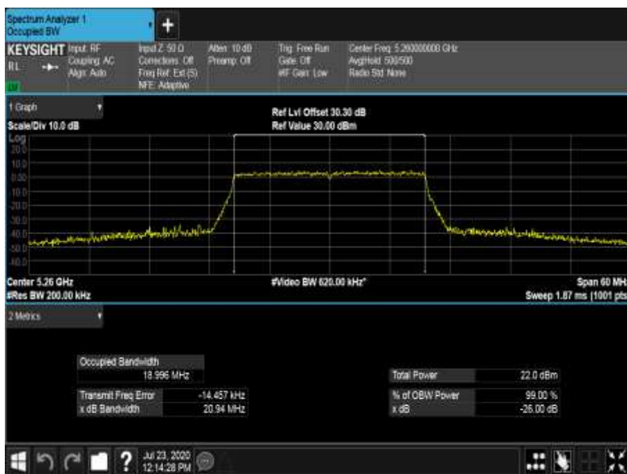
Figure 535 - 5260 MHz - 99% Occupied Bandwidth
