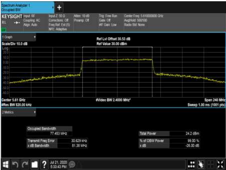
Figure 707 - 5610 MHz - 99% Occupied Bandwidth
