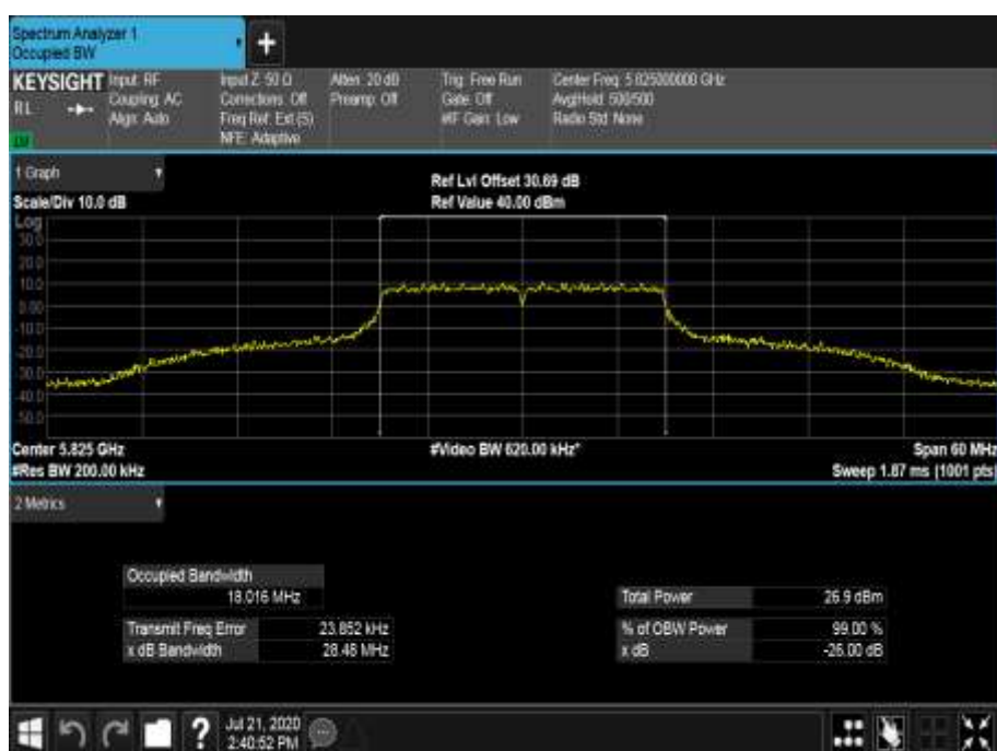
Figure 751 - 5825 MHz - 99% Occupied Bandwidth
