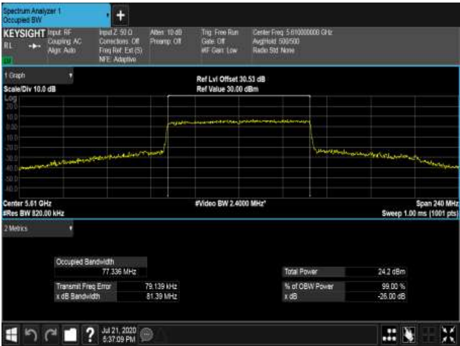
Figure 713 - 5610 MHz - 99% Occupied Bandwidth
