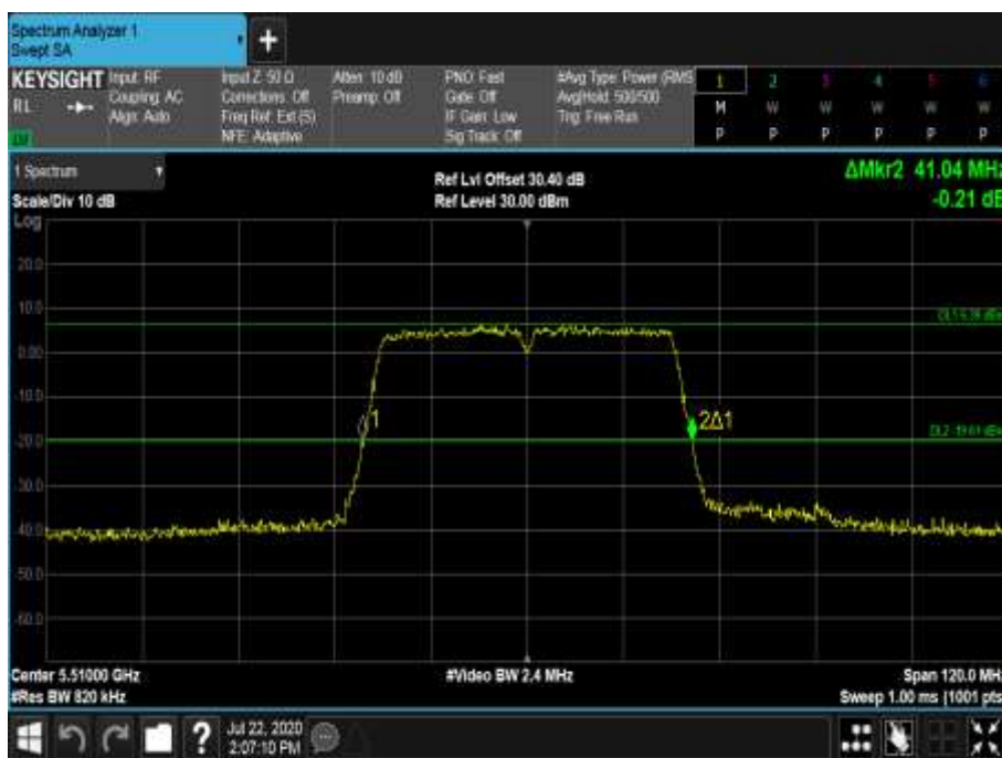
Figure 632 - 5510 MHz - 26 dB Emission Bandwidth
