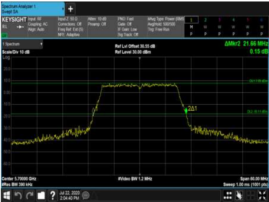
Figure 604 - 5700 MHz - 26 dB Emission Bandwidth
