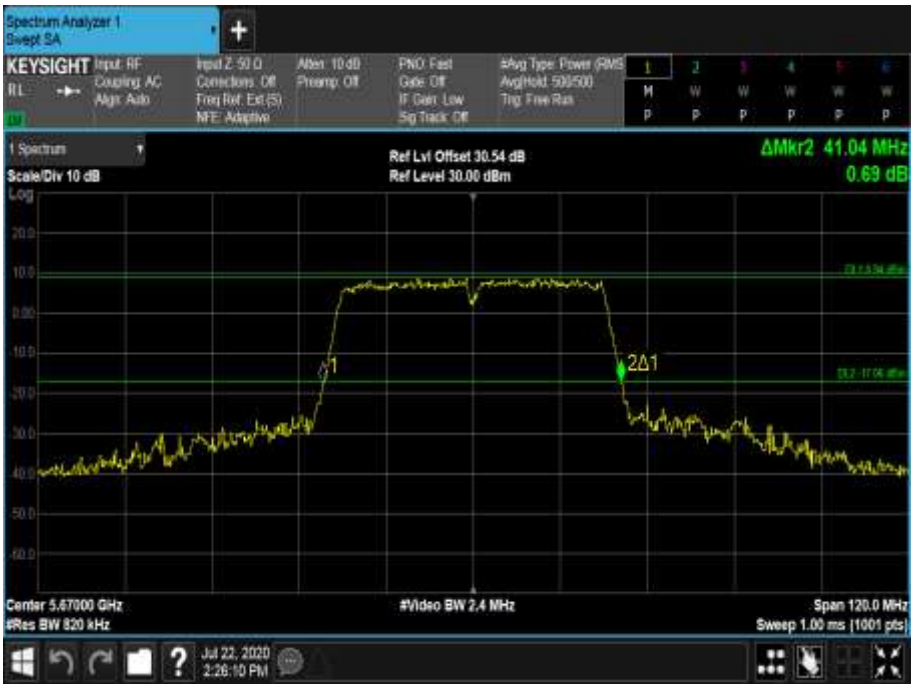
Figure 644 - 5670 MHz - 26 dB Emission Bandwidth
