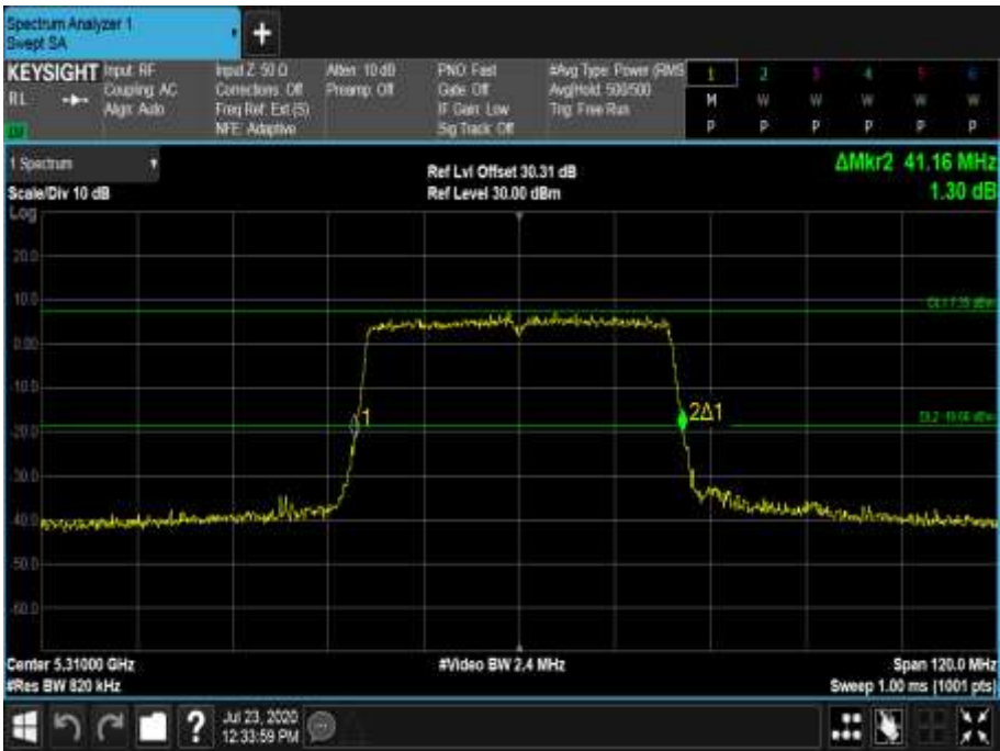
Figure 558 - 5310 MHz - 26 dB Emission Bandwidth
