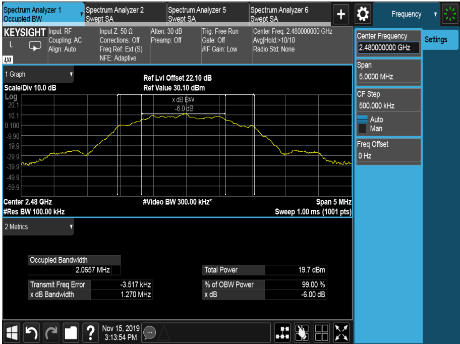
Figure 6 - 2480 MHz – Emission Bandwidth
