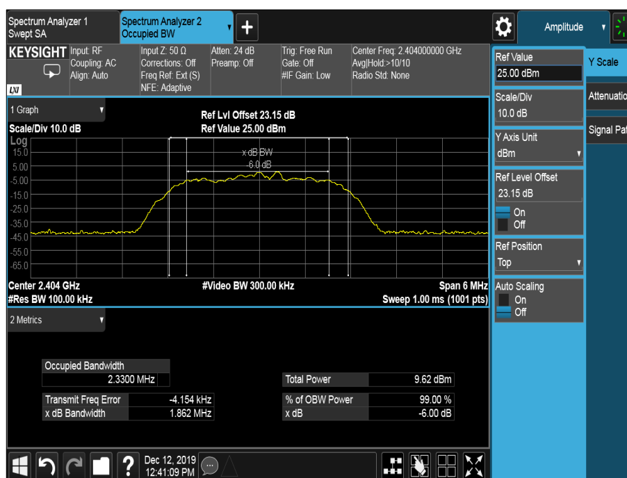
Figure 7 - 2404 MHz – Emission Bandwidth
