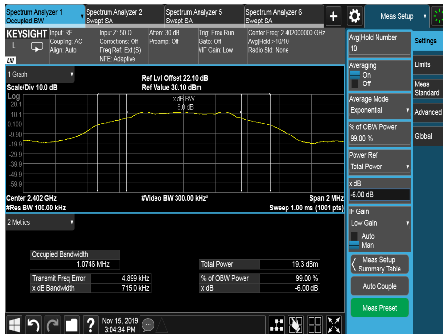
Figure 1 - 2402 MHz – Emission Bandwidth
