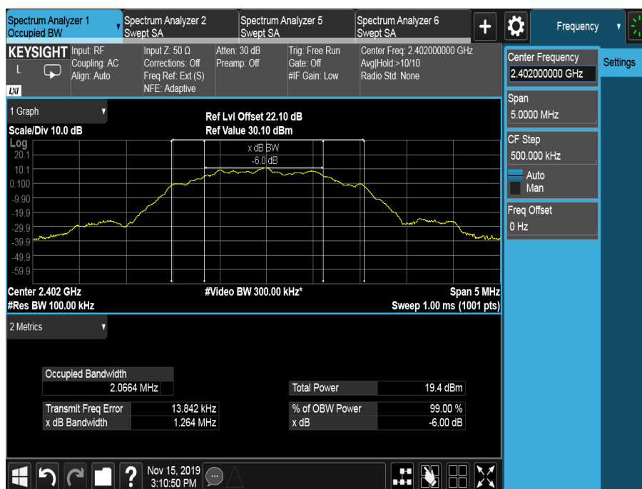
Figure 4 - 2402 MHz – Emission Bandwidth
