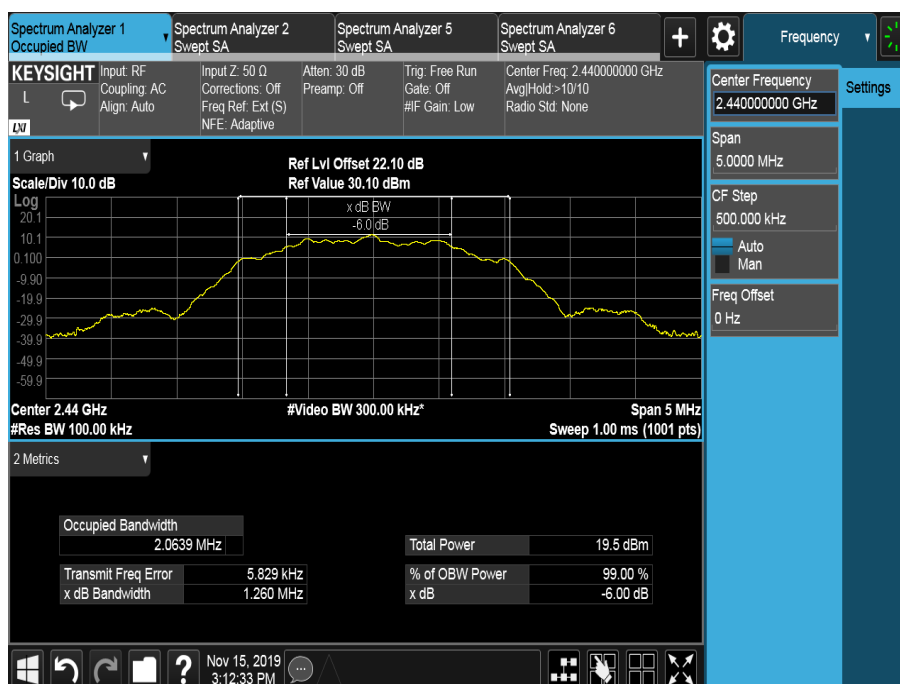
Figure 5 - 2440 MHz – Emission Bandwidth
