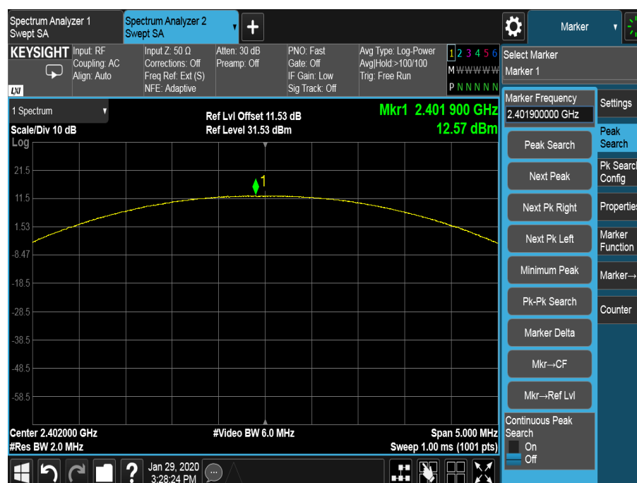
Figure 82 - 2402 MHz - Maximum Output Power
