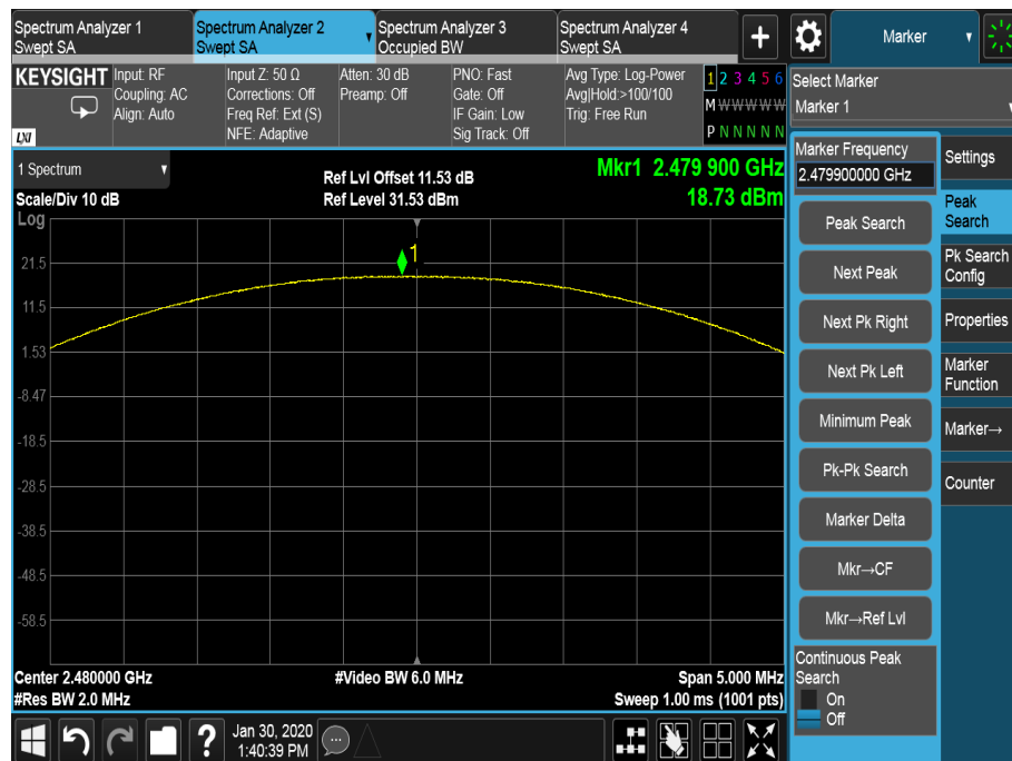
Figure 97 - 2480 MHz - Maximum Output Power
