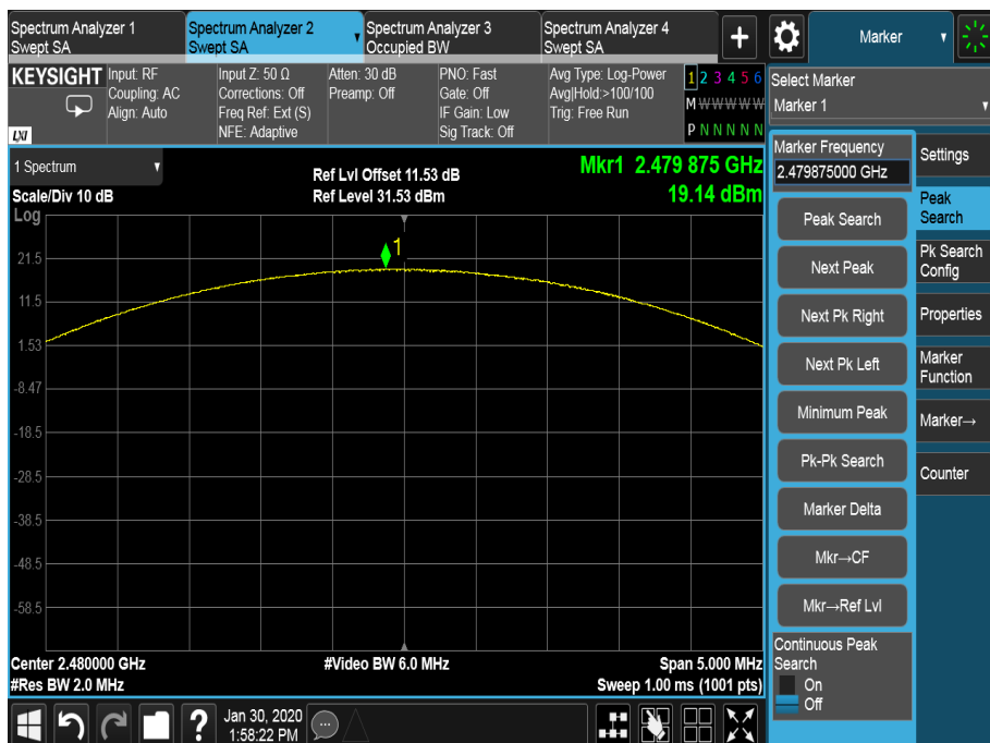
Figure 98 - 2480 MHz - Maximum Output Power
