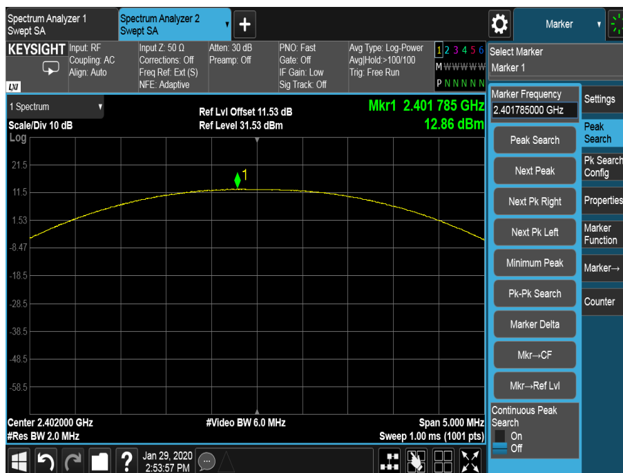
Figure 81 - 2402 MHz - Maximum Output Power
