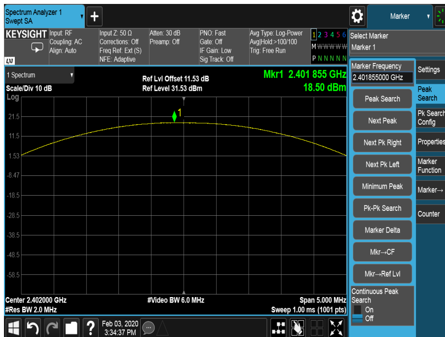
Figure 91 - 2402 MHz - Maximum Output Power
