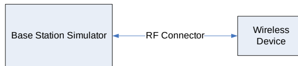
Figure 8-3 Power Measurement Setup
