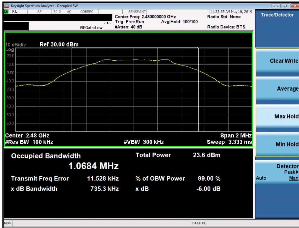
Plot 7-3. 6dB Bandwidth Plot (Bluetooth (LE), ePA – Ch. 39)
