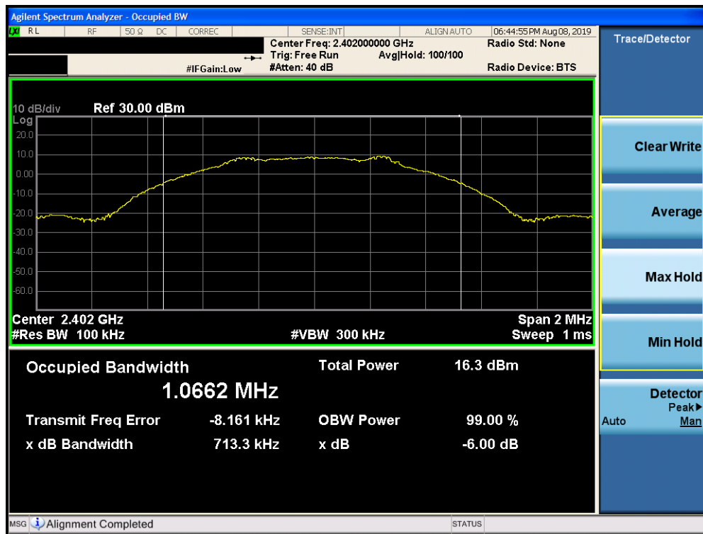
Plot 7-4. 6dB Bandwidth Plot (Bluetooth (LE), iPA – Ch. 0)
