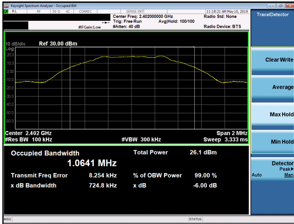
Plot 7-1. 6dB Bandwidth Plot (Bluetooth (LE), ePA – Ch. 0)
