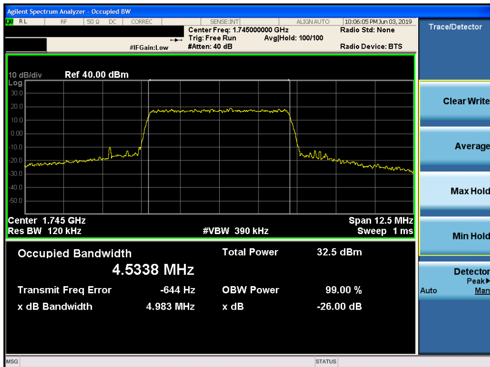
Plot 7-38. Occupied Bandwidth Plot (Band 66/4 - 5.0MHz 16-QAM - Full RB Configuration)
