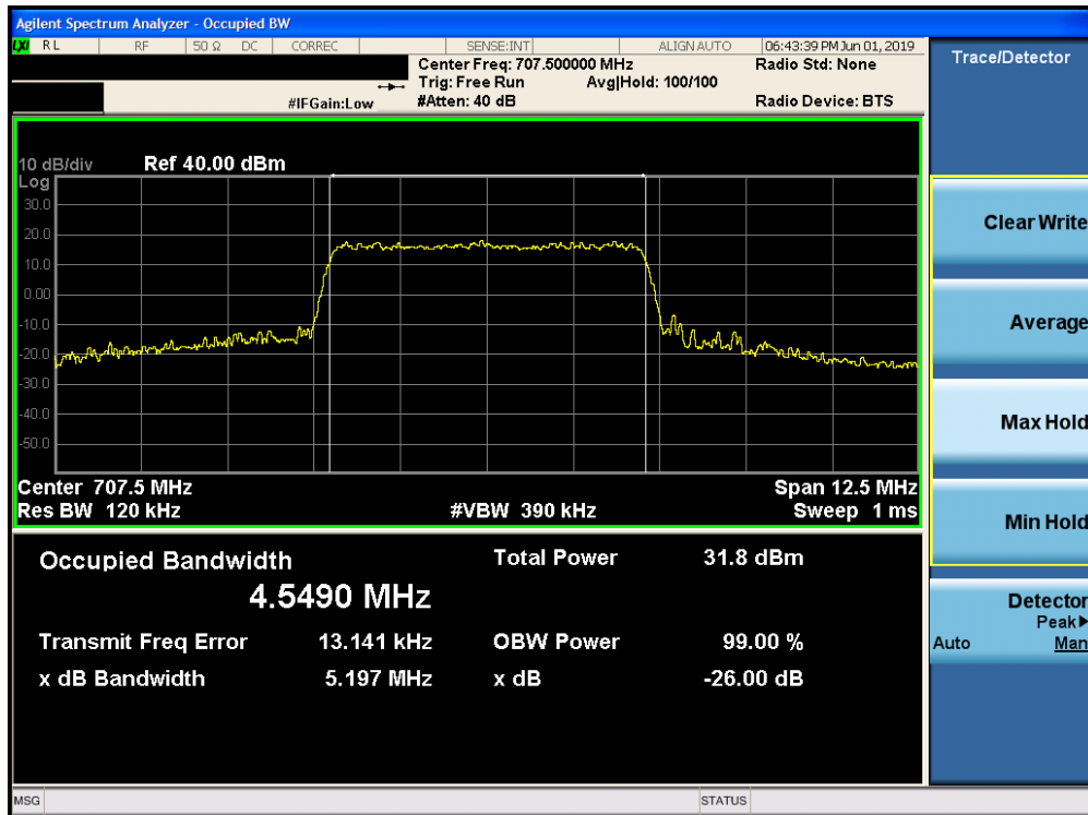
Plot 7-9. Occupied Bandwidth Plot (Band 12/17 - 5.0MHz 64-QAM - Full RB Configuration)
