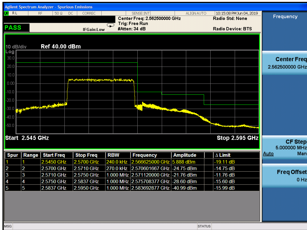
Plot 7-310. Upper ACP Plot (Band 7 - 15.0MHz QPSK - Full RB Configuration)
