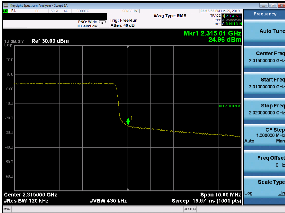
Plot 7-303. Upper Band Edge Plot (Band 30 - 10.0MHz QPSK - Full RB Configuration)
