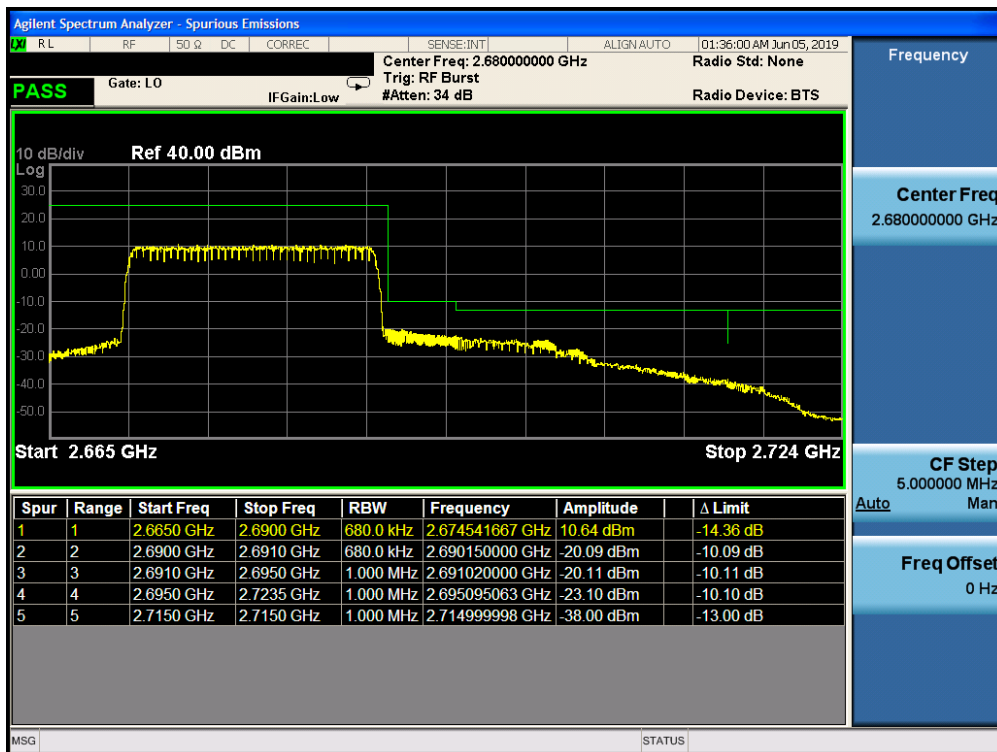
Plot 7-320. Upper ACP Plot (Band 41 - 20.0MHz QPSK - Full RB Configuration)
