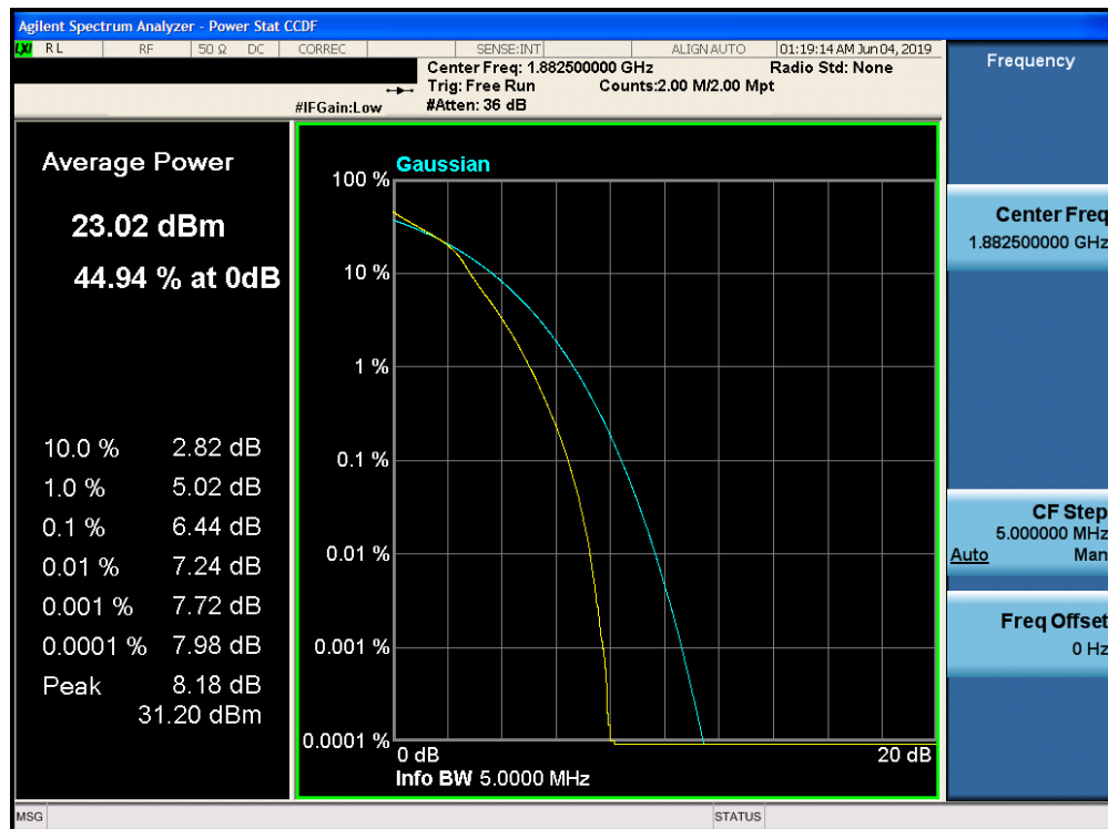
Plot 7-390. PAR Plot (Band 25 - 5.0MHz 16-QAM - Full RB Configuration)
