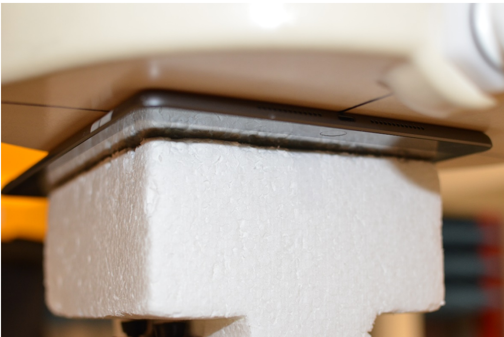
SAR Test Setup Photo 2: Back Side at 0.0 cm – Antenna A/Antenna B
