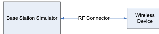
Figure 8-3 Power Measurement Setup
