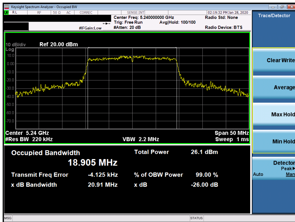
Plot 7-12. 26dB Bandwidth Plot SISO CORE 0 (20MHz BW 802.11ax- RU242 (UNII Band 1) – Ch. 48)
