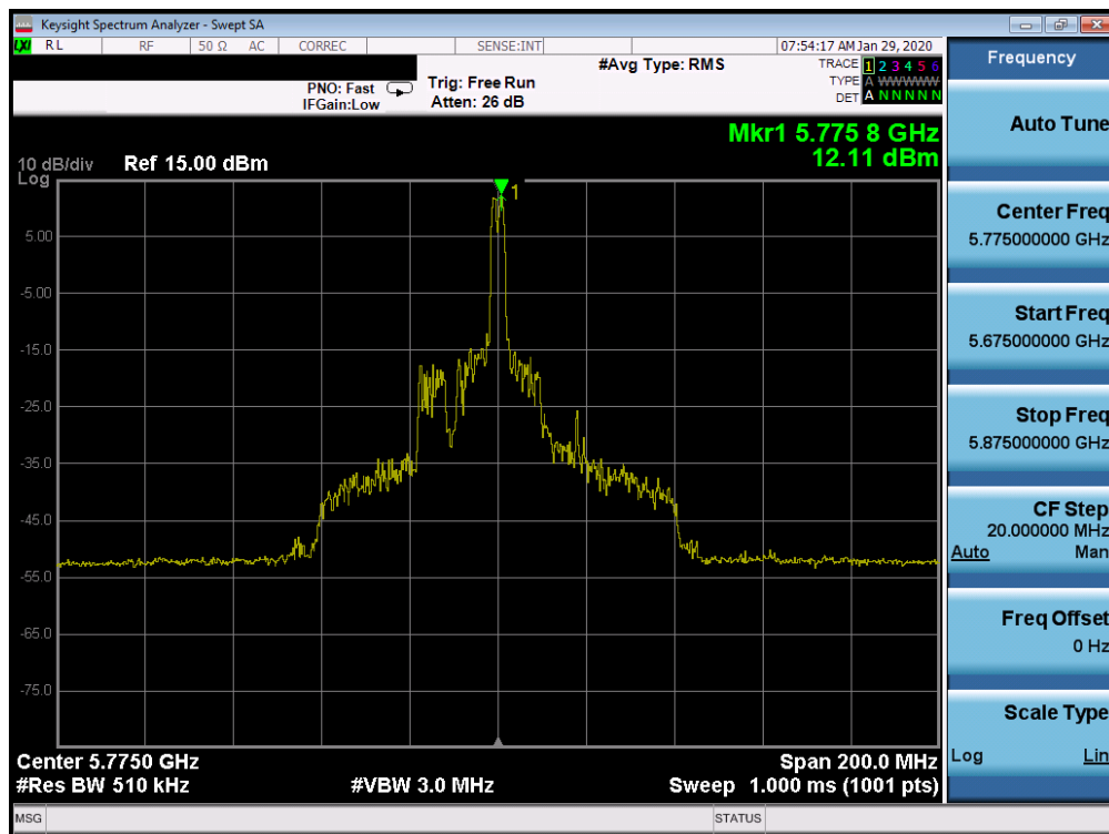
Plot 7-435. Power Spectral Density Plot SISO CORE 1 (80MHz BW 802.11ax Index 18 – RU26 (UNII Band 3) – Ch. 155)
