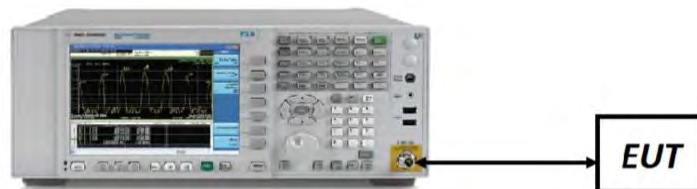
Figure 7-3. Test Instrument & Measurement Setup
