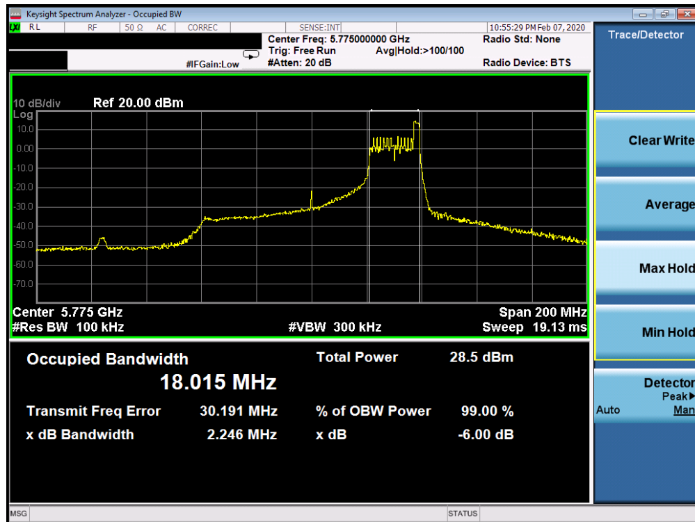
Plot 7-183. 6dB Bandwidth Plot SISO CORE 0 (80MHz BW 802.11ax Index 36 – RU26 (UNII Band 3) – Ch. 155)
