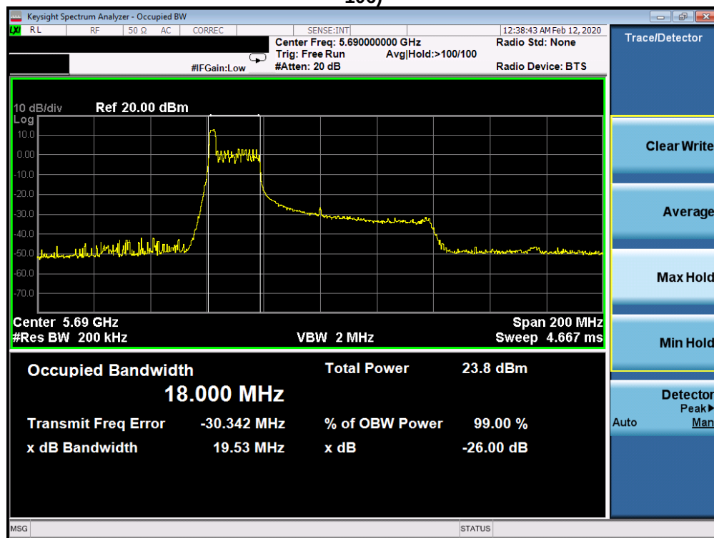
Plot 7-156. 26dB Bandwidth Plot SISO CORE 1 (80MHz BW 802.11ax Index 0 – RU26 (UNII Band 2C) – Ch. 138)
