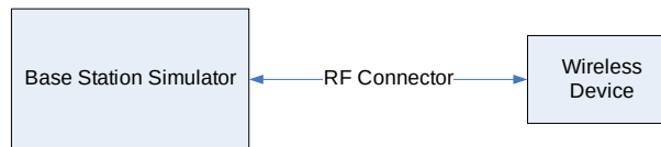
Figure 8-3 Power Measurement Setup
