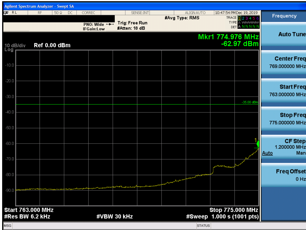
Plot 7-182. Lower Emission Mask Edge Plot (Band 13 – 5.0MHz QPSK – RB Size 25)
