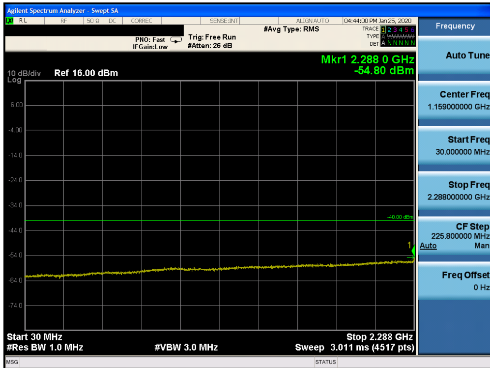
Plot 7-148. Conducted Spurious Plot (Band 30 – 5.0MHz QPSK – RB Size 1, RB Offset 0 – Mid Channel)
