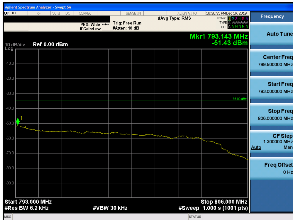
Plot 7-188. Upper Emission Mask Edge Plot (Band 13 – 10.0MHz QPSK – RB Size 50)
