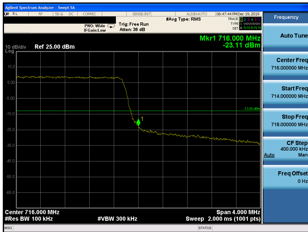
Plot 7-174. Upper Band Edge Plot (Band 12 – 5.0MHz QPSK – RB Size 25)
