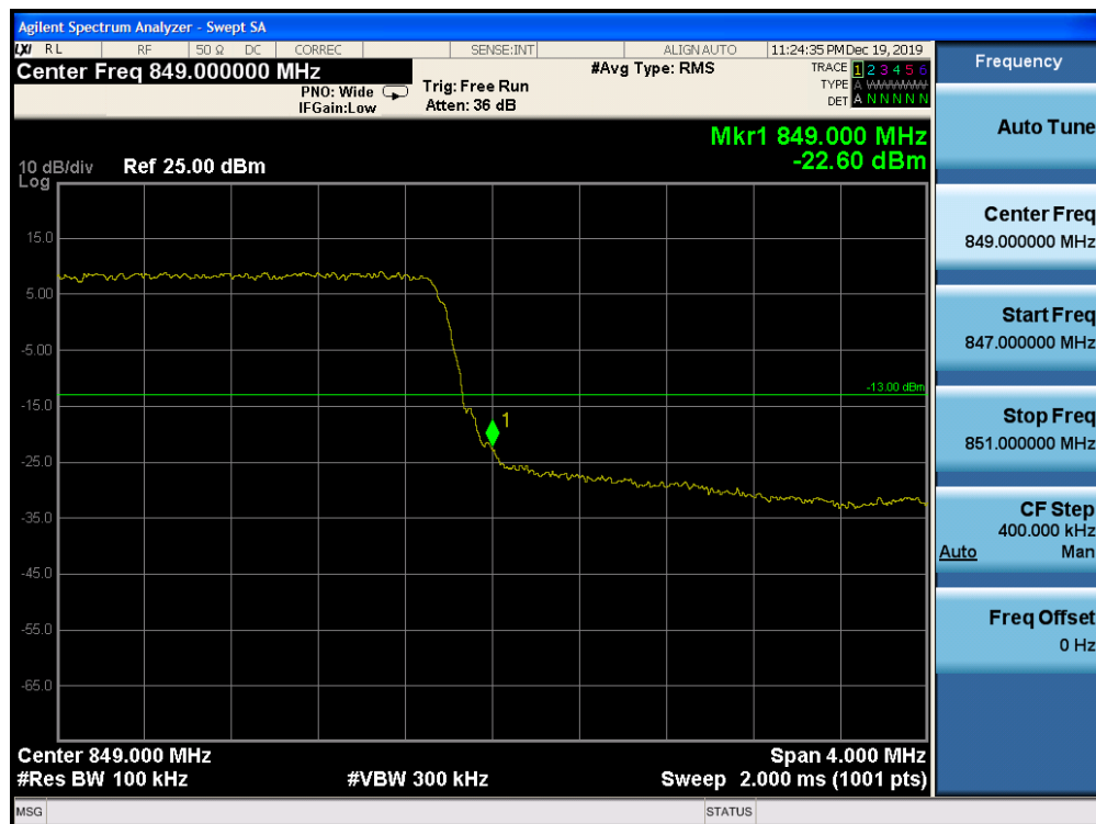
Plot 7-194. Upper Band Edge Plot (Band 5 – 5.0MHz QPSK – RB Size 25)
