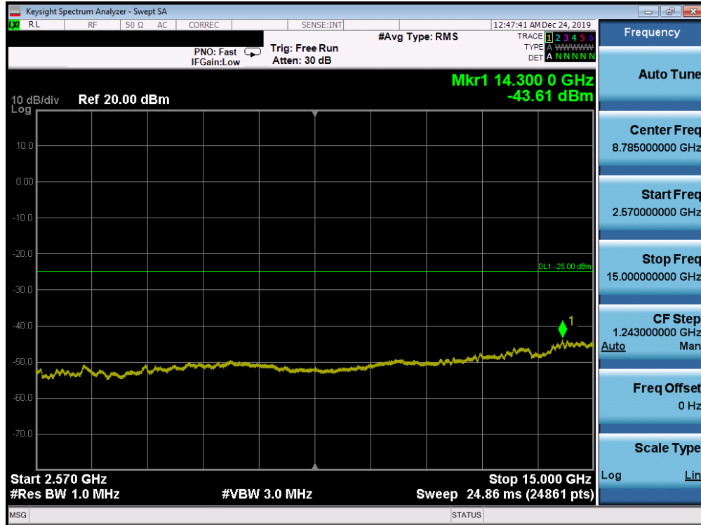
Plot 7-155. Conducted Spurious Plot (Band 7 – 20.0MHz QPSK – RB Size 1, RB Offset 0 – Mid Channel)
