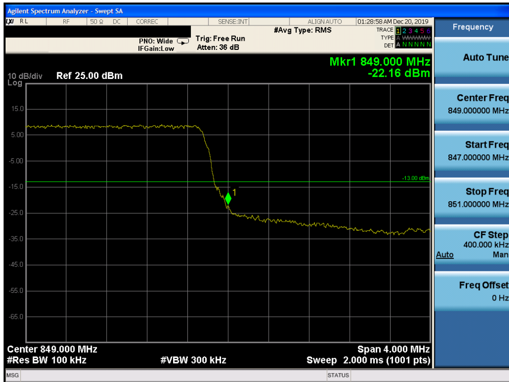
Plot 7-202. Upper Band Edge Plot (Band 5 – 5.0MHz QPSK – RB Size 25)
