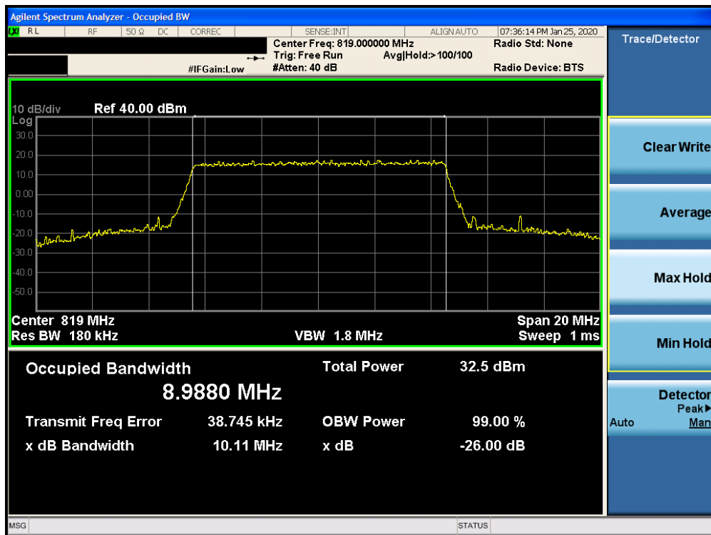
Plot 7-3. Occupied Bandwidth Plot (LTE Band 26 - 10MHz 64-QAM - Full RB Configuration)
