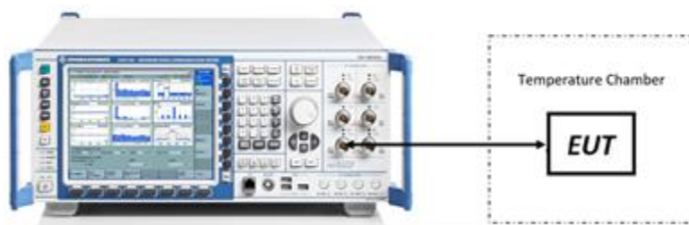
Figure 7-6. Test Instrument & Measurement Setup
