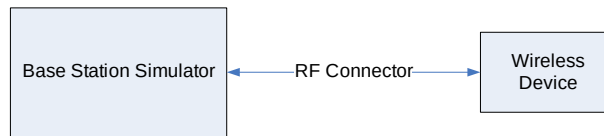
Figure 8-2 Power Measurement Setup
