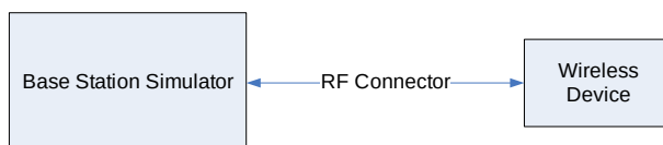
Figure 8-1 Power Measurement Setup
