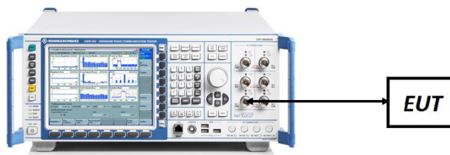
Figure 7-5. ERP/EIRP Measurement Setup
