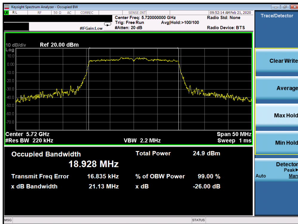
Plot 7-140. 26dB Bandwidth Plot SISO CORE 1 (20MHz BW 802.11ax– RU242 (UNII Band 2C) – Ch. 144)
