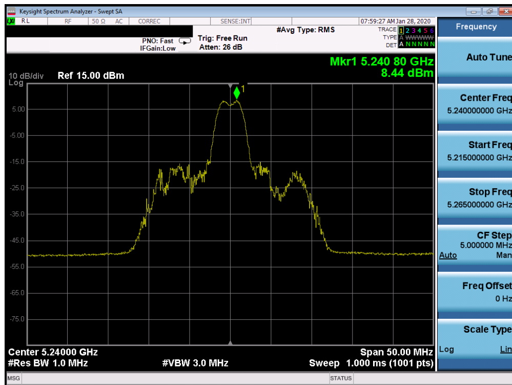
Plot 7-216. Power Spectral Density Plot SISO CORE 0 (20MHz BW 802.11ax Index 4 – RU26 (UNII Band 1) – Ch. 48)
