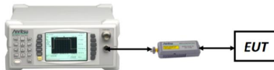
Figure 7-2. Radiated Measurement Setup for Power Meter Measurements
