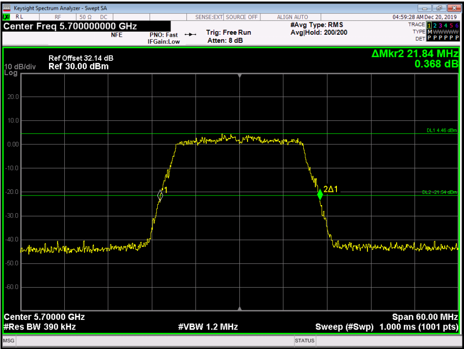
Figure 191 - 5700 MHz - 26 dB Emission Bandwidth
