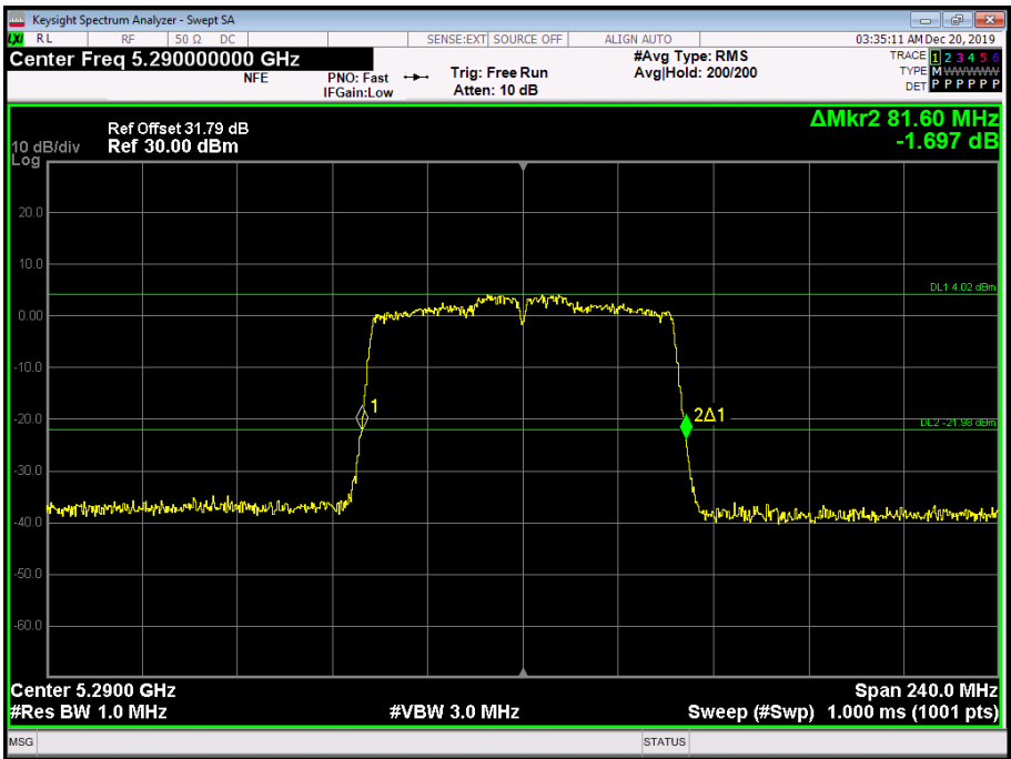
Figure 155 - 5290 MHz - 26 dB Emission Bandwidth
