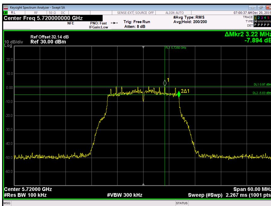
Figure 259 - 5720 MHz - 6 dB DTS Bandwidth
