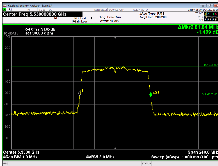
Figure 235 - 5530 MHz - 26 dB Emission Bandwidth
