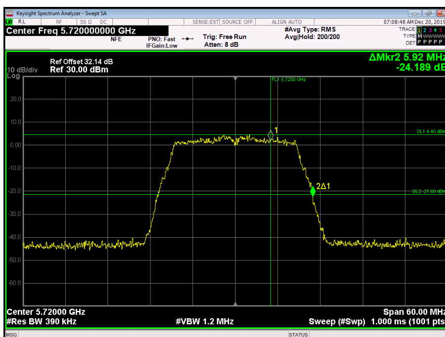
Figure 272 - 5720 MHz - 26 dB Emission Bandwidth
