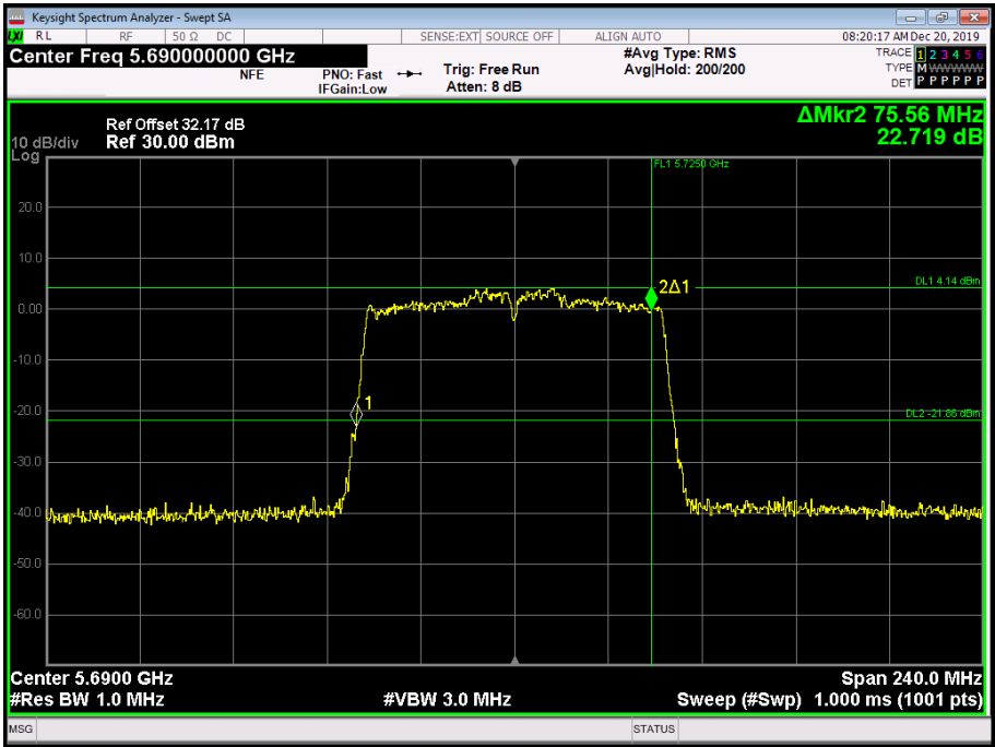
Figure 251 - 5690 MHz - 26 dB Emission Bandwidth
