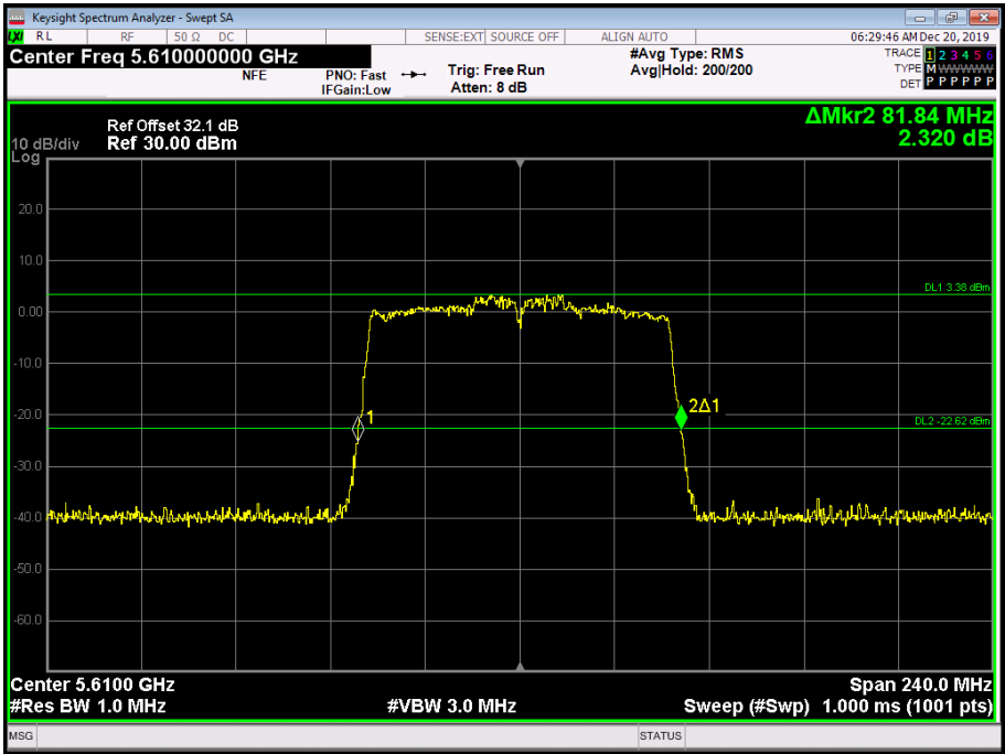
Figure 249 - 5610 MHz - 26 dB Emission Bandwidth
