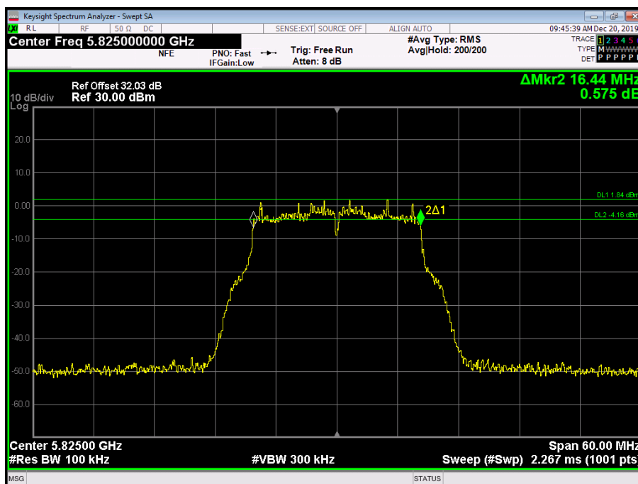
Figure 268 - 5825 MHz - 6 dB DTS Bandwidth
