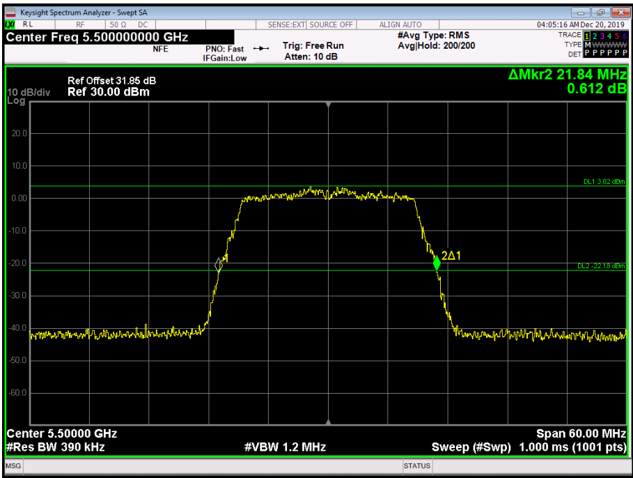
Figure 179 - 5500 MHz - 26 dB Emission Bandwidth
