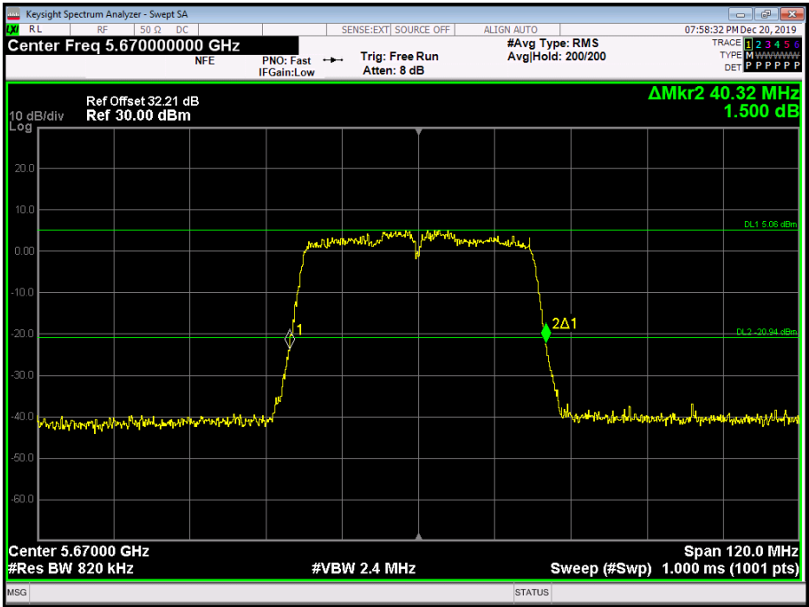
Figure 207 - 5670 MHz - 26 dB Emission Bandwidth
