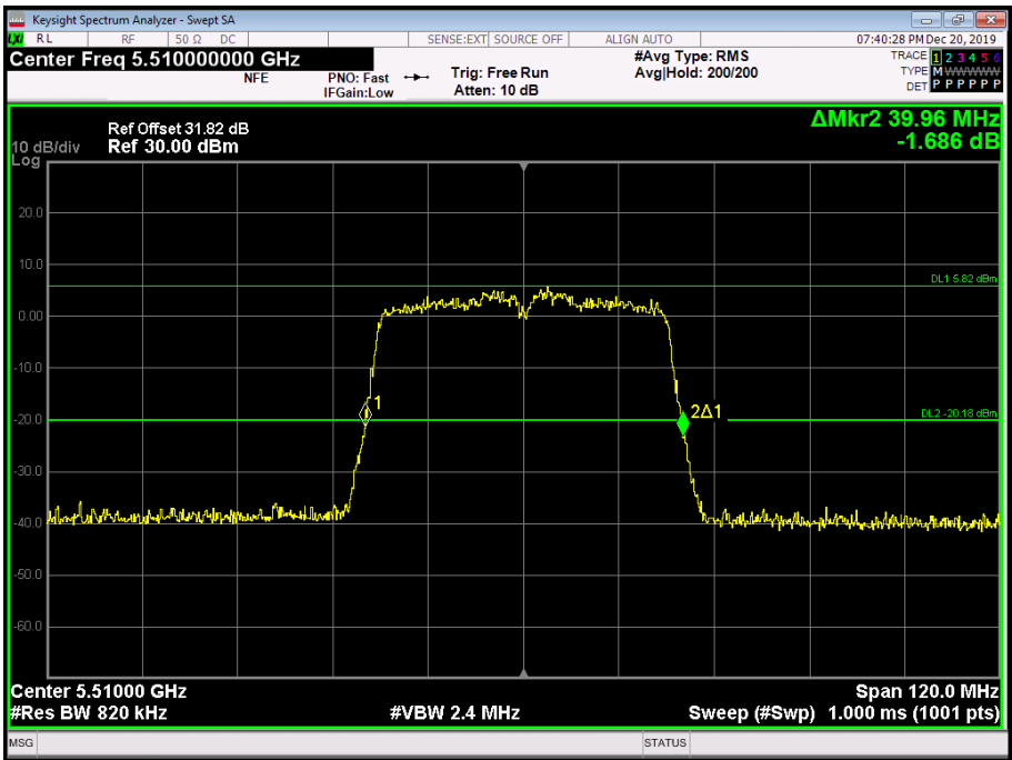
Figure 211 - 5510 MHz - 26 dB Emission Bandwidth
