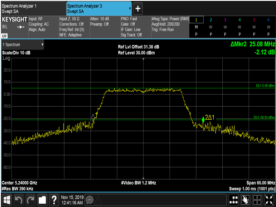
Figure 35 - 5240 MHz - 26 dB Emission Bandwidth
