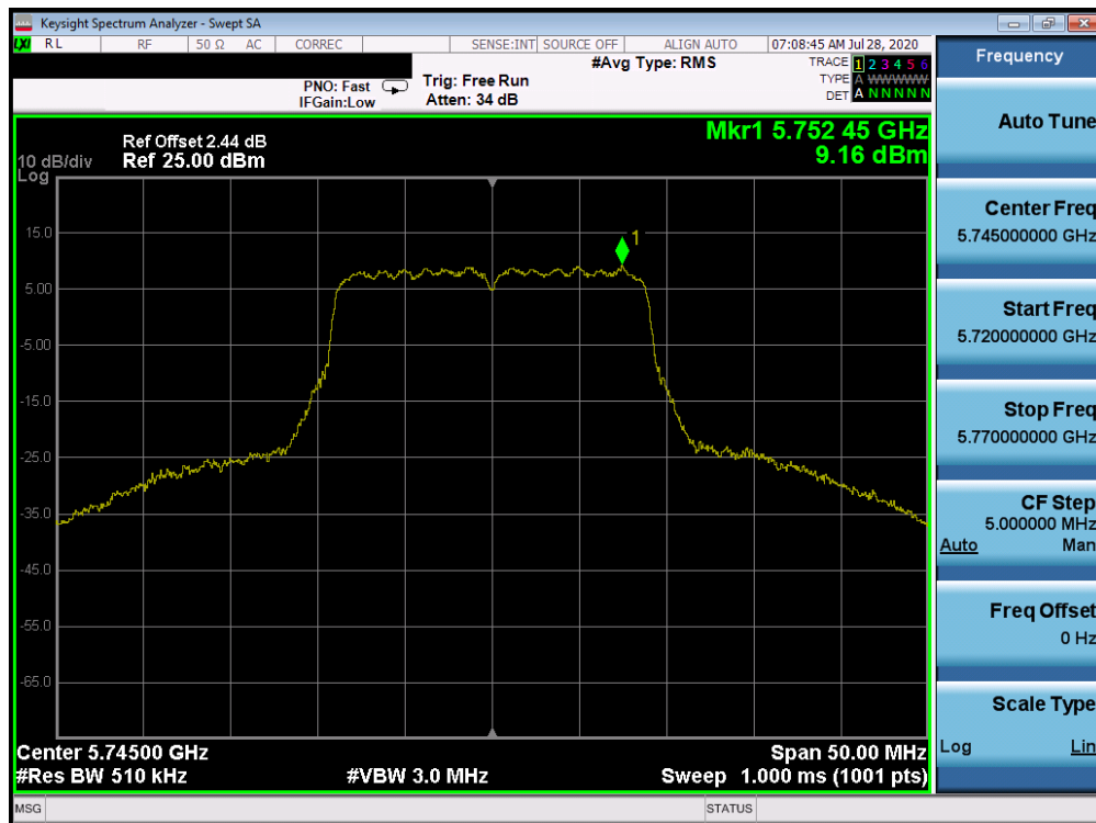
Plot 7-162. Power Spectral Density Plot CDD ANT WF7a (20MHz BW 802.11n (UNII Band 3) – Ch. 149)
