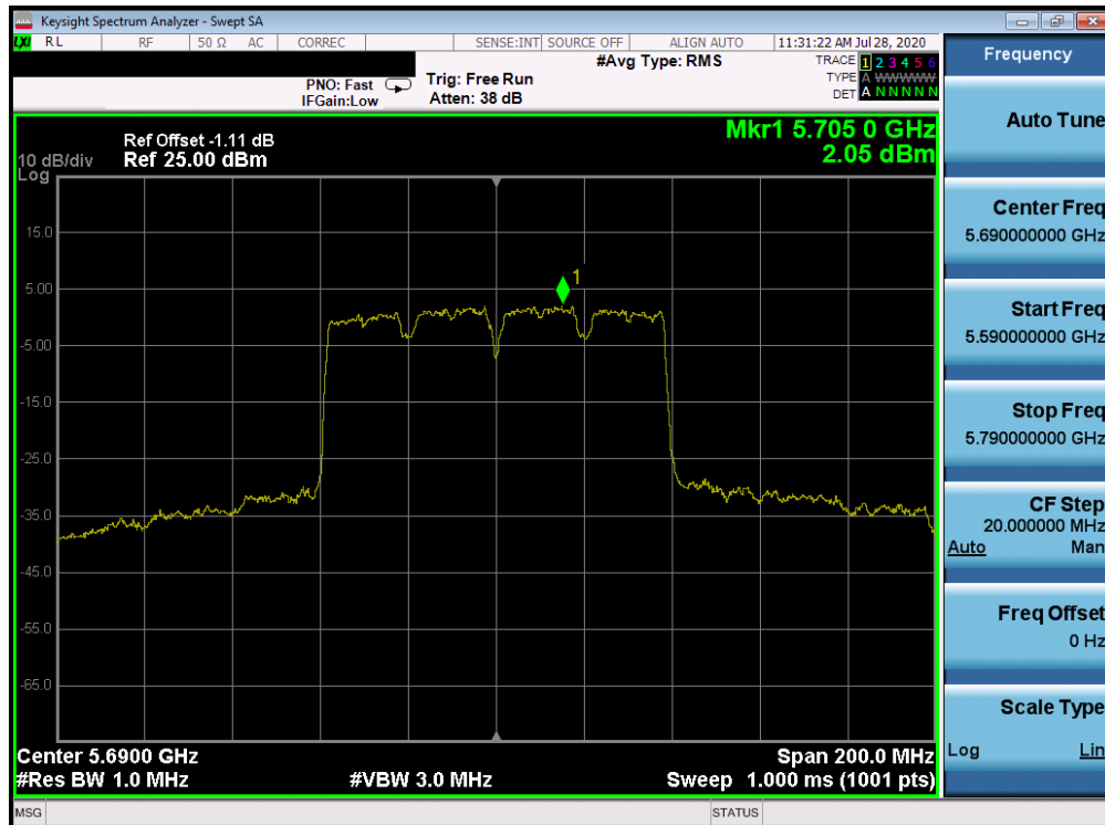
Plot 7-160. Power Spectral Density Plot CDD ANT WF7a (80MHz BW 802.11ac (UNII Band 2C) – Ch. 138)
