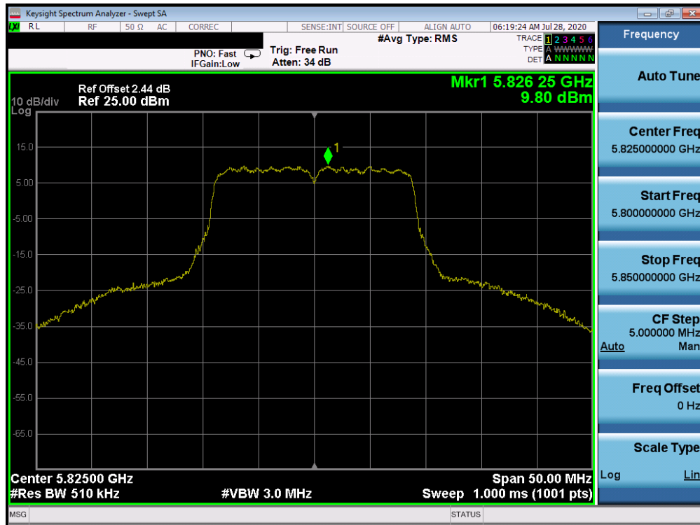
Plot 7-165. Power Spectral Density Plot CDD ANT WF8 (20MHz BW 802.11n (UNII Band 3) – Ch. 165)
