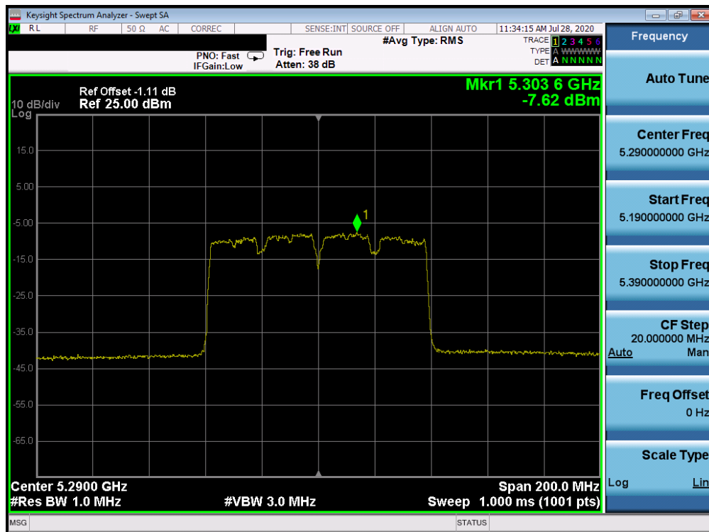
Plot 7-144. Power Spectral Density Plot CDD ANT WF7a (80MHz BW 802.11ac (UNII Band 2A) – Ch. 58)
