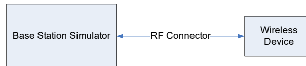
Figure 8-3 Power Measurement Setup
