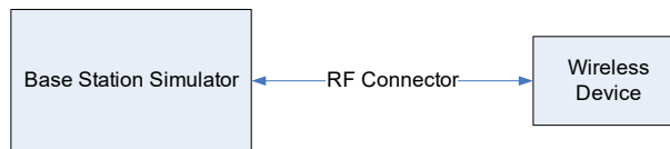
Figure 8-2 Power Measurement Setup
