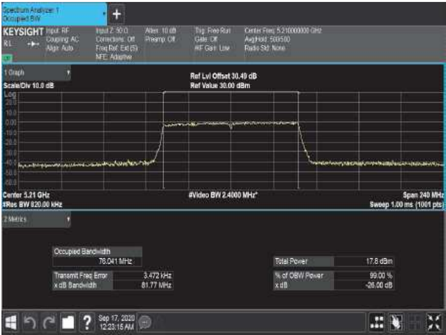
Figure 276 - 5210 MHz - 99% Occupied Bandwidth
