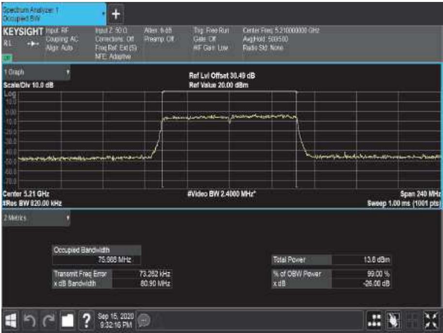
Figure 284 - 5210 MHz - 99% Occupied Bandwidth
