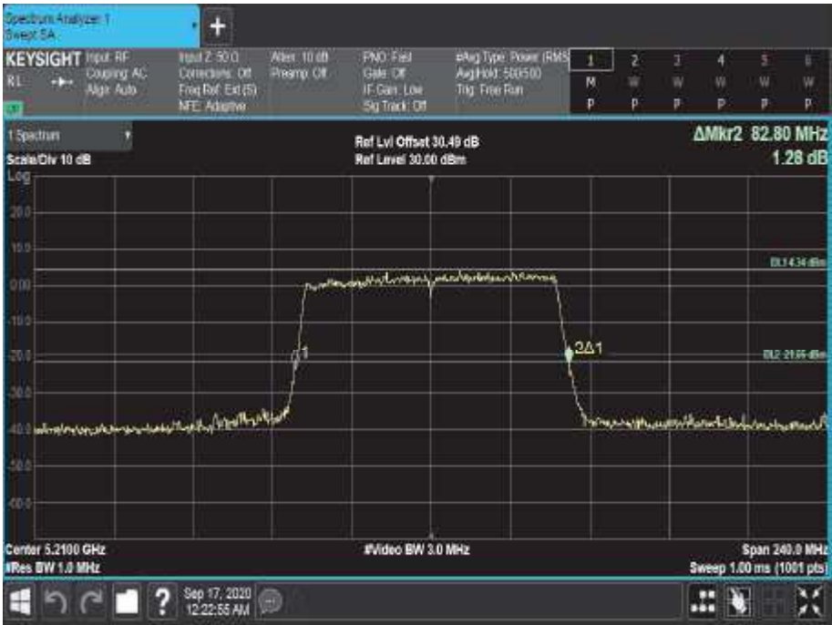
Figure 275 - 5210 MHz - 26 dB Emission Bandwidth
