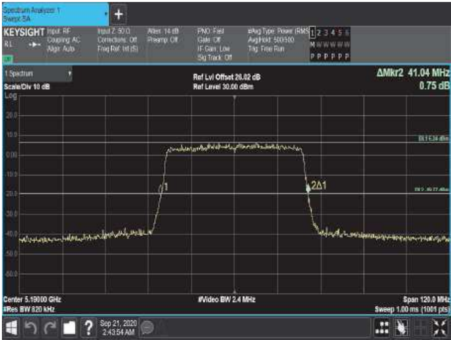
Figure 205 - 5190 MHz - 26 dB Emission Bandwidth
