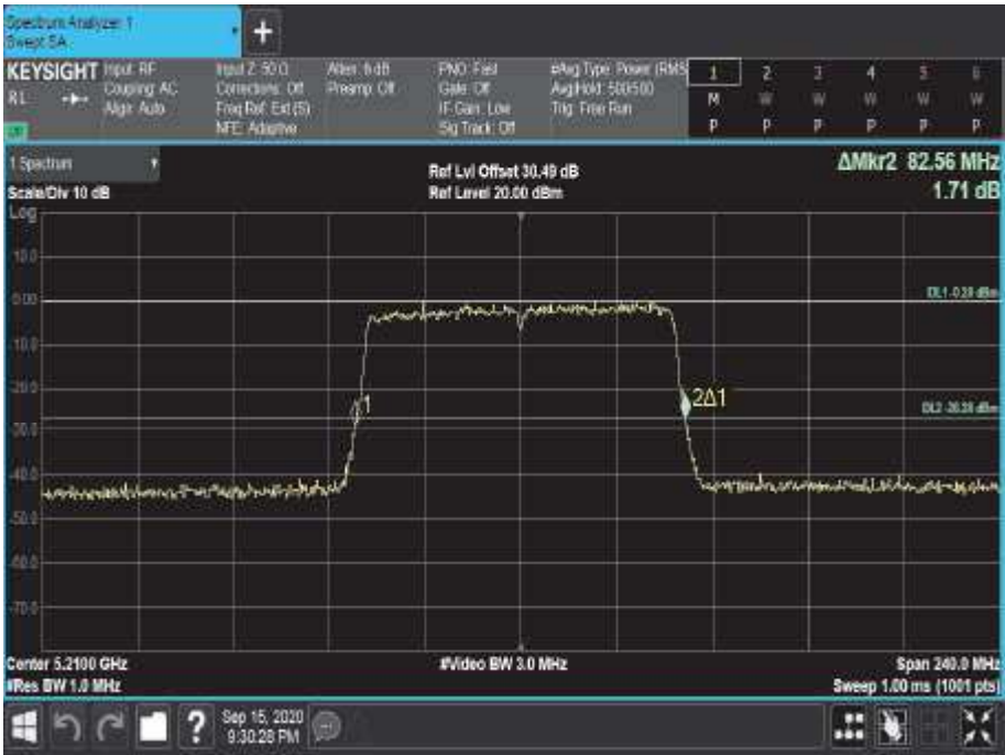
Figure 279 - 5210 MHz - 26 dB Emission Bandwidth
