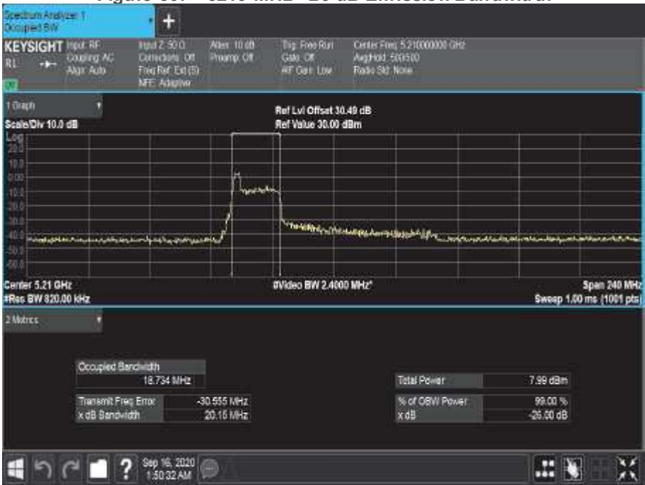
Figure 308 - 5210 MHz - 99% Occupied Bandwidth
