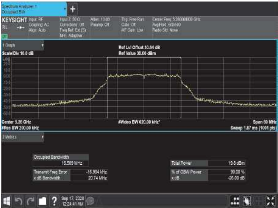
Figure 326 - 5260 MHz - 99% Occupied Bandwidth
