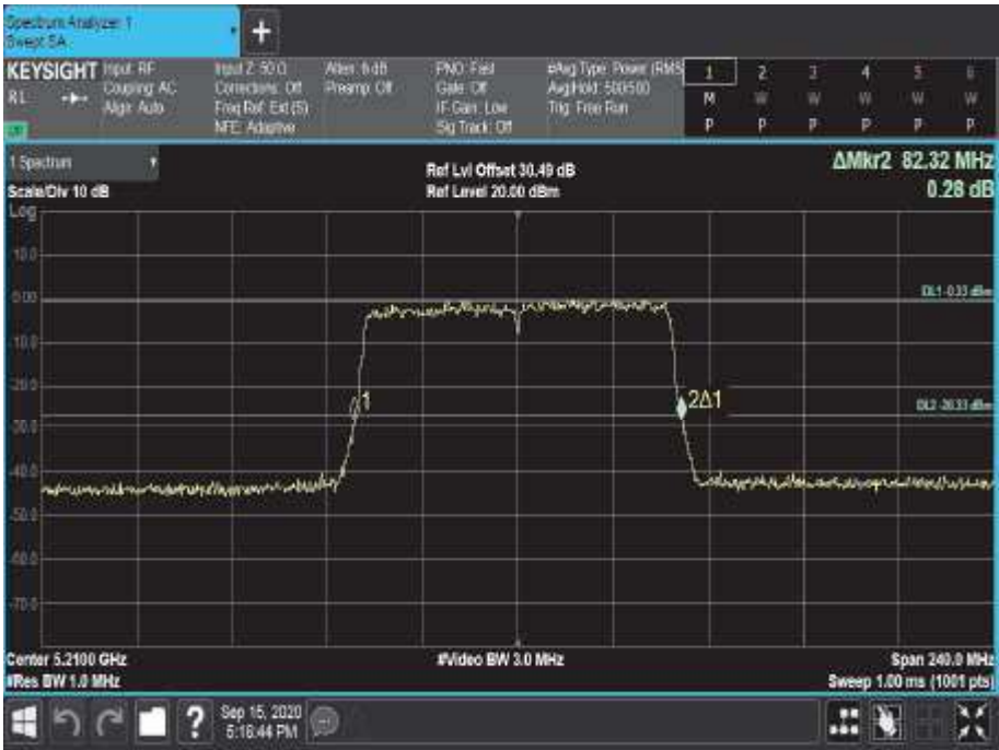
Figure 283 - 5210 MHz - 26 dB Emission Bandwidth
