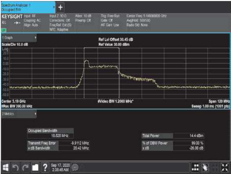
Figure 210 - 5190 MHz - 99% Occupied Bandwidth
