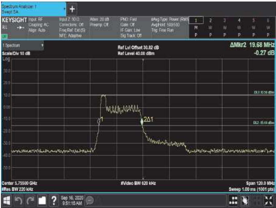
Figure 782 - 5755 MHz - 26 dB Emission Bandwidth
