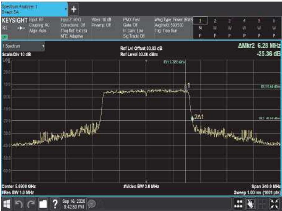
Figure 833 - 5690 MHz - 26 dB Emission Bandwidth
