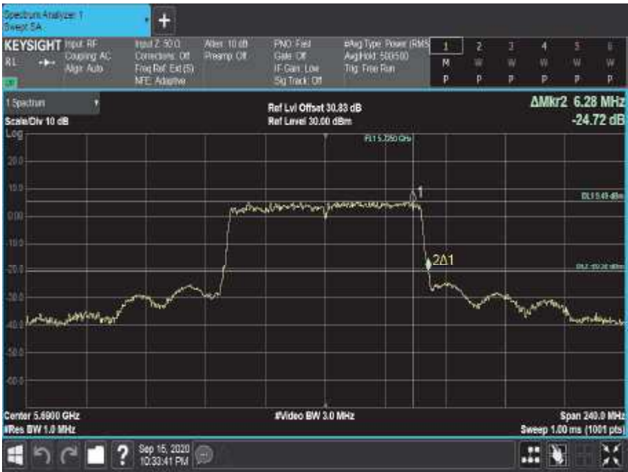
Figure 827 - 5690 MHz - 26 dB Emission Bandwidth
