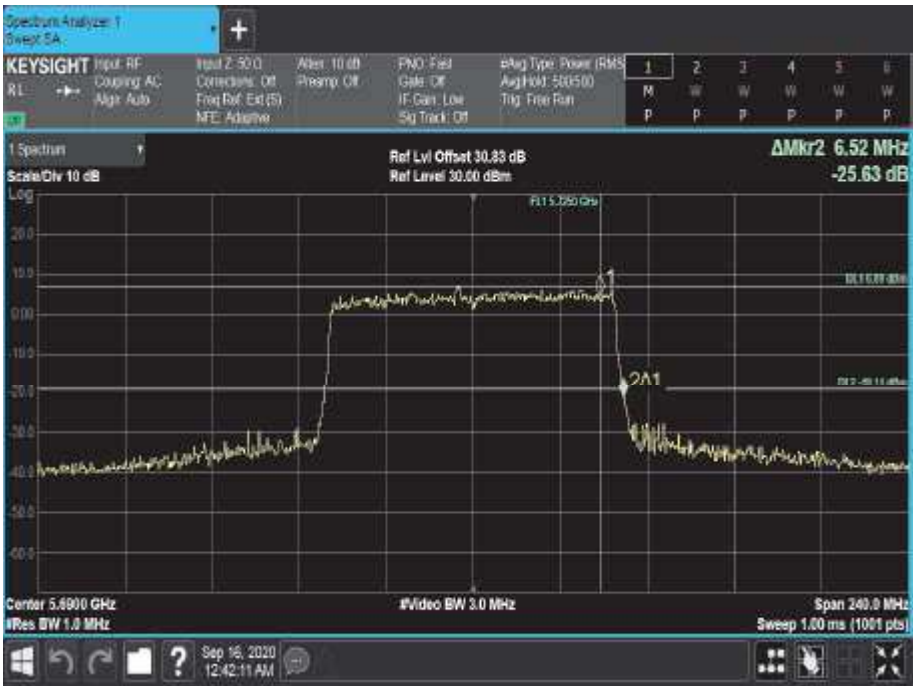
Figure 863 - 5690 MHz - 26 dB Emission Bandwidth
