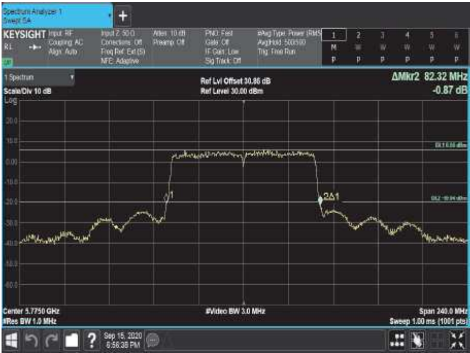
Figure 830 - 5775 MHz - 26 dB Emission Bandwidth
