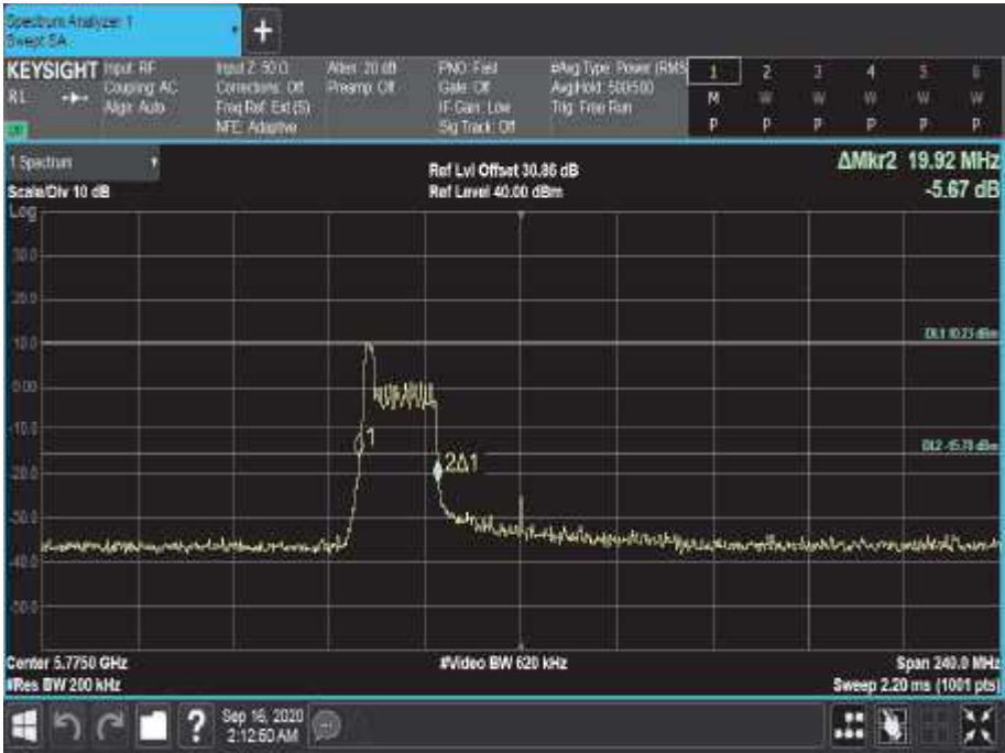
Figure 857 - 5775 MHz - 26 dB Emission Bandwidth
