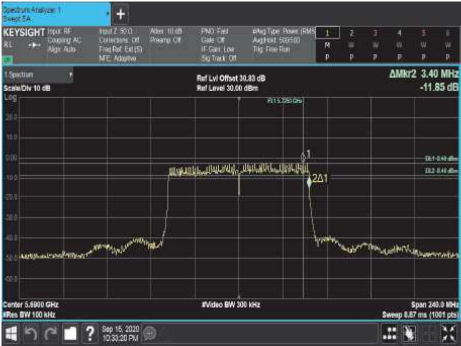
Figure 826 - 5690 MHz - 6 dB DTS Bandwidth
