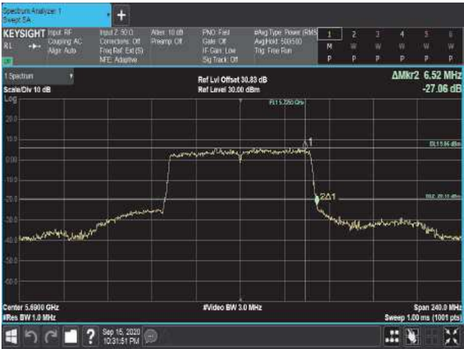
Figure 821 - 5690 MHz - 26 dB Emission Bandwidth
