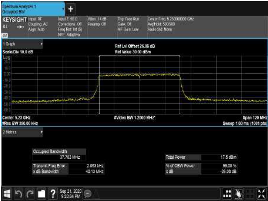
Figure 148 - 5230 MHz - 99% Occupied Bandwidth
