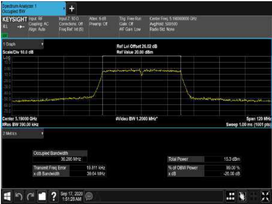
Figure 110 - 5190 MHz - 99% Occupied Bandwidth
