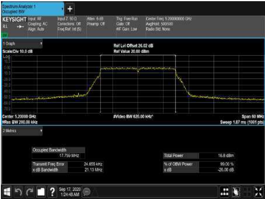
Figure 28 - 5200 MHz - 99% Occupied Bandwidth
