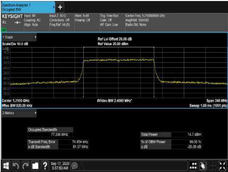
Figure 180 - 5210 MHz - 99% Occupied Bandwidth
