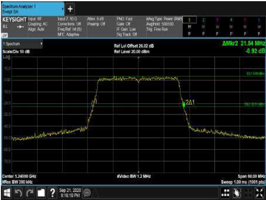
Figure 95 - 5240 MHz - 26 dB Emission Bandwidth
