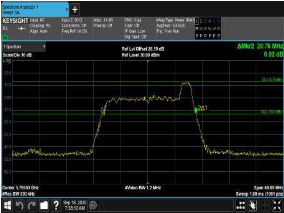
Figure 566 - 5785 MHz - 26 dB Emission Bandwidth
