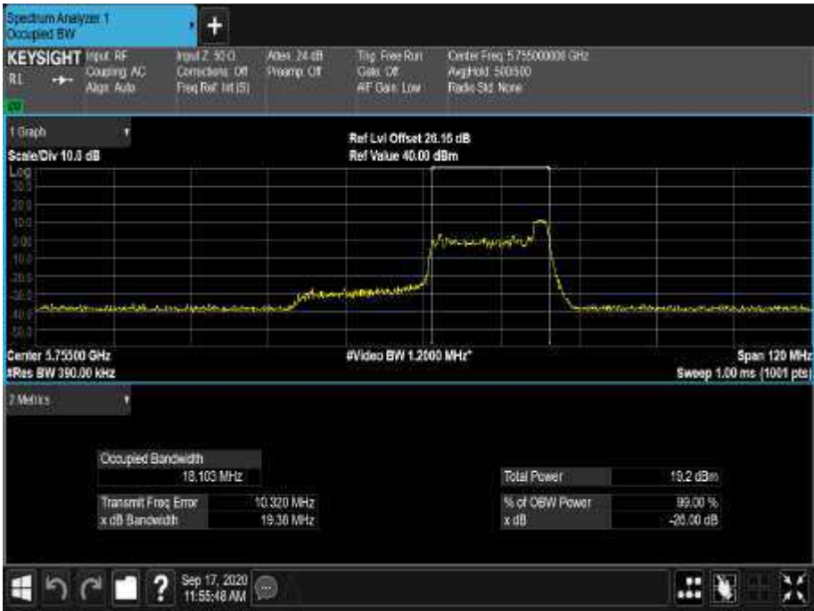
Figure 624 - 5755 MHz - 99% Occupied Bandwidth
