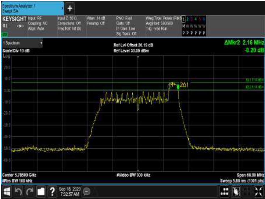
Figure 535 - 5785 MHz - 6 dB DTS Bandwidth
