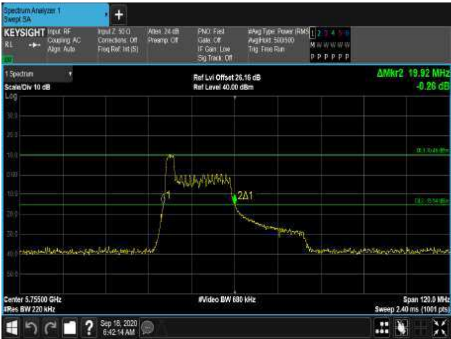
Figure 638 - 5755 MHz - 26 dB Emission Bandwidth
