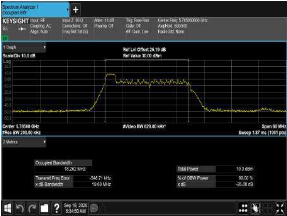
Figure 528 - 5785 MHz - 99% Occupied Bandwidth
