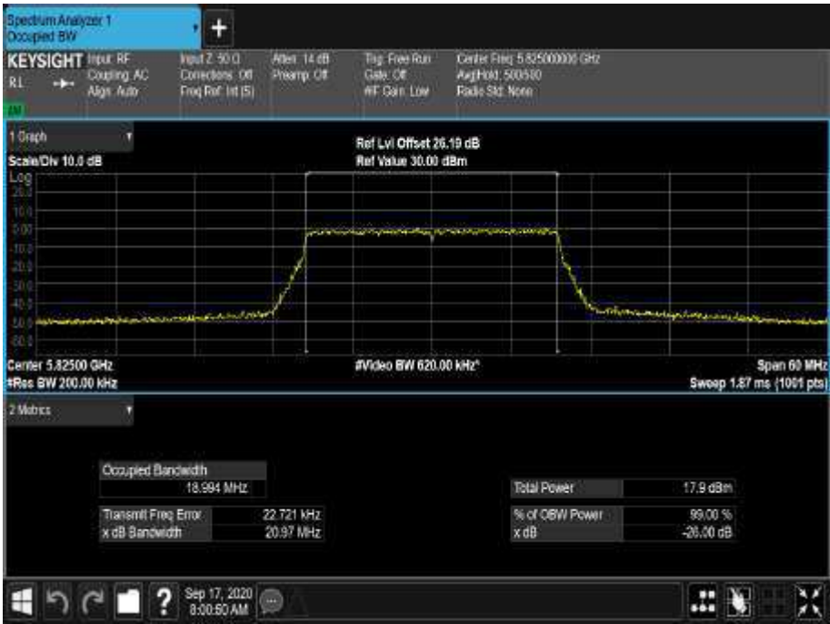
Figure 492 - 5825 MHz - 99% Occupied Bandwidth
