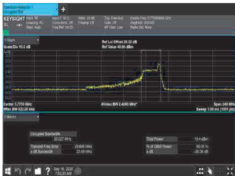
Figure 729 - 5775 MHz - 99% Occupied Bandwidth
