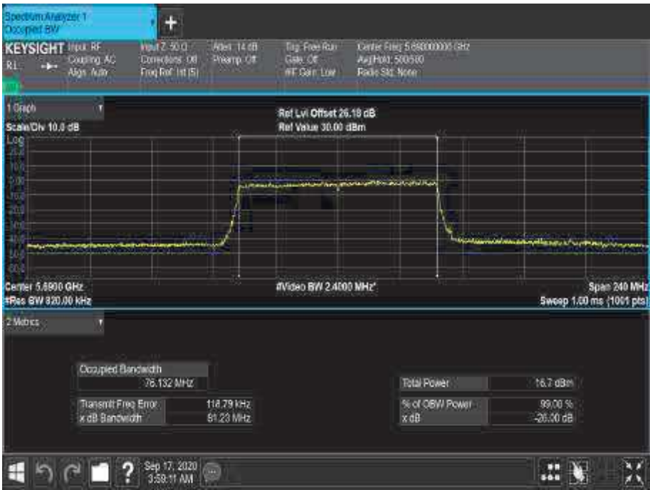
Figure 672 - 5690 MHz - 99% Occupied Bandwidth
