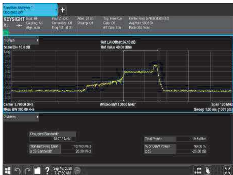
Figure 669 - 5795 MHz - 99% Occupied Bandwidth
