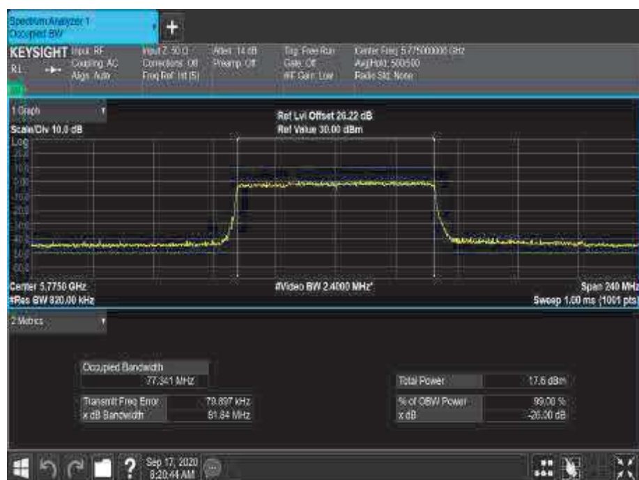
Figure 699 - 5775 MHz - 99% Occupied Bandwidth
