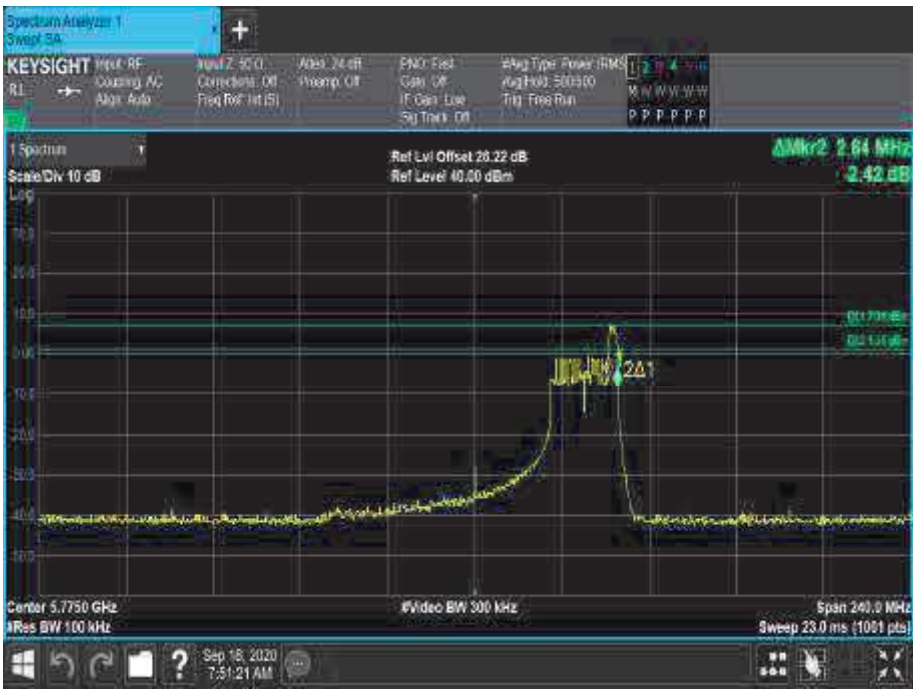
Figure 727 - 5775 MHz - 6 dB DTS Bandwidth
