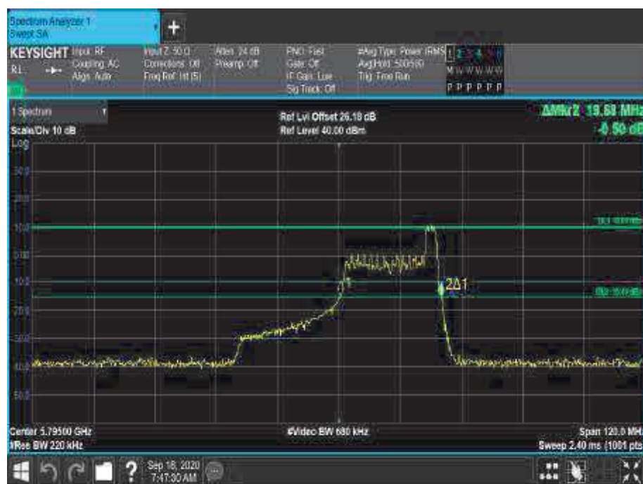
Figure 668 - 5795 MHz - 26 dB Emission Bandwidth
