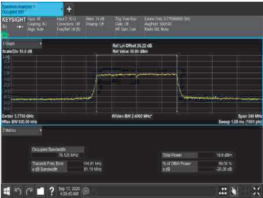
Figure 681 - 5775 MHz - 99% Occupied Bandwidth
