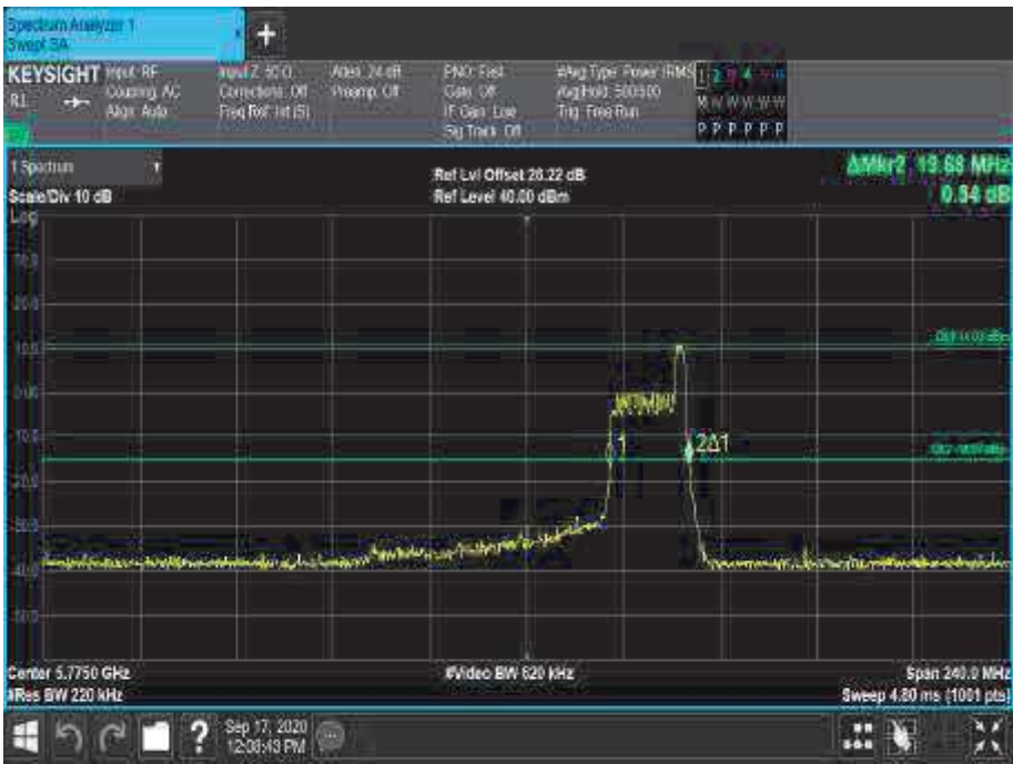
Figure 704 - 5775 MHz - 26 dB Emission Bandwidth
