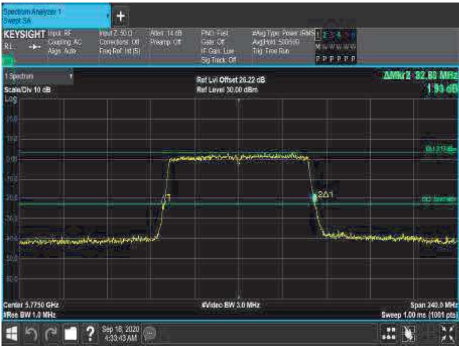
Figure 680 - 5775 MHz - 26 dB Emission Bandwidth
