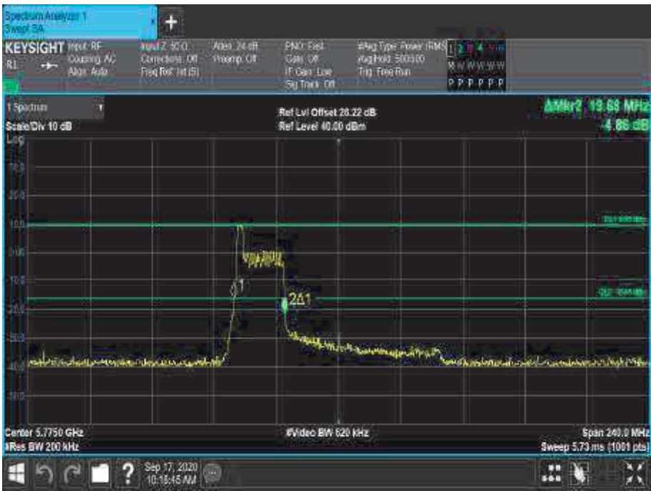
Figure 701 - 5775 MHz - 26 dB Emission Bandwidth
