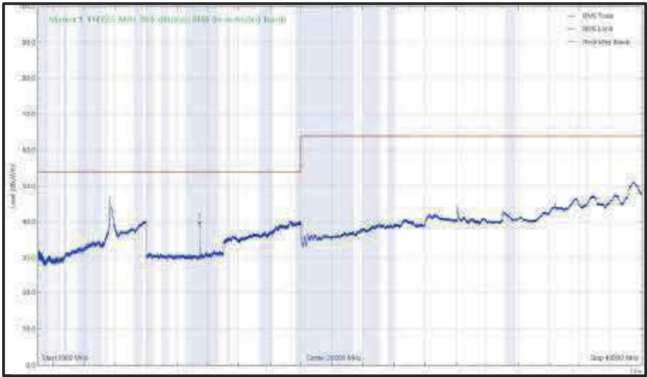
Figure 964 - 5745 MHz (CH1 49), HE 20, RU26-0, Core 0 + Core 1, 1 GHz to 40 GHz, Vertical (RMS)
