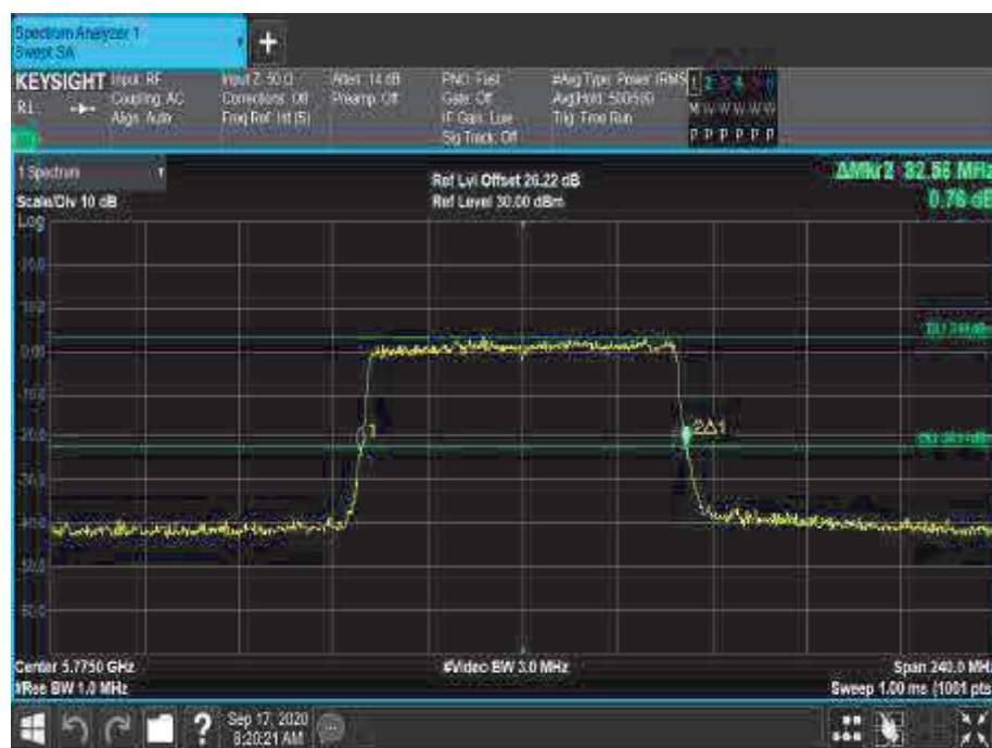
Figure 698 - 5775 MHz - 26 dB Emission Bandwidth
