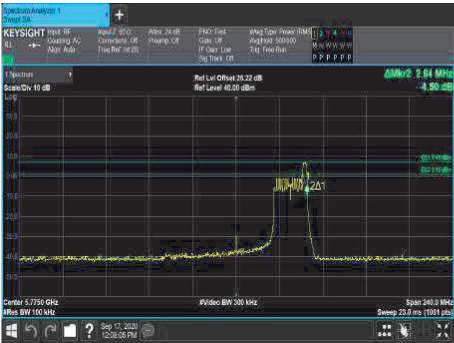
Figure 703 - 5775 MHz - 6 dB DTS Bandwidth
