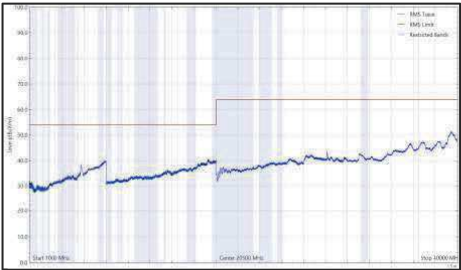
Figure 946 - U-NII-3 - 5745 MHz (CH149), HT20, CDD, Core 0 + Core 1, 1 GHz to 40 GHz, Horizontal (RMS)
