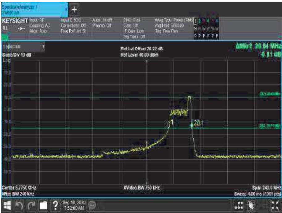
Figure 728 - 5775 MHz - 26 dB Emission Bandwidth
