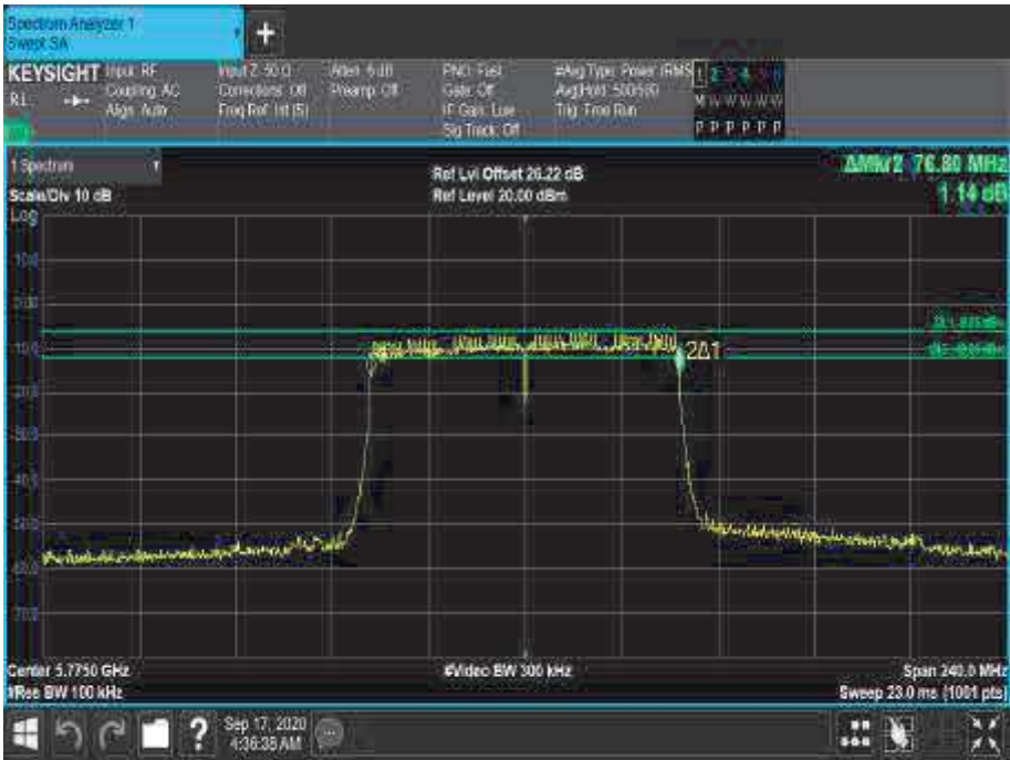
Figure 673 - 5775 MHz - 6 dB DTS Bandwidth
