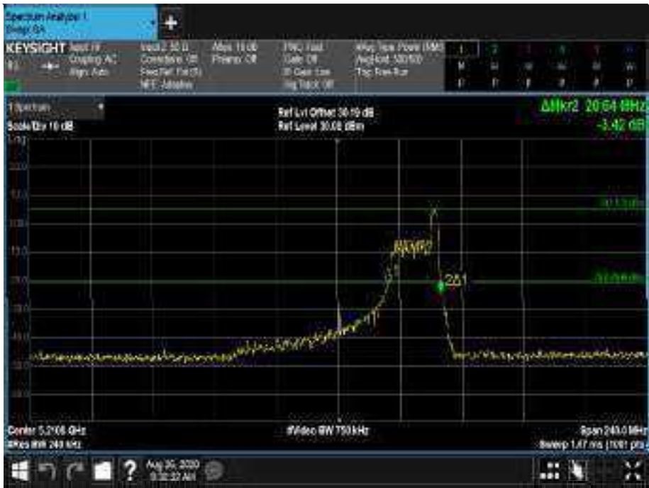
Figure299 - 5210 MHz - 26 dB Emission Bandwidth
