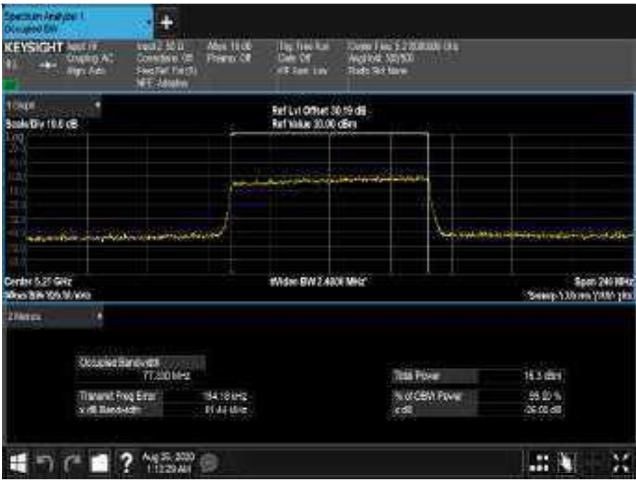
Figure314 - 5210 MHz - 99% Occupied Bandwidth
