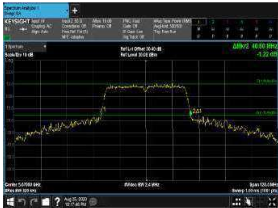
Figure 483 - 5670 MHz - 26 dB Emission Bandwidth
