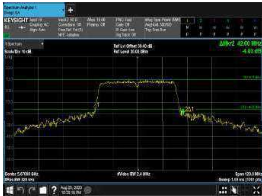
Figure 491 - 5670 MHz - 26 dB Emission Bandwidth
