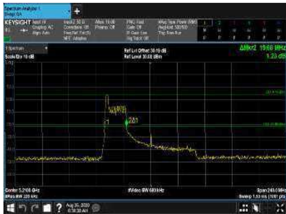
Figure 295 - 5210 MHz - 26 dB Emission Bandwidth
