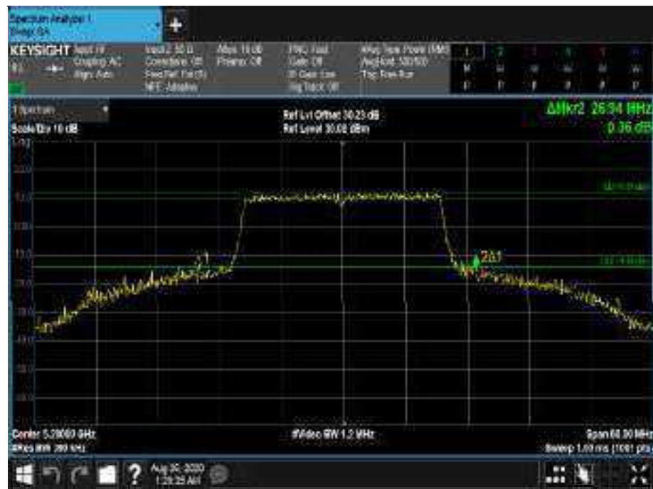
Figure 357 - 5280 MHz - 26 dB Emission Bandwidth
