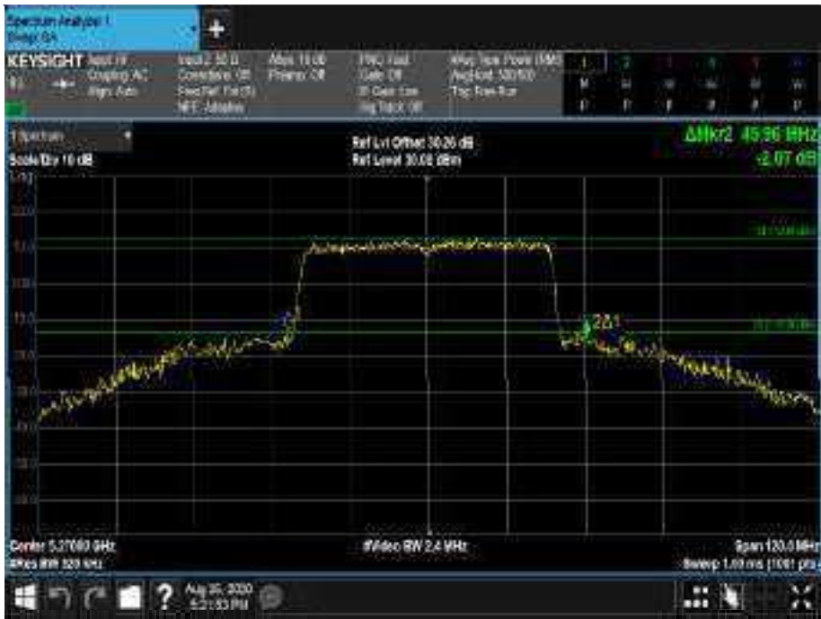
Figure397 - 5270 MHz - 26 dB Emission Bandwidth
