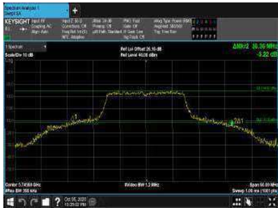
Figure 593 - 5745 MHz - 26 dB Emission Bandwidth
