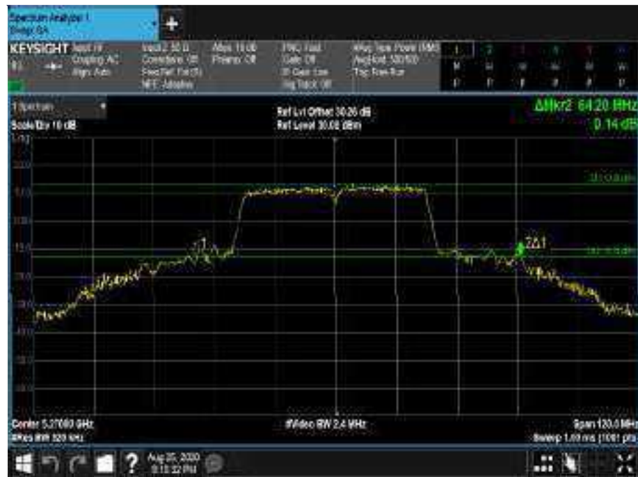
Figure373 - 5270 MHz - 26 dB Emission Bandwidth
