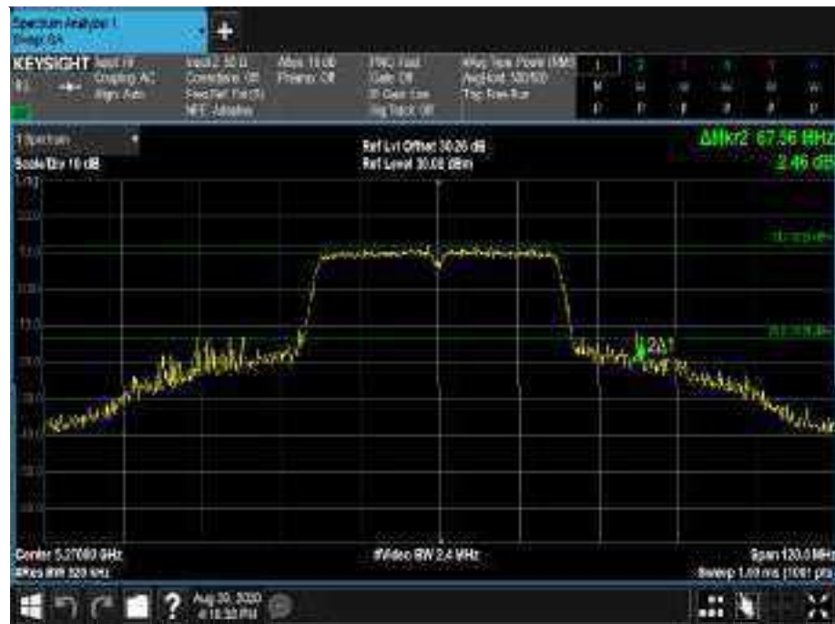
Figure385 - 5270 MHz - 26 dB Emission Bandwidth
