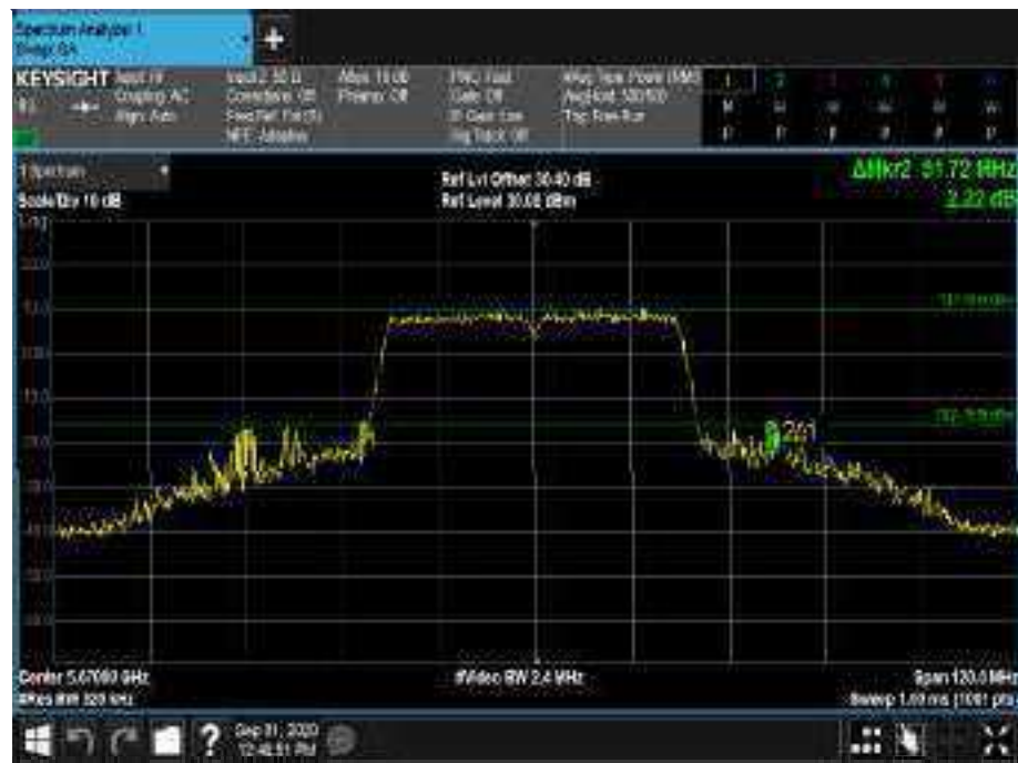
Figure507 - 5670 MHz - 26 dB Emission Bandwidth
