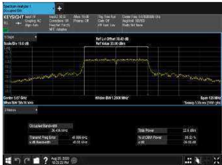
Figure 500 - 5670 MHz - 99% Occupied Bandwidth
