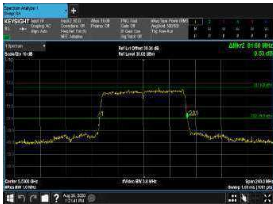
Figure547 - 5530 MHz - 26 dB Emission Bandwidth
