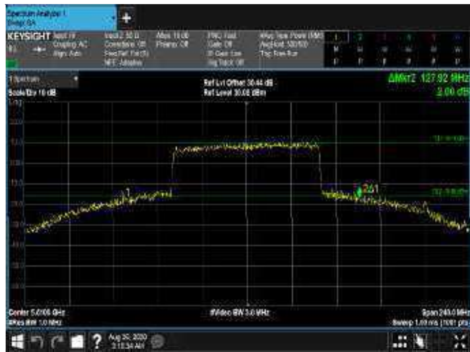
Figure573 - 5610 MHz - 26 dB Emission Bandwidth
