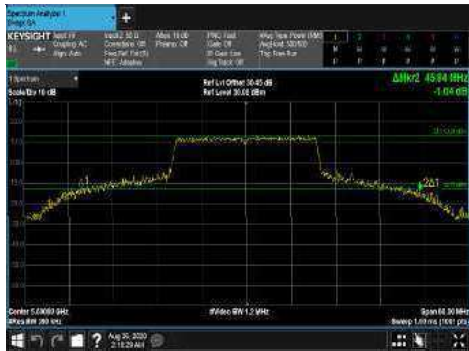
Figure 457 - 5600 MHz - 26 dB Emission Bandwidth
