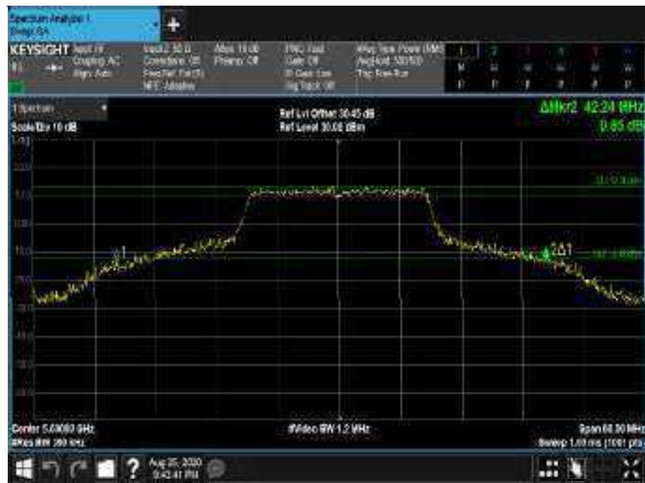
Figure 425 - 5600 MHz - 26 dB Emission Bandwidth
