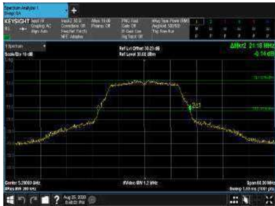
Figure 327 - 5280 MHz - 26 dB Emission Bandwidth
