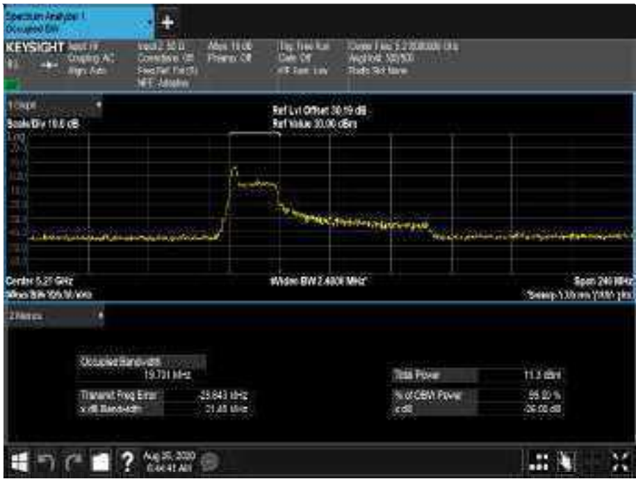
Figure320 - 5210 MHz - 99% Occupied Bandwidth
