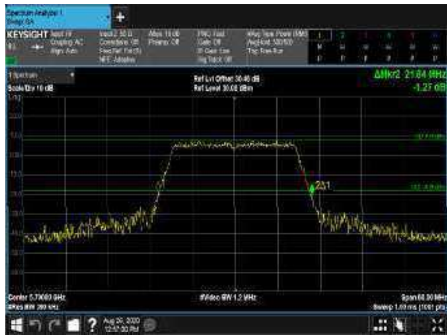
Figure 435 - 5700 MHz - 26 dB Emission Bandwidth
