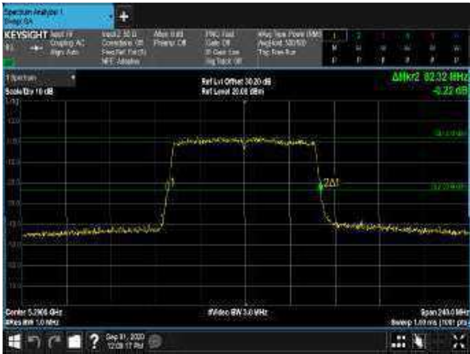
Figure 407 - 5290 MHz - 26 dB Emission Bandwidth
