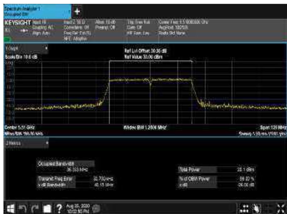
Figure 480 - 5510 MHz - 99% Occupied Bandwidth
