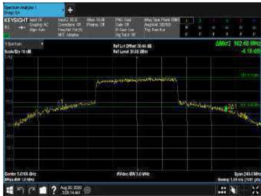
Figure561 - 5610 MHz - 26 dB Emission Bandwidth
