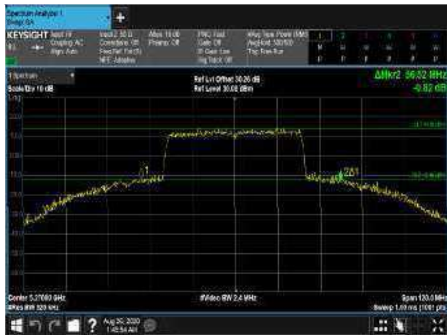
Figure389 - 5270 MHz - 26 dB Emission Bandwidth
