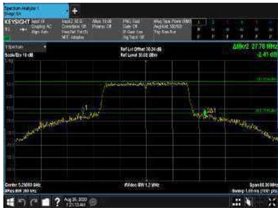
Figure 355 - 5260 MHz - 26 dB Emission Bandwidth
