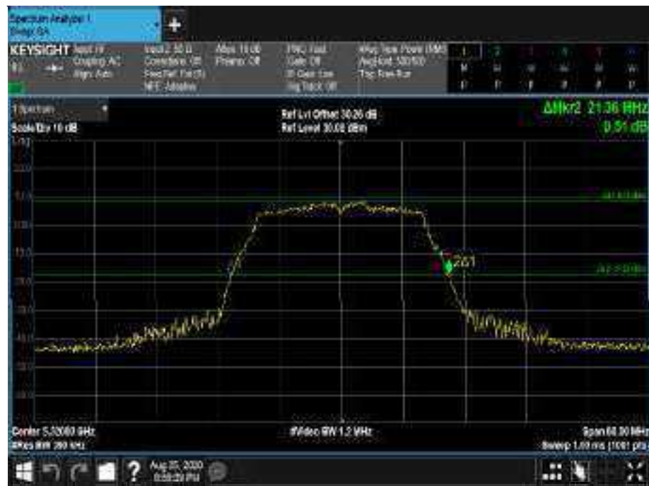
Figure 329 - 5320 MHz - 26 dB Emission Bandwidth
