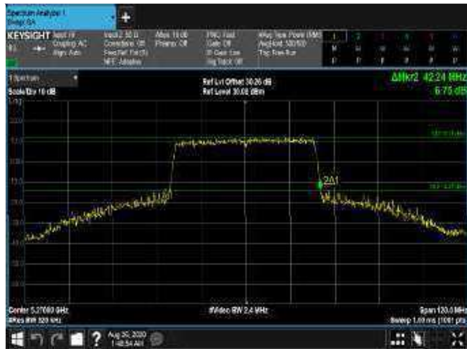
Figure 393 - 5270 MHz - 26 dB Emission Bandwidth
