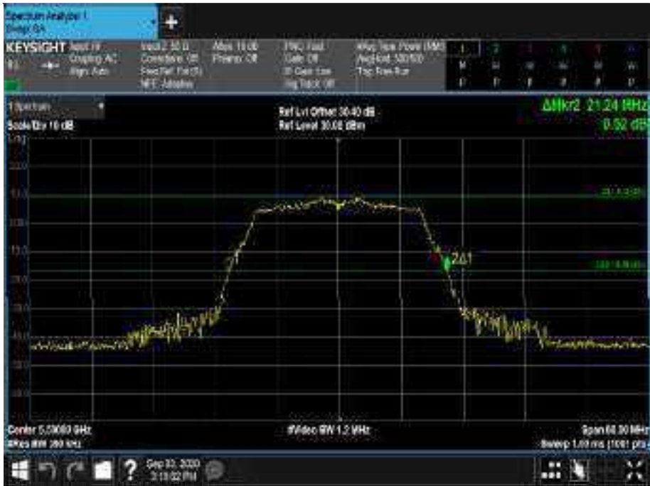
Figure 415 - 5500 MHz - 26 dB Emission Bandwidth
