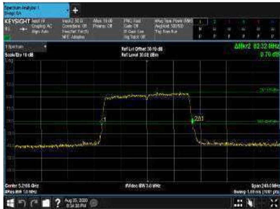
Figure283 - 5210 MHz - 26 dB Emission Bandwidth
