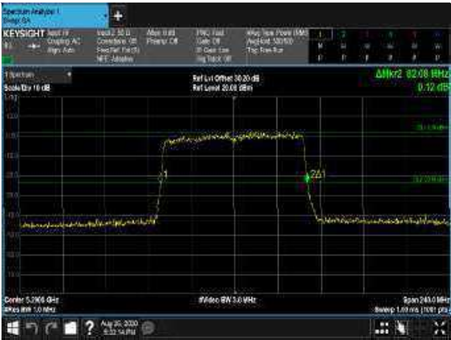
Figure 413 - 5290 MHz - 26 dB Emission Bandwidth
