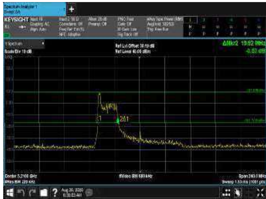
Figure 293 - 5210 MHz - 26 dB Emission Bandwidth
