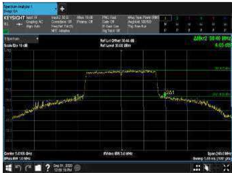
Figure 555 - 5610 MHz - 26 dB Emission Bandwidth
