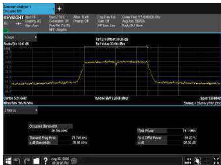
Figure 496 - 5510 MHz - 99% Occupied Bandwidth
