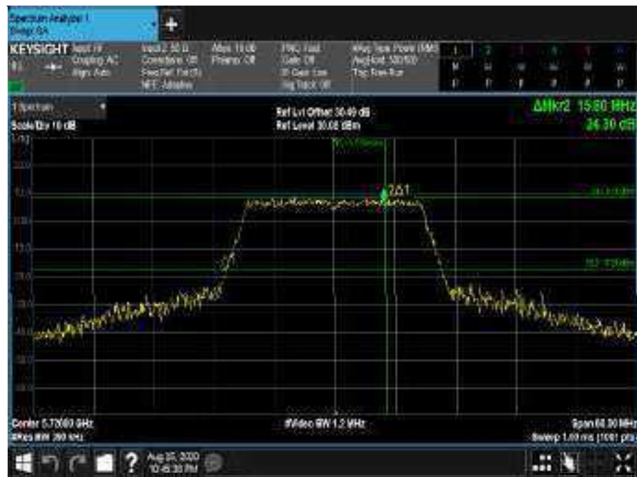
Figure 437 - 5720 MHz - 26 dB Emission Bandwidth
