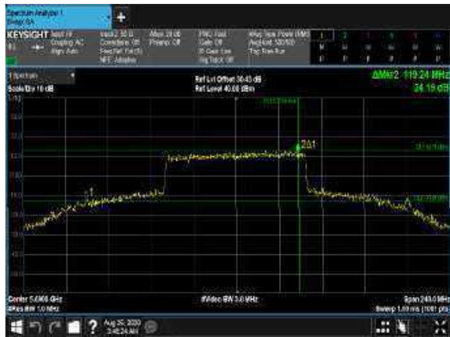
Figure575 - 5690 MHz - 26 dB Emission Bandwidth
