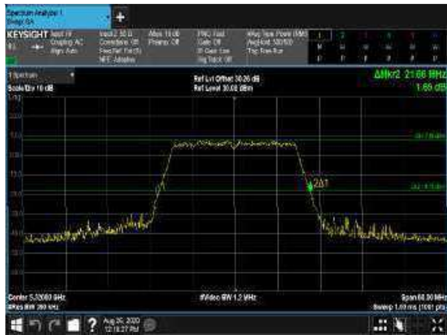
Figure 341 - 5320 MHz - 26 dB Emission Bandwidth
