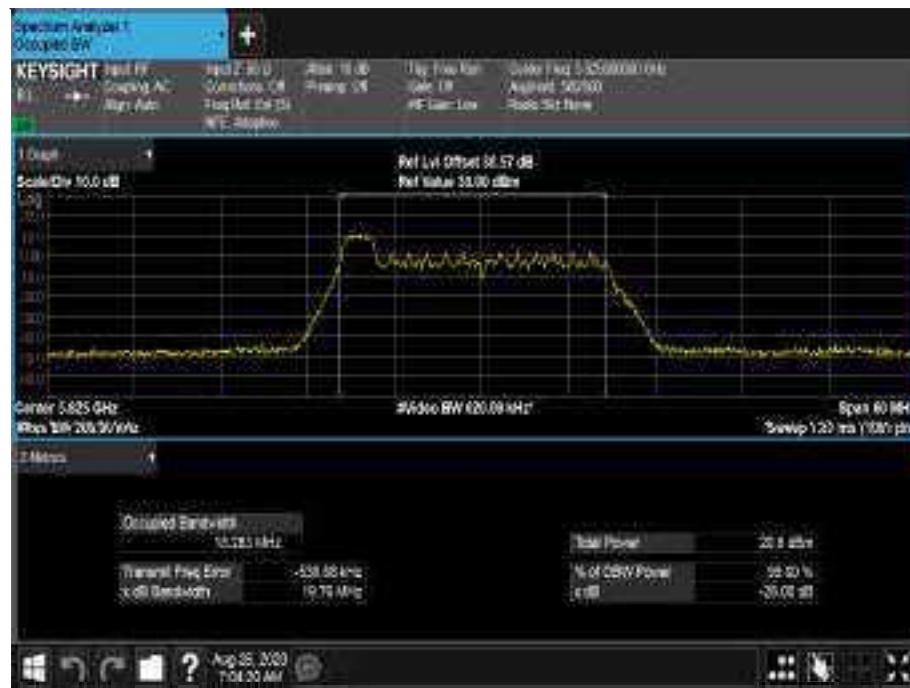
Figure 705 - 5825 MHz - 99% Occupied Bandwidth
