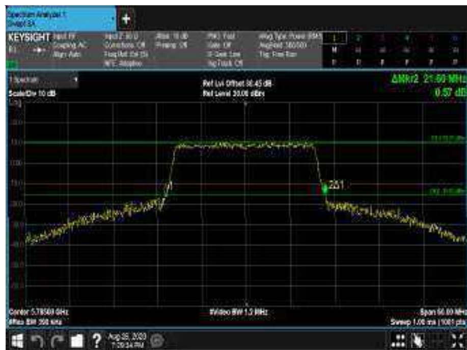
Figure692 - 5785 MHz - 26 dB Emission Bandwidth
