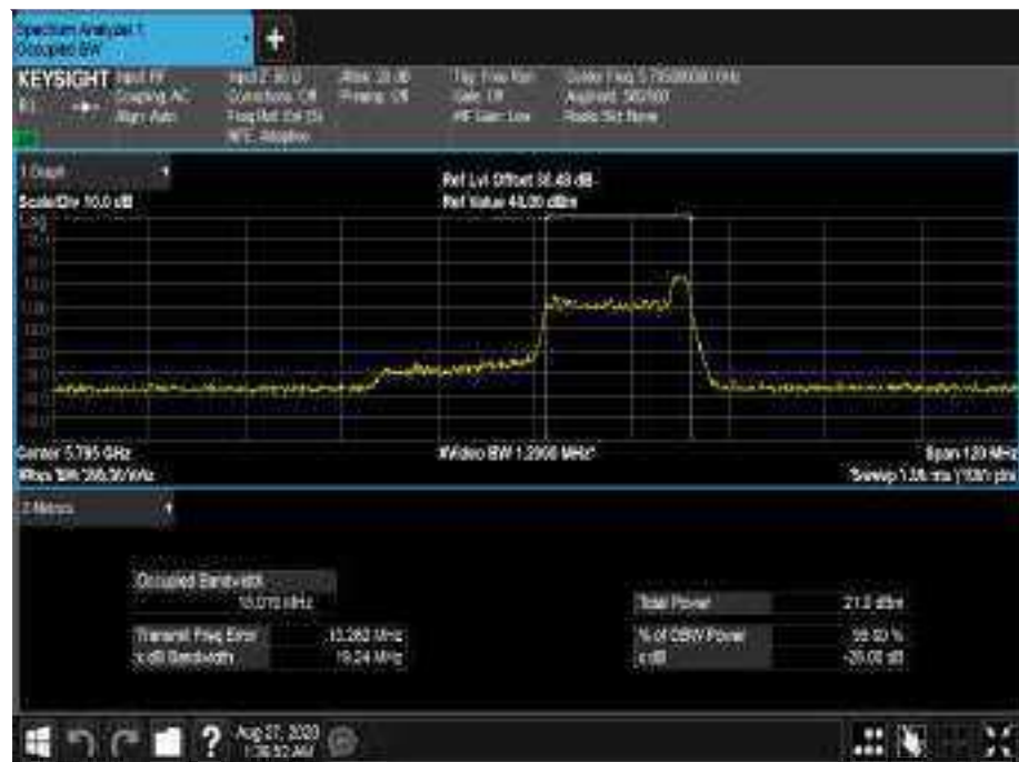
Figure 771 - 5795 MHz - 99% Occupied Bandwidth
