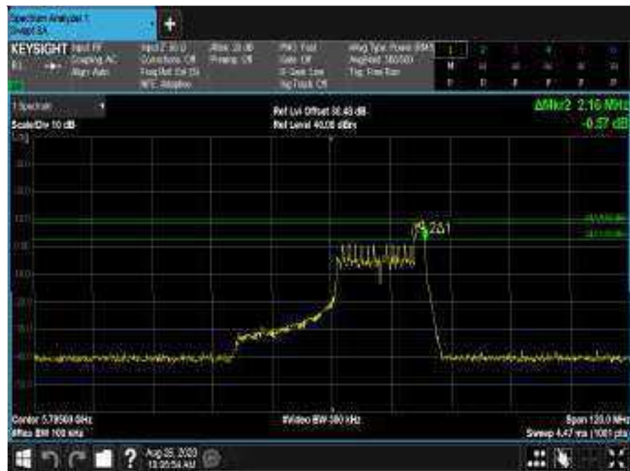
Figure 790 - 5795 MHz - 6 dB DTS Bandwidth
