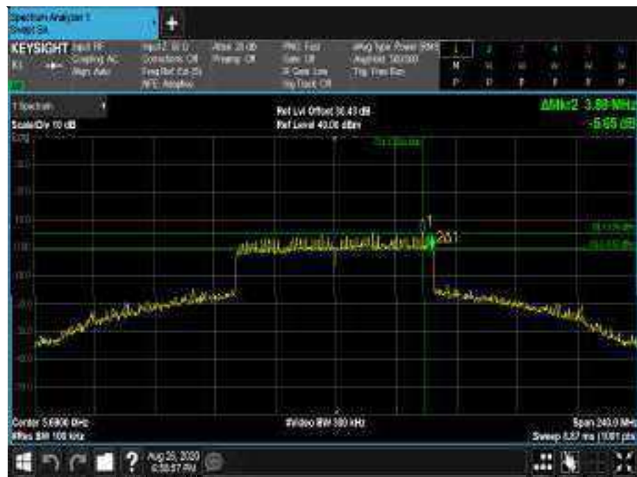
Figure838 - 5690 MHz - 6 dB DTS Bandwidth
