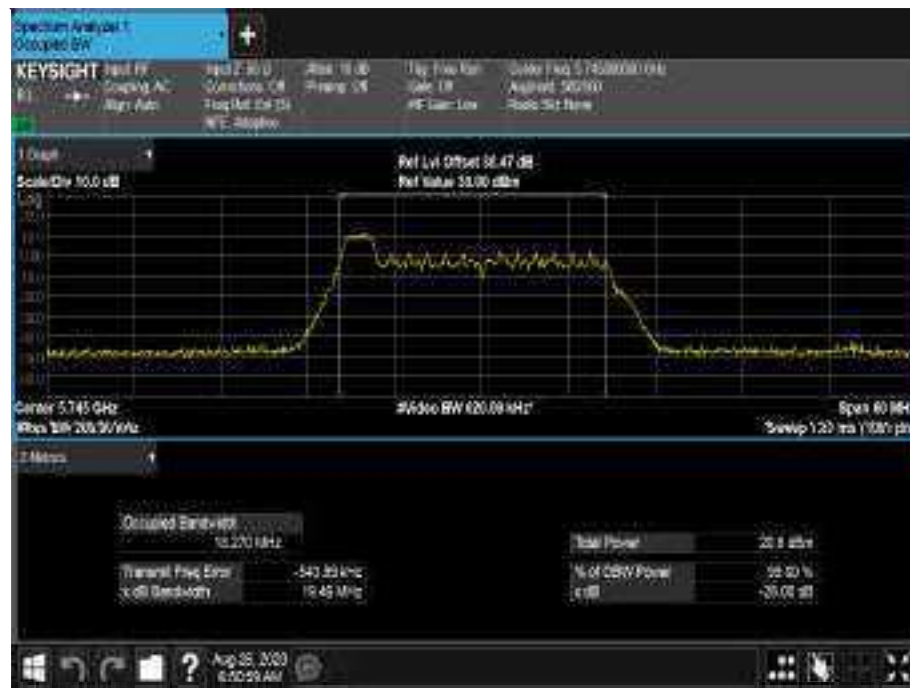
Figure 699 - 5745 MHz - 99% Occupied Bandwidth
