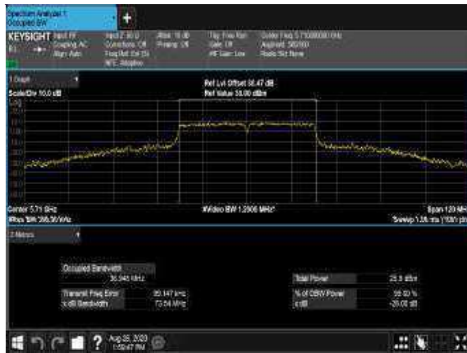
Figure 735 - 5710 MHz - 99% Occupied Bandwidth
