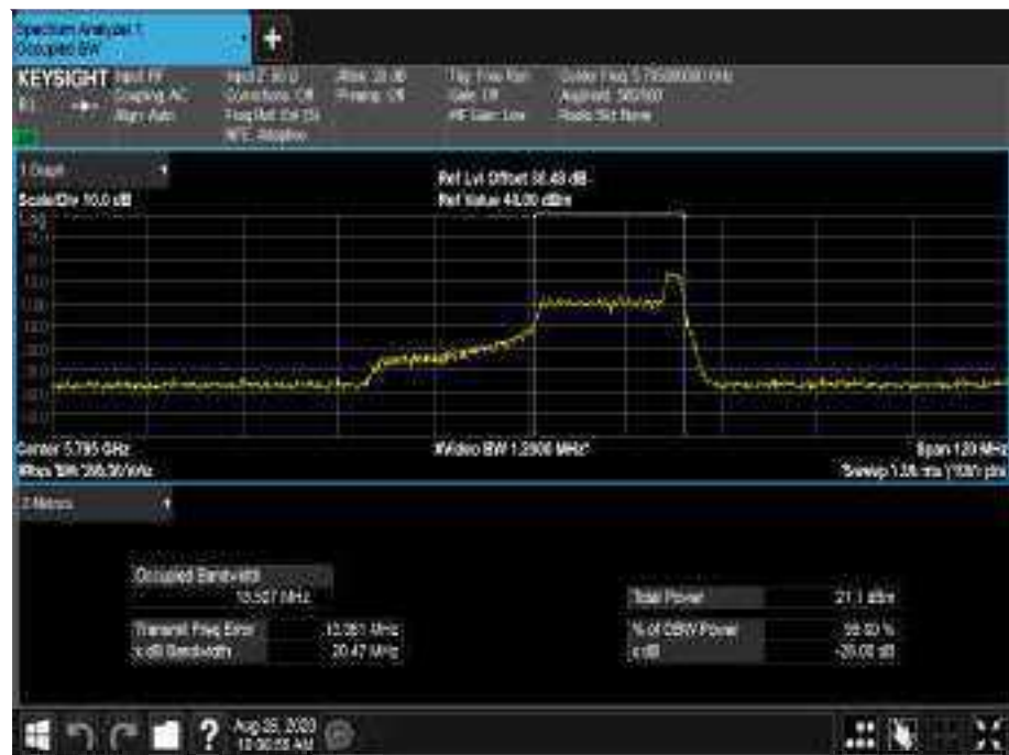
Figure 792 - 5795 MHz - 99% Occupied Bandwidth
