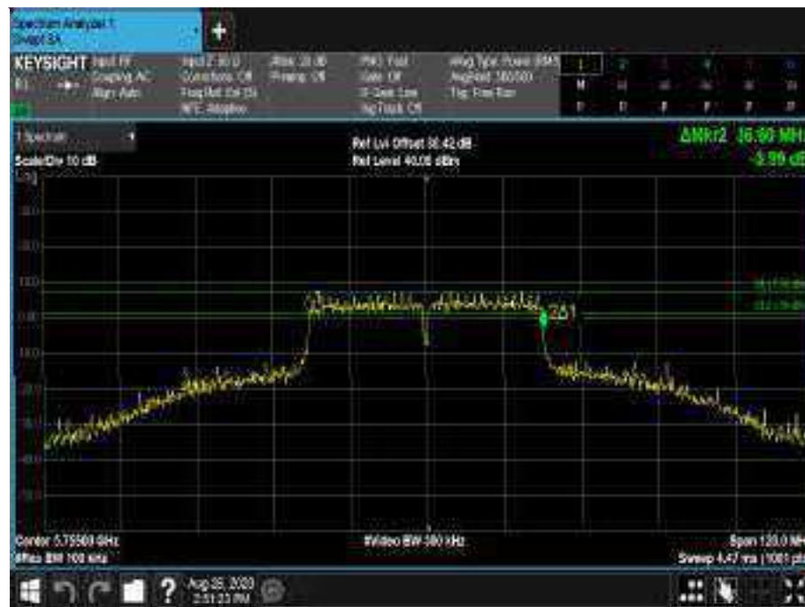
Figure 718 - 5755 MHz - 6 dB DTS Bandwidth
