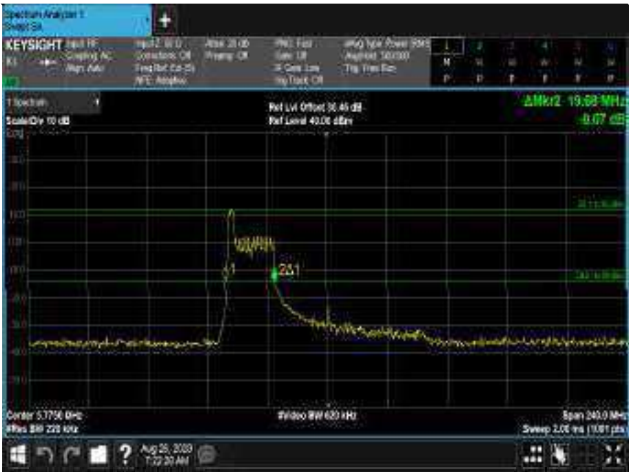
Figure857 - 5775 MHz - 26 dB Emission Bandwidth
