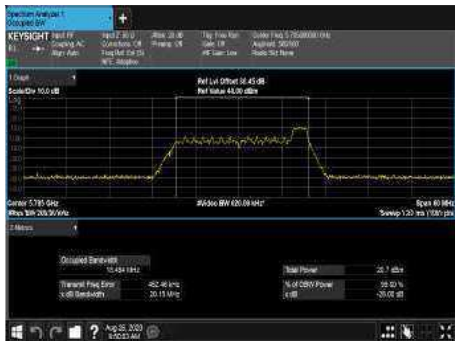
Figure 711 - 5785 MHz - 99% Occupied Bandwidth
