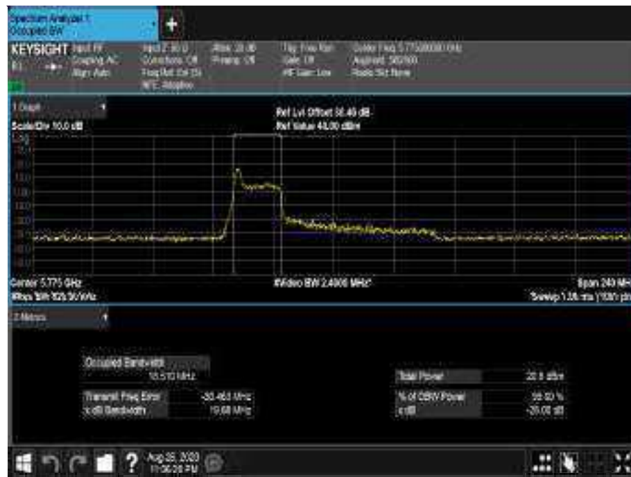
Figure846 - 5775 MHz - 99% Occupied Bandwidth
