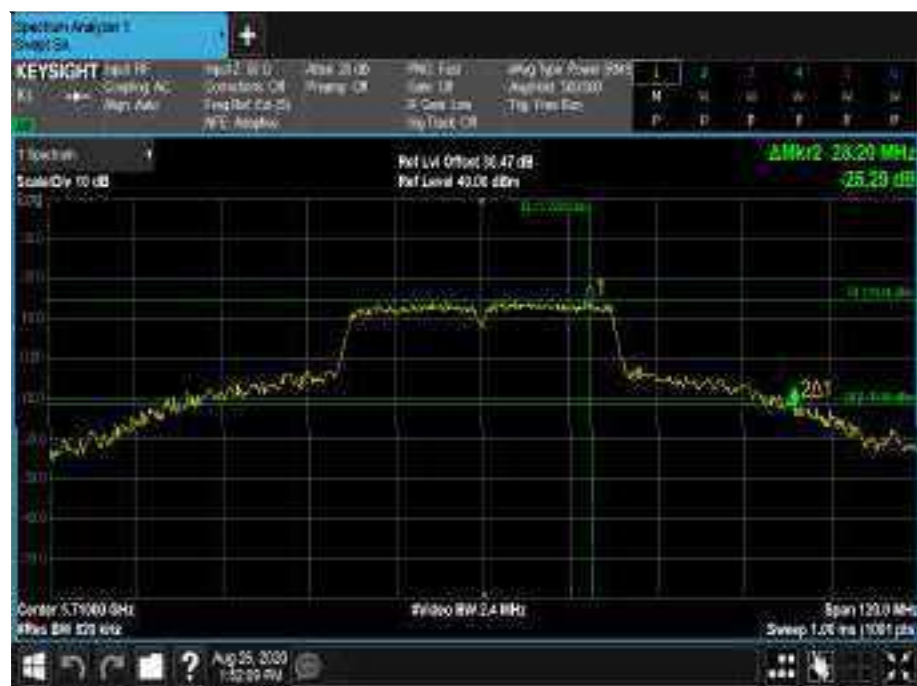
Figure 716 - 5710 MHz - 26 dB Emission Bandwidth
