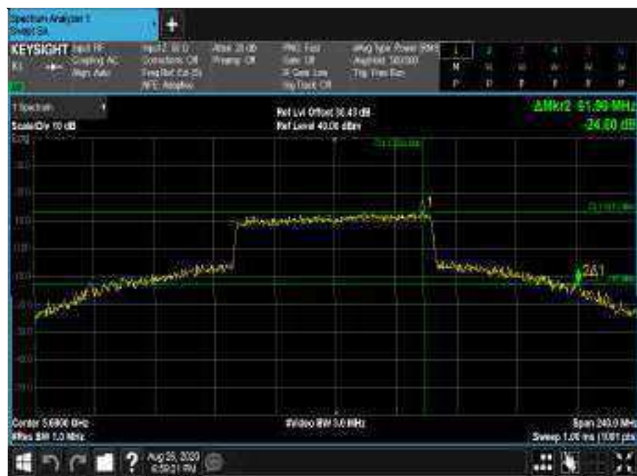
Figure839 - 5690 MHz - 26 dB Emission Bandwidth
