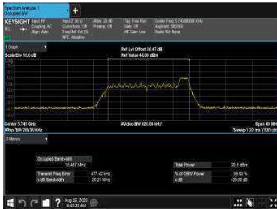
Figure 708 - 5745 MHz - 99% Occupied Bandwidth
