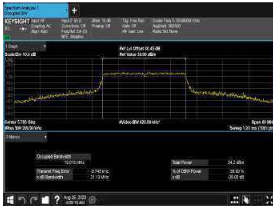
Figure693 - 5785 MHz - 99% Occupied Bandwidth
