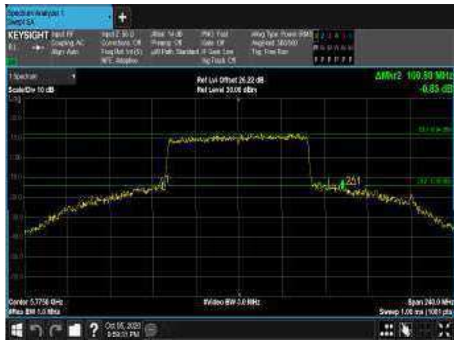
Figure866 - 5775 MHz - 26 dB Emission Bandwidth
