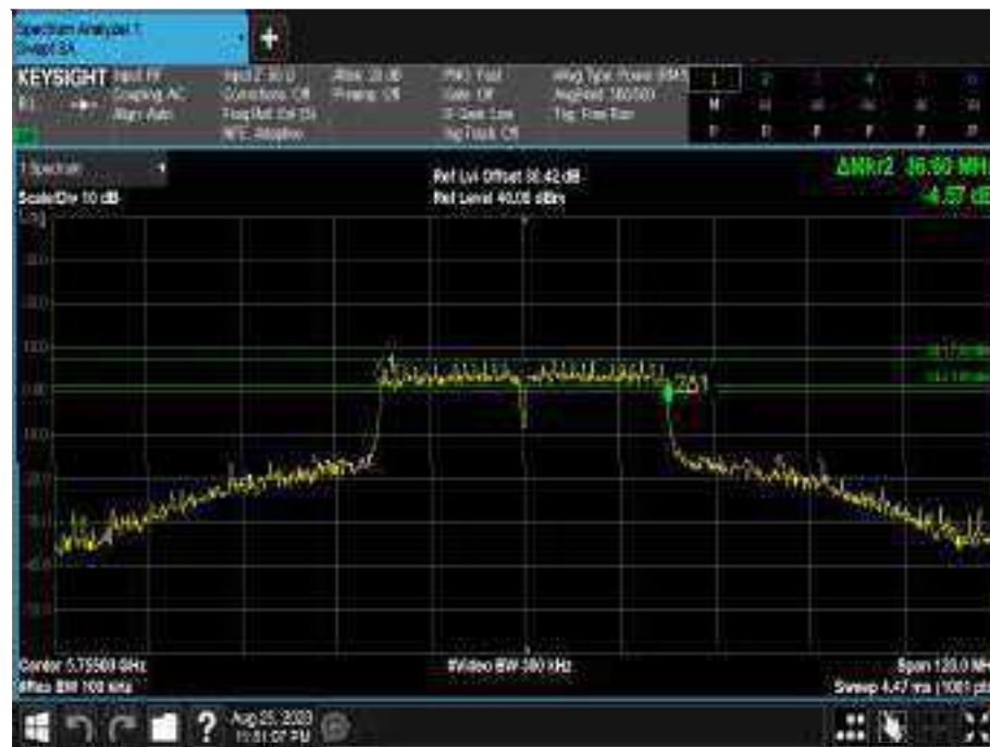
Figure 736 - 5755 MHz - 6 dB DTS Bandwidth
