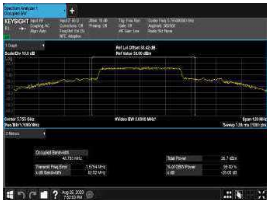
Figure 798 - 5755 MHz - 99% Occupied Bandwidth
