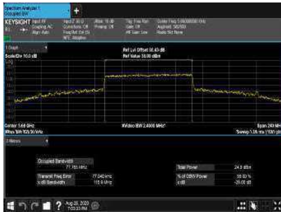
Figure852 - 5690 MHz - 99% Occupied Bandwidth
