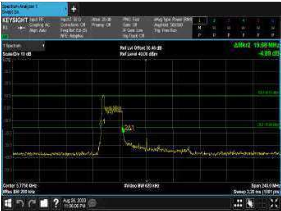
Figure845 - 5775 MHz - 26 dB Emission Bandwidth
