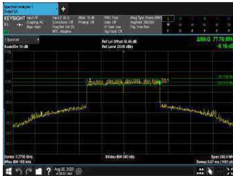
Figure865 - 5775 MHz - 6 dB DTS Bandwidth
