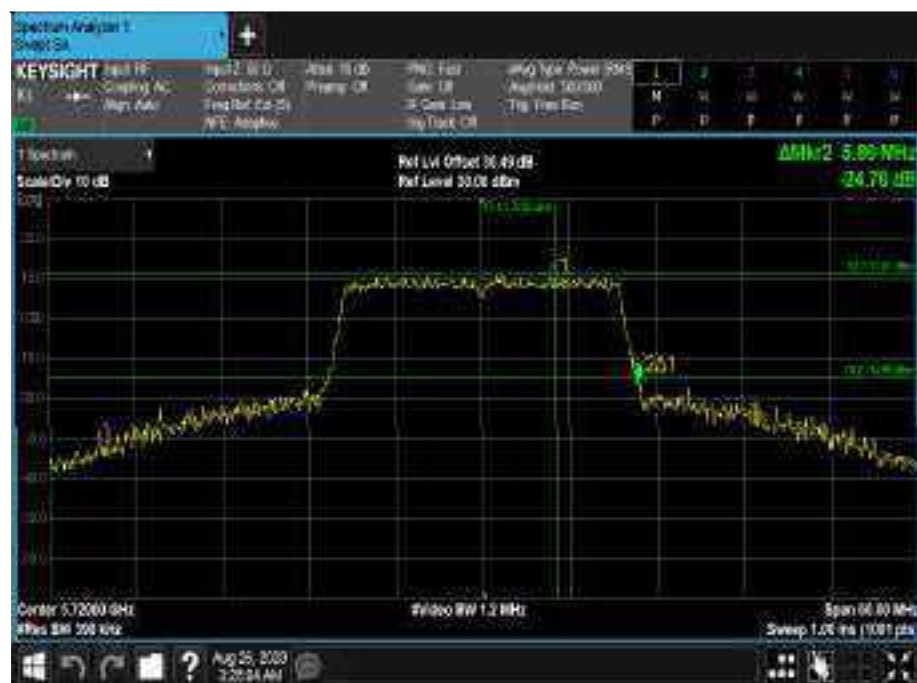
Figure 686 - 5720 MHz - 26 dB Emission Bandwidth
