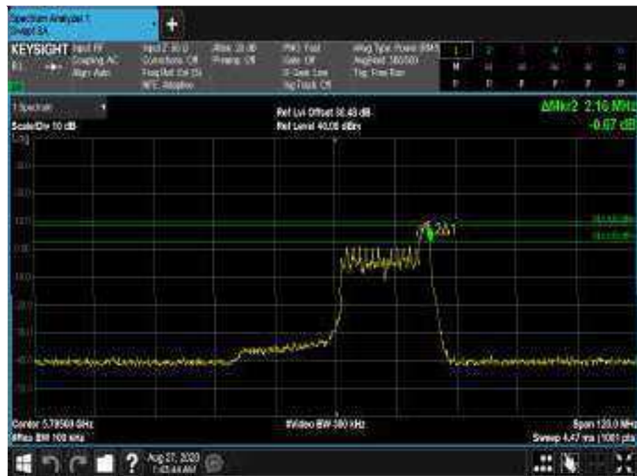
Figure811 - 5795 MHz - 6 dB DTS Bandwidth
