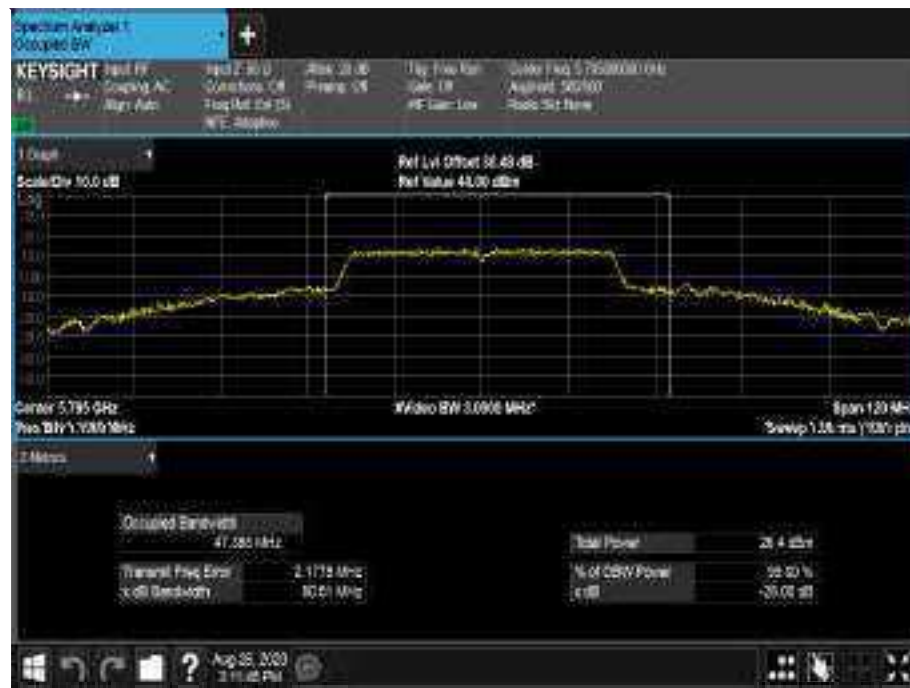
Figure 741 - 5795 MHz - 99% Occupied Bandwidth
