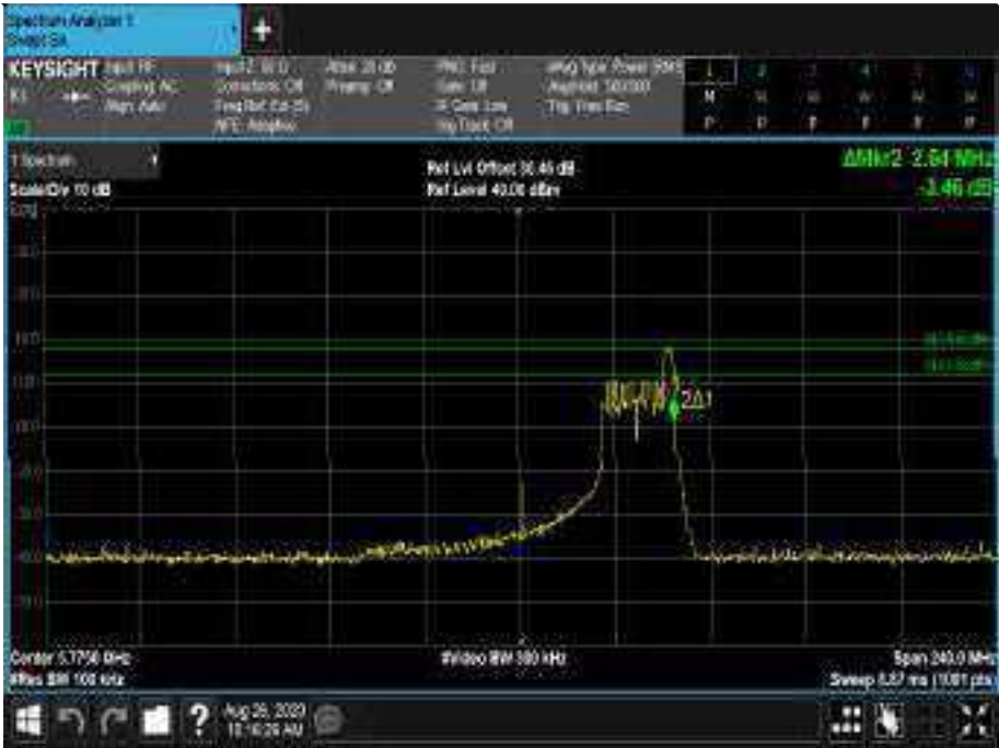
Figure871 - 5775 MHz - 6 dB DTS Bandwidth
