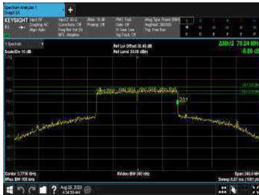
Figure853 - 5775 MHz - 6 dB DTS Bandwidth
