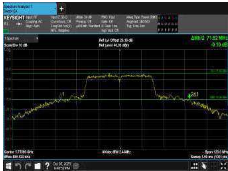
Figure 737 - 5755 MHz - 26 dB Emission Bandwidth
