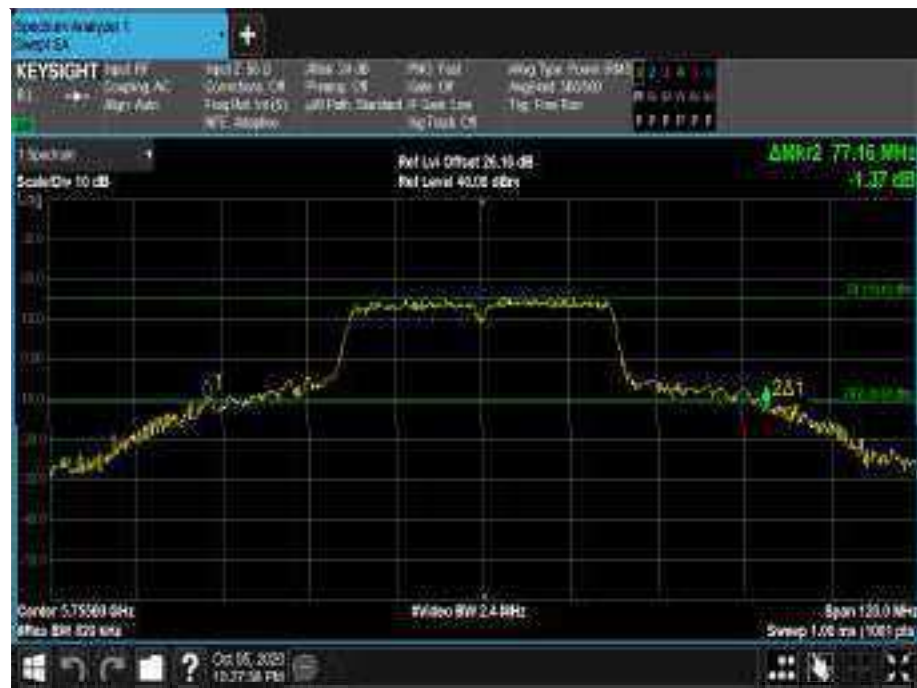
Figure 719 - 5755 MHz - 26 dB Emission Bandwidth
