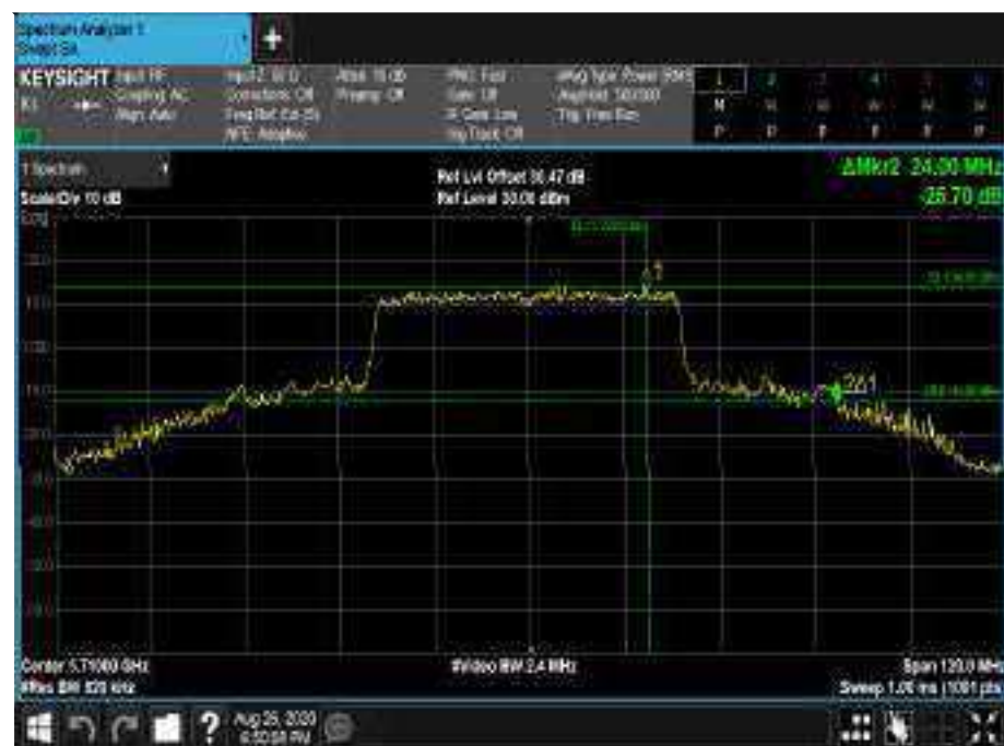
Figure 794 - 5710 MHz - 26 dB Emission Bandwidth
