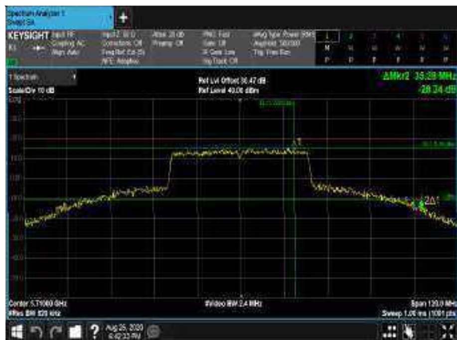
Figure 752 - 5710 MHz - 26 dB Emission Bandwidth
