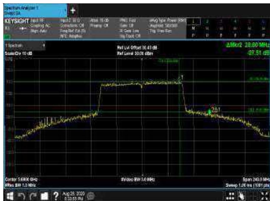
Figure833 - 5690 MHz - 26 dB Emission Bandwidth
