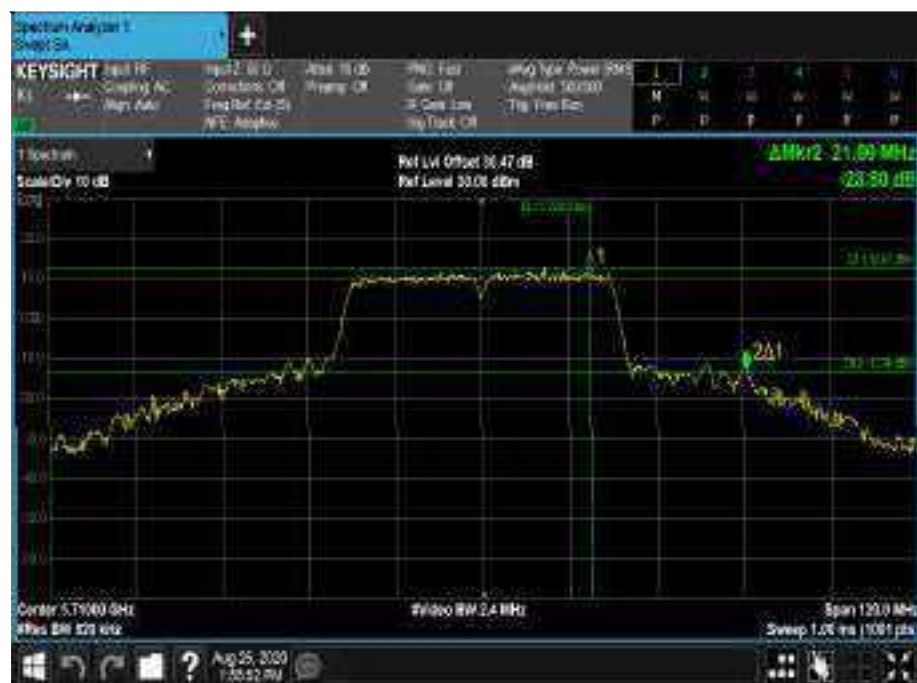
Figure 725 - 5710 MHz - 26 dB Emission Bandwidth
