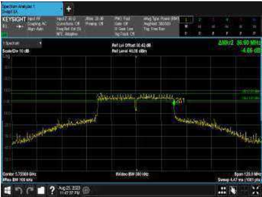
Figure 727 - 5755 MHz - 6 dB DTS Bandwidth
