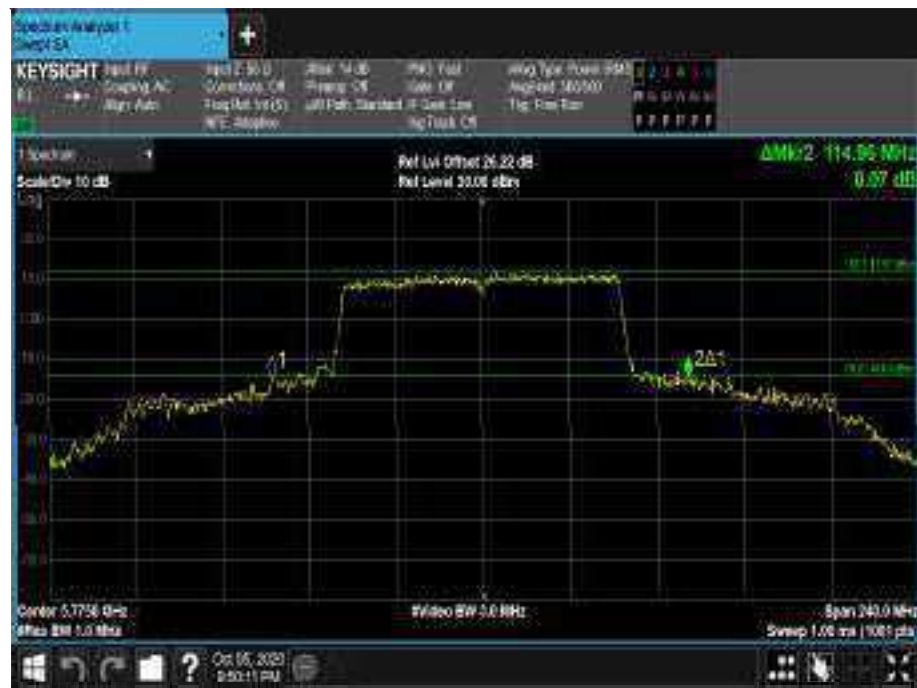
Figure824 - 5775 MHz - 26 dB Emission Bandwidth
