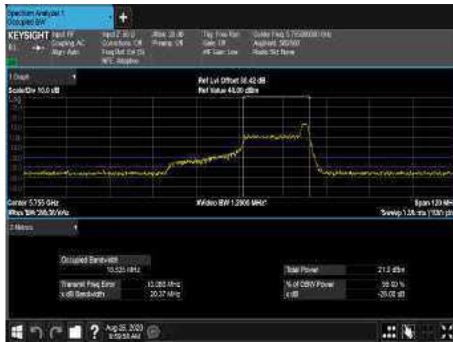
Figure 789 - 5755 MHz - 99% Occupied Bandwidth
