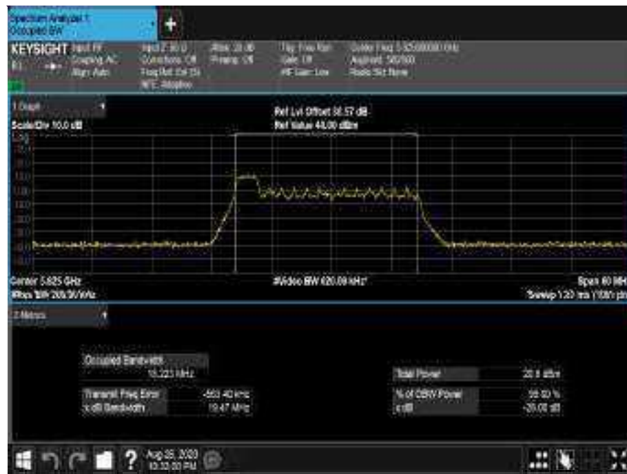
Figure 645 - 5825 MHz - 99% Occupied Bandwidth
