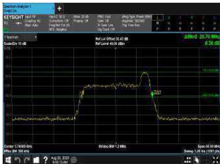
Figure 707 - 5745 MHz - 26 dB Emission Bandwidth
