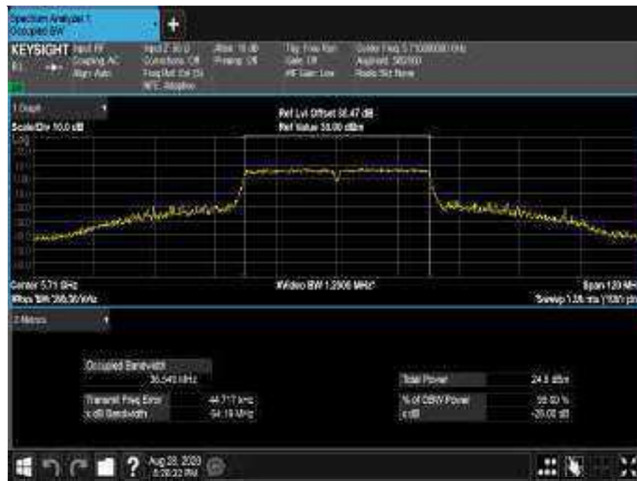
Figure 744 - 5710 MHz - 99% Occupied Bandwidth
