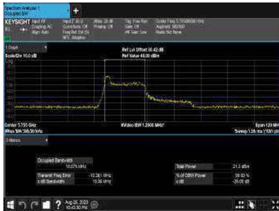
Figure 762 - 5755 MHz - 99% Occupied Bandwidth
