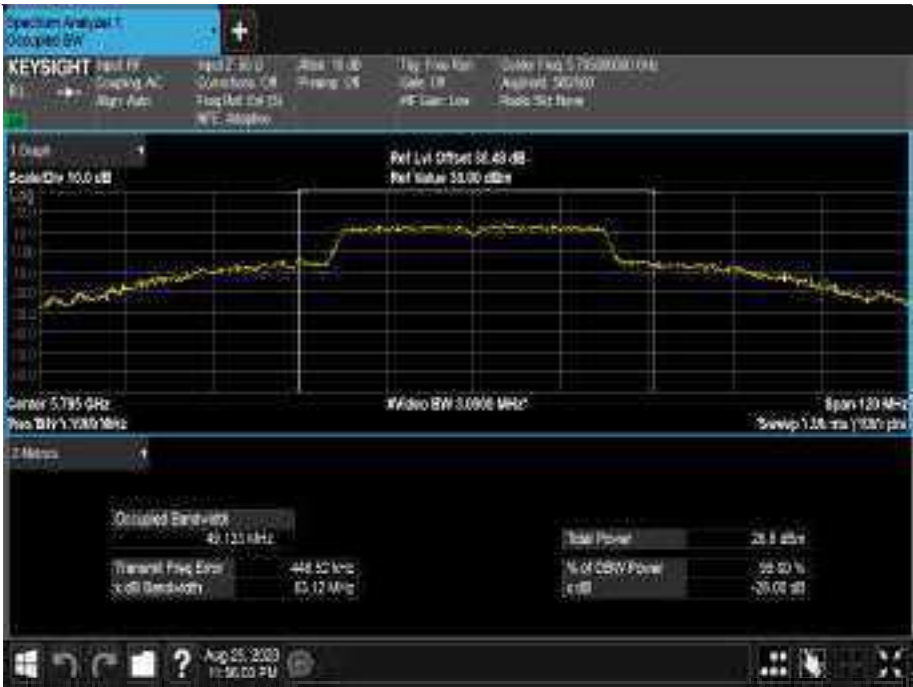
Figure 732 - 5795 MHz - 99% Occupied Bandwidth
