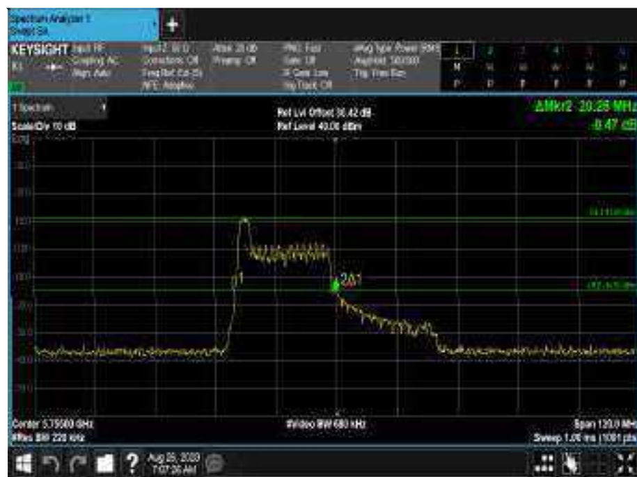
Figure 782 - 5755 MHz - 26 dB Emission Bandwidth
