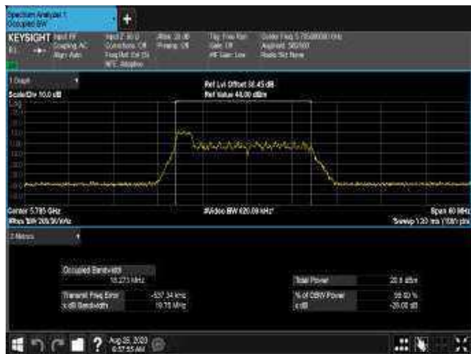
Figure 702 - 5785 MHz - 99% Occupied Bandwidth
