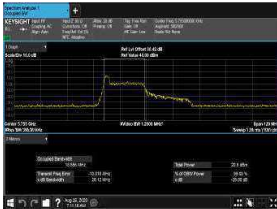
Figure804 - 5755 MHz - 99% Occupied Bandwidth
