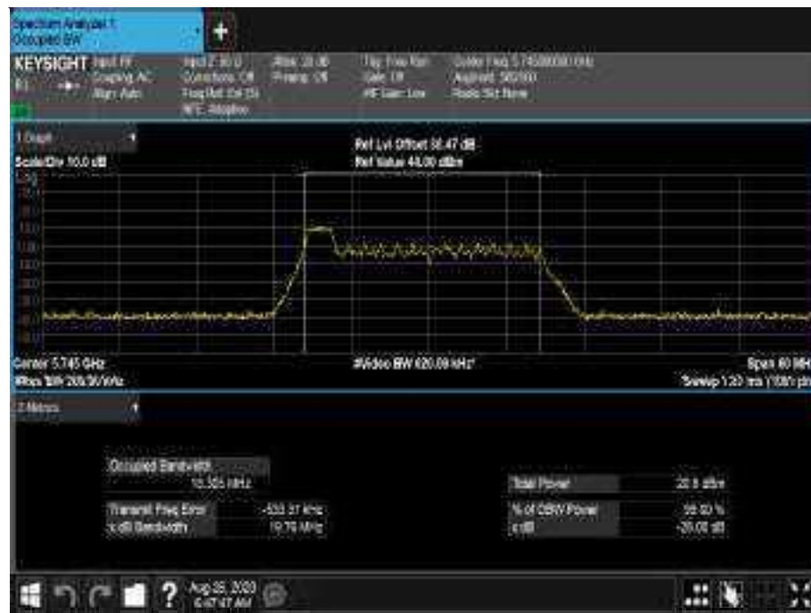
Figure669 - 5745 MHz - 99% Occupied Bandwidth
