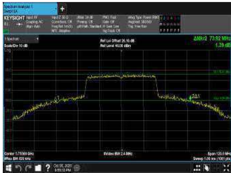
Figure 776 - 5755 MHz - 26 dB Emission Bandwidth
