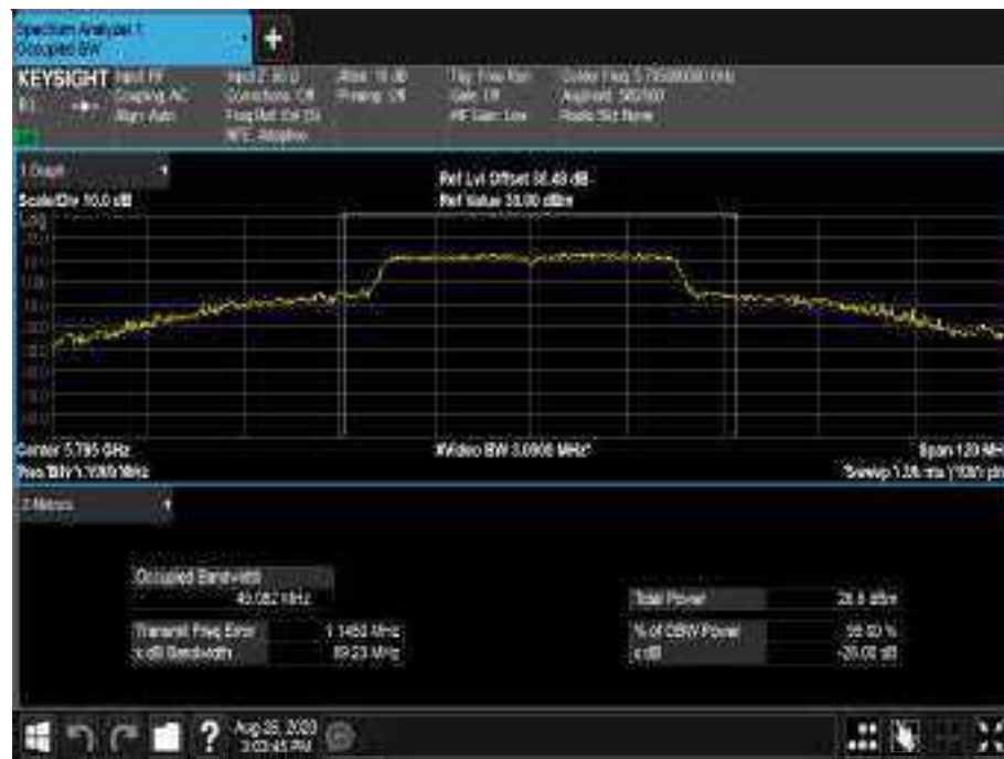
Figure 723 - 5795 MHz - 99% Occupied Bandwidth
