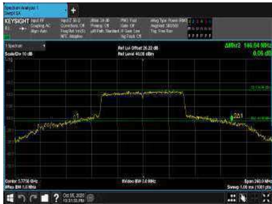
Figure 818 - 5775 MHz - 26 dB Emission Bandwidth
