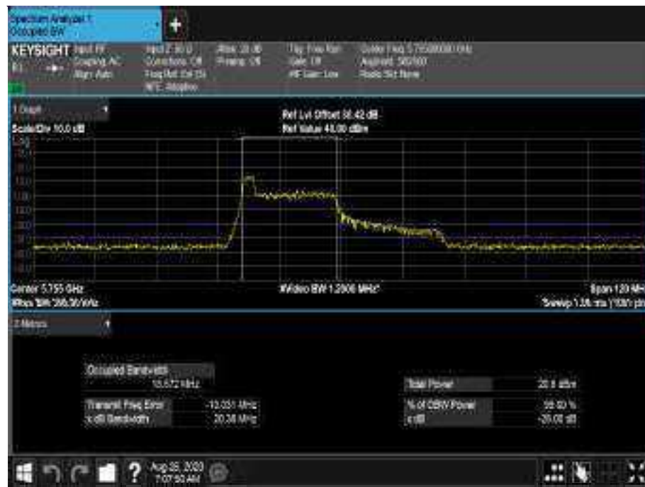
Figure 783 - 5755 MHz - 99% Occupied Bandwidth
