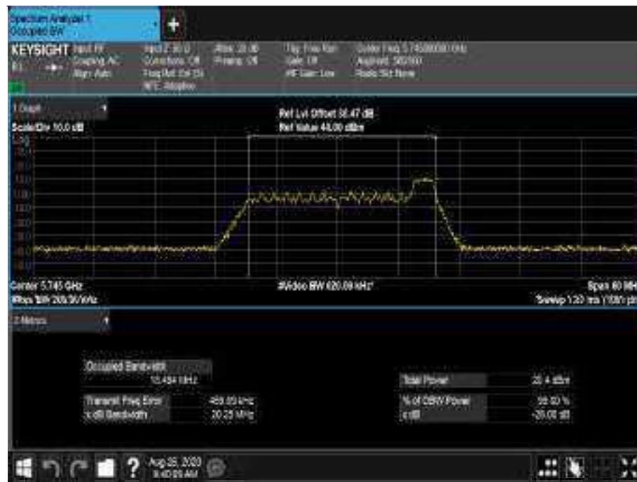
Figure678 - 5745 MHz - 99% Occupied Bandwidth
