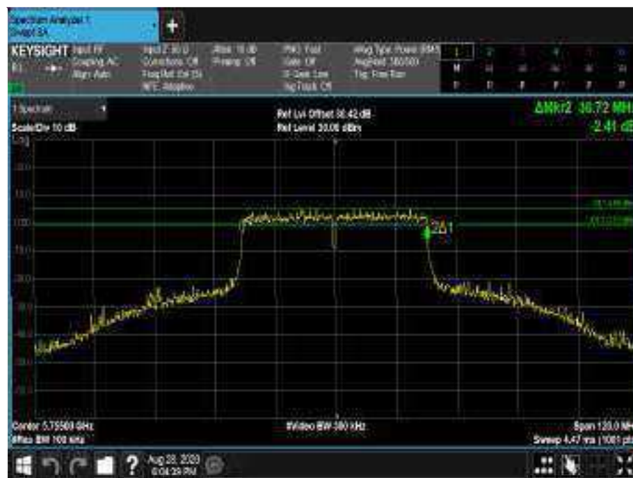
Figure 745 - 5755 MHz - 6 dB DTS Bandwidth
