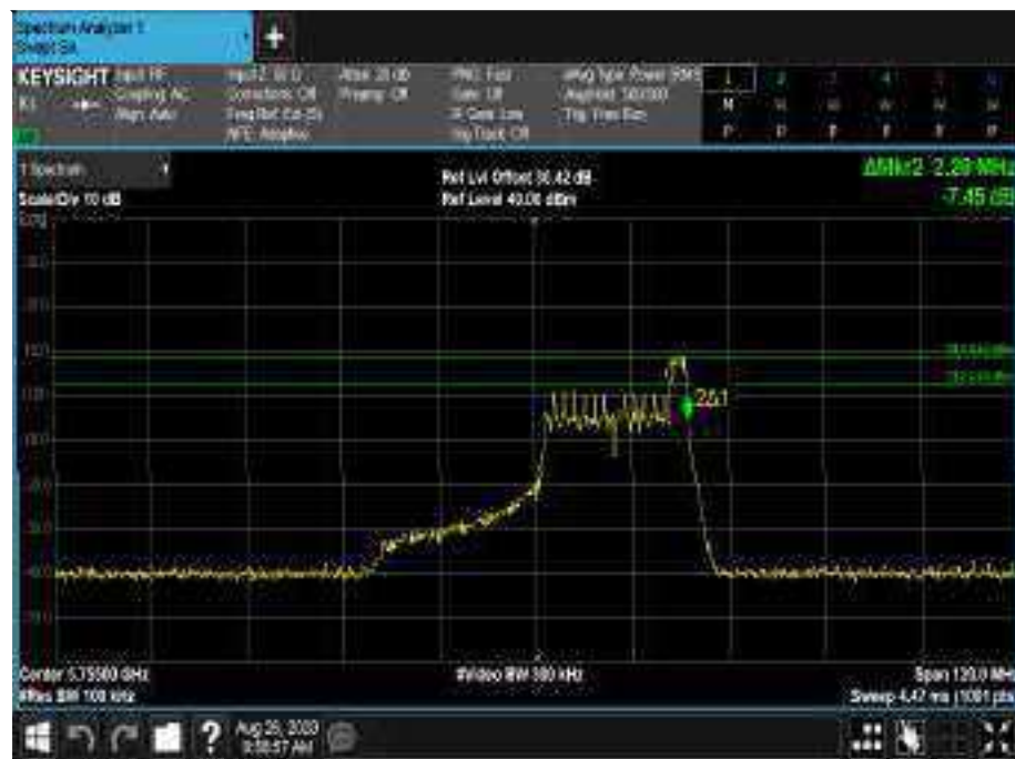
Figure 787 - 5755 MHz - 6 dB DTS Bandwidth
