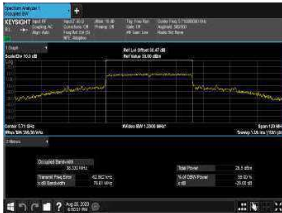
Figure795 - 5710 MHz - 99% Occupied Bandwidth
