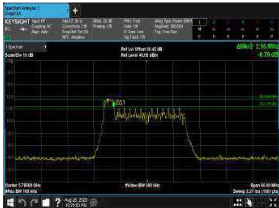
Figure670 - 5785 MHz - 6 dB DTS Bandwidth
