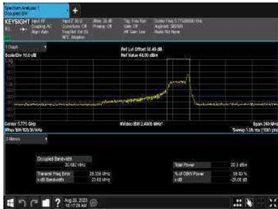
Figure873 - 5775 MHz - 99% Occupied Bandwidth
