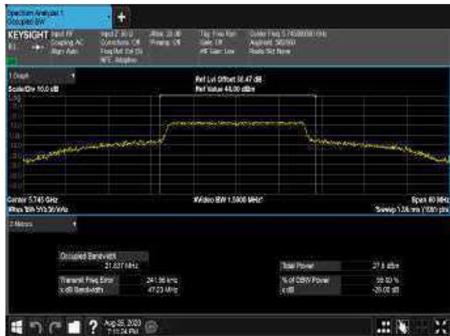
Figure 630 - 5745 MHz - 99% Occupied Bandwidth
