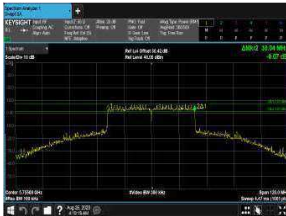
Figure775 - 5755 MHz - 6 dB DTS Bandwidth
