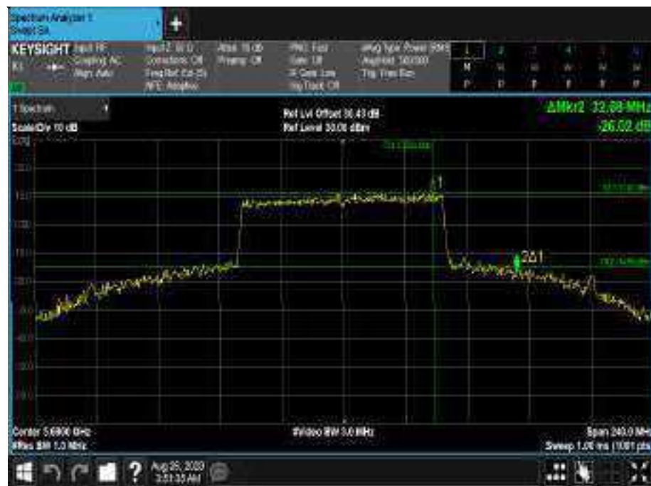
Figure 851 - 5690 MHz - 26 dB Emission Bandwidth
