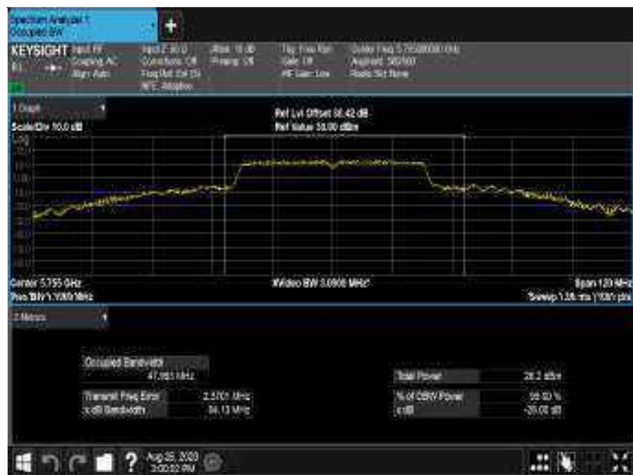
Figure 738 - 5755 MHz - 99% Occupied Bandwidth
