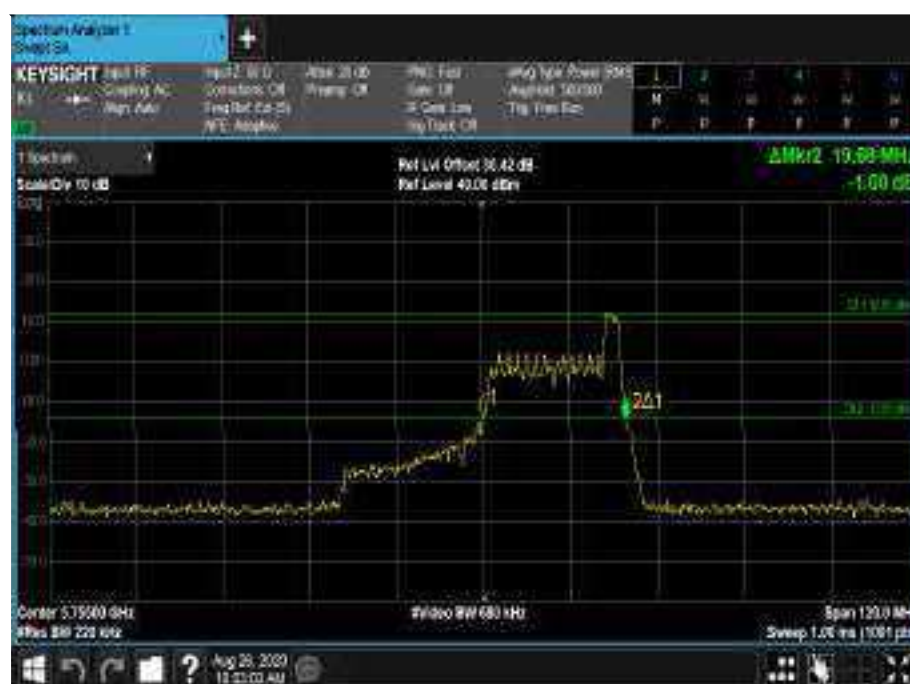
Figure 809 - 5755 MHz - 26 dB Emission Bandwidth
