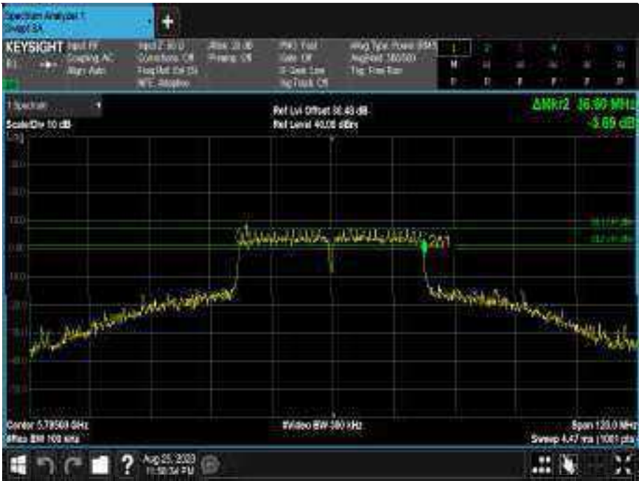
Figure 739 - 5795 MHz - 6 dB DTS Bandwidth
