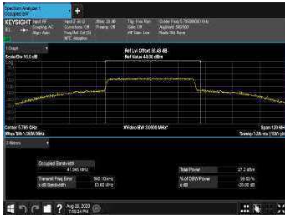
Figure 780 - 5795 MHz - 99% Occupied Bandwidth
