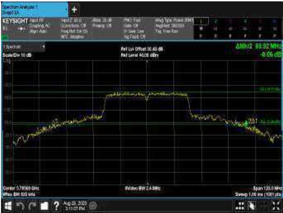
Figure 740 - 5795 MHz - 26 dB Emission Bandwidth
