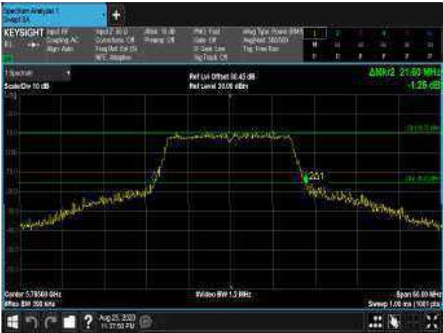
Figure608 - 5785 MHz - 26 dB Emission Bandwidth
