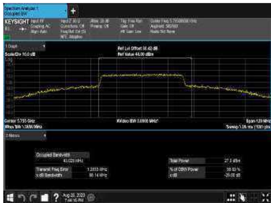
Figure 756 - 5755 MHz - 99% Occupied Bandwidth
