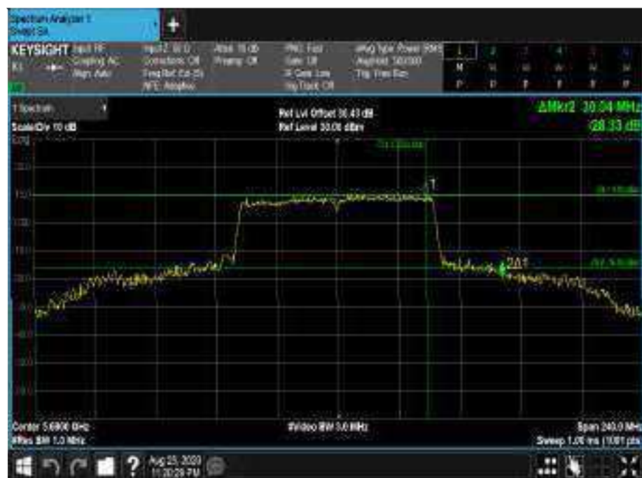
Figure 821 - 5690 MHz - 26 dB Emission Bandwidth
