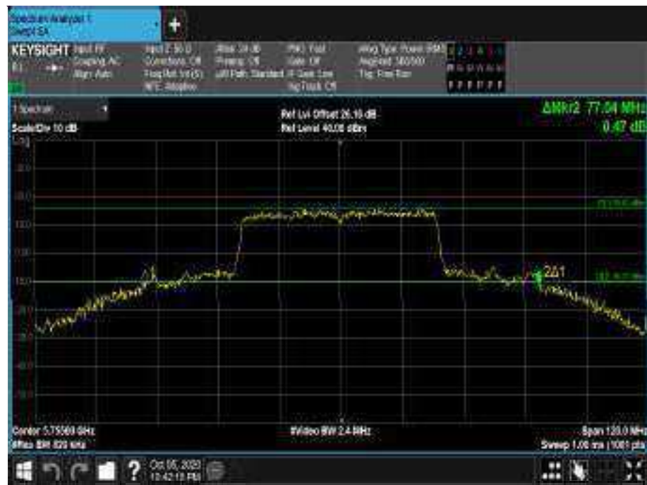
Figure 797 - 5755 MHz - 26 dB Emission Bandwidth
