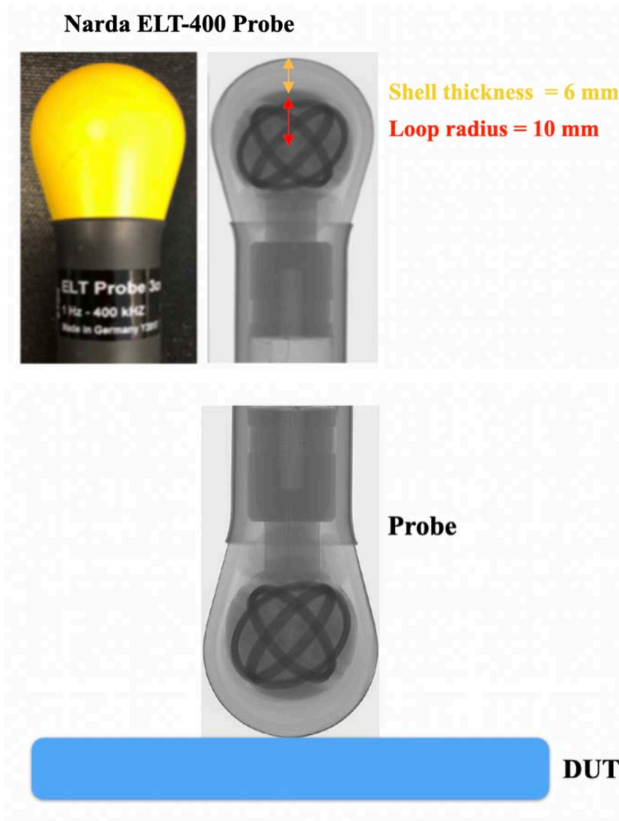
Figure 2: ELT-400 probe.
