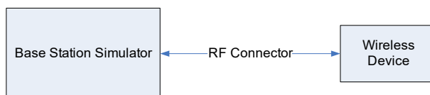
Figure 8-3 Power Measurement Setup
