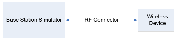
Figure 8-2 Power Measurement Setup
