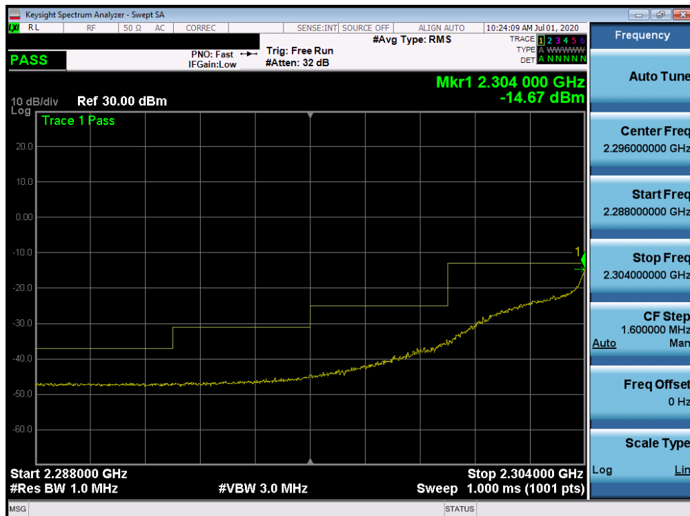
Plot 7-331. Lower Extended Band Edge Plot (Band 30 - 5.0MHz QPSK - Full RB Configuration)
