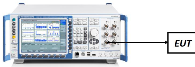
Figure 7-5. ERP/EIRP Measurement Setup
