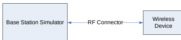
Figure 8-3 Power Measurement Setup
