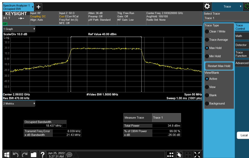
Plot 7-87. Occupied Bandwidth Plot (NR Band n41 - 20MHz CP-OFDM QPSK - Full RB)
