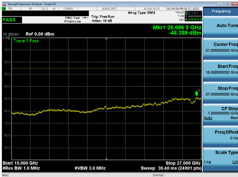
Plot 7-153. Conducted Spurious Plot (LTE Band 7 - 20MHz QPSK - RB Size 1, RB Offset 0 - Mid Channel)
