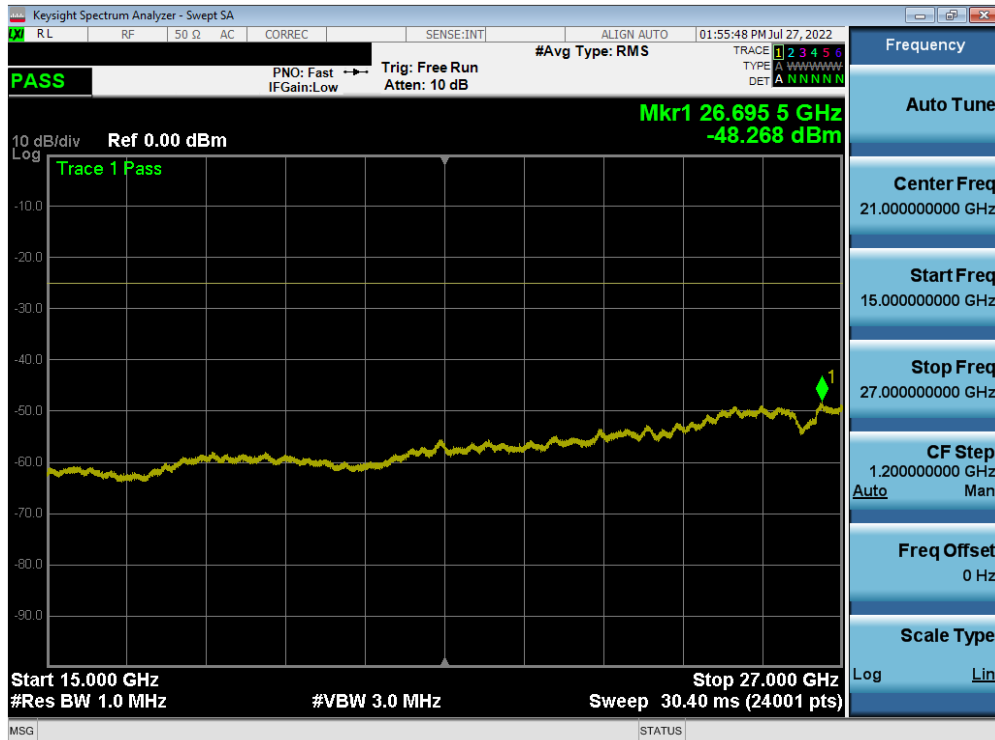
Plot 7-150. Conducted Spurious Plot (LTE Band 7 - 20MHz QPSK - RB Size 1, RB Offset 0 - Low Channel)
