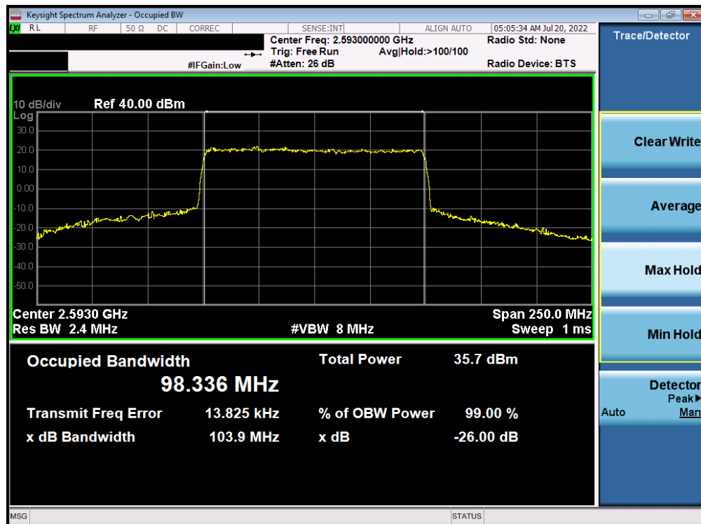
Plot 7-129. Occupied Bandwidth Plot (NR Band n41 - 100MHz CP-OFDM 64-QAM - Full RB)
