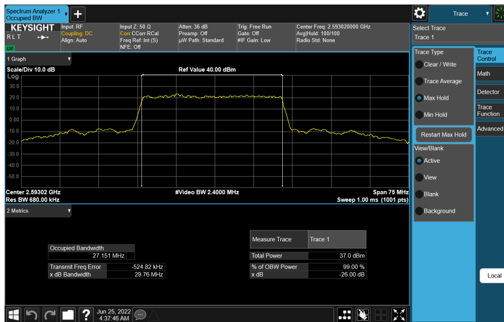
Plot 7-91. Occupied Bandwidth Plot (NR Band n41 - 30MHz DFT-s-OFDM \pi/2 BPSK - Full RB)
