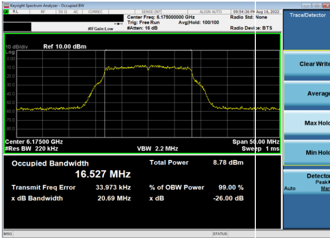
Plot 7-1. 26dB & 99% Bandwidth Plot Antenna 5b (20MHz 802.11a (UNII Band 5) – Ch. 45, 12Mbps)
