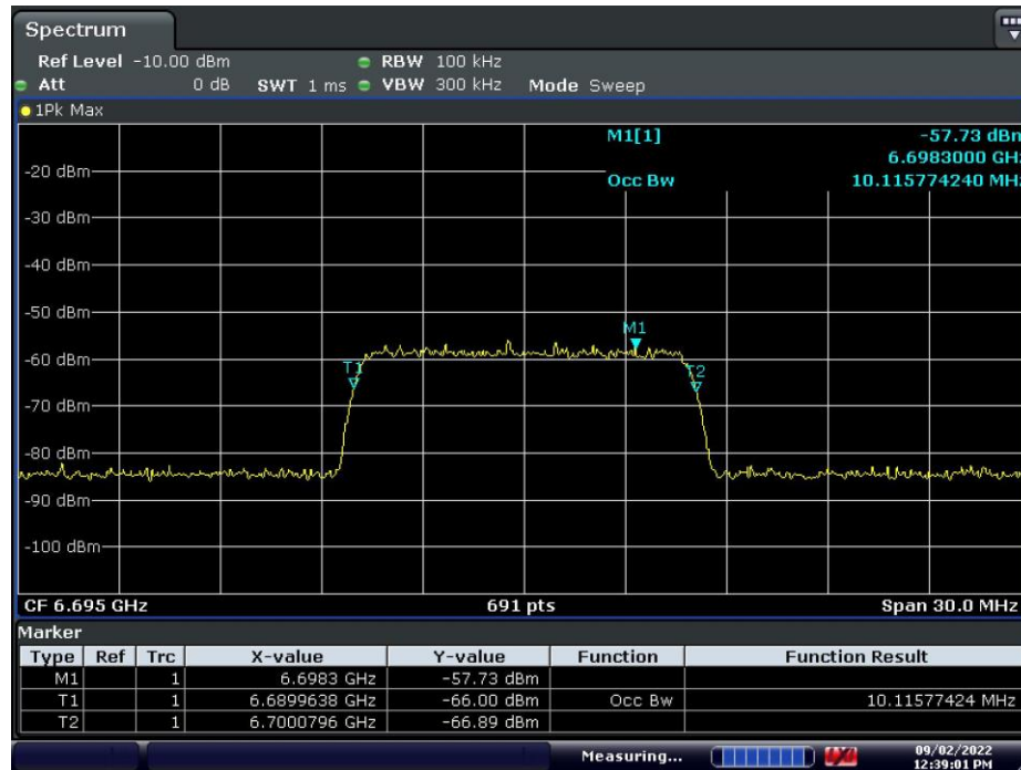
Plot 7-561. AWGN Signal – UNII 7 – 20MHz
