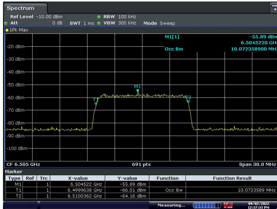
Plot 7-559. AWGN Signal – UNII 6 – 160MHz – Mid
