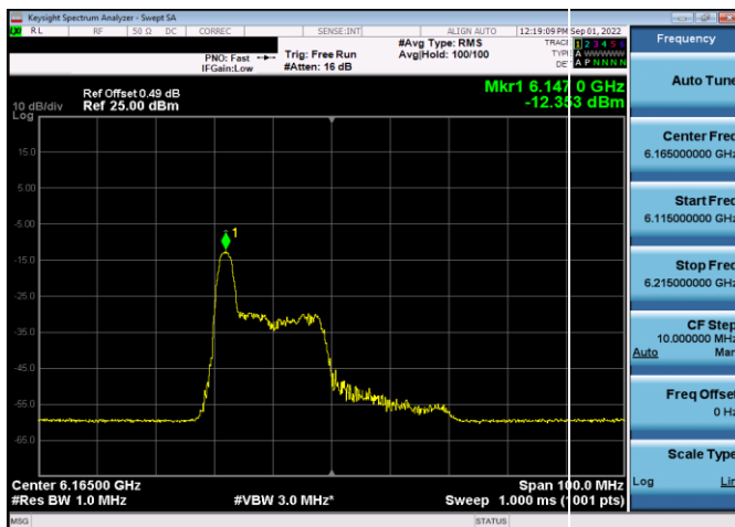
Plot 7-265. Power Spectral Density Plot SDM Antenna 5b (40MHz 802.11ax RU26 (UNII Band 5) – Ch. 43)
