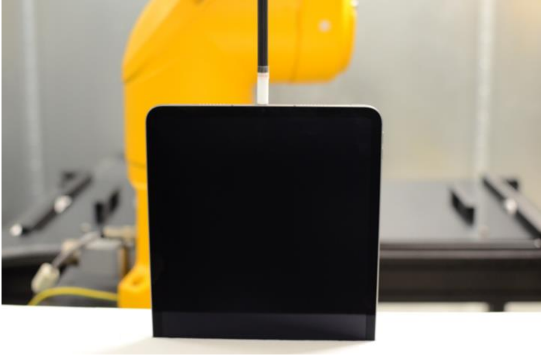
Figure D-4 Near Field Power Density Test Setup Photo – Top Edge at 2mm
