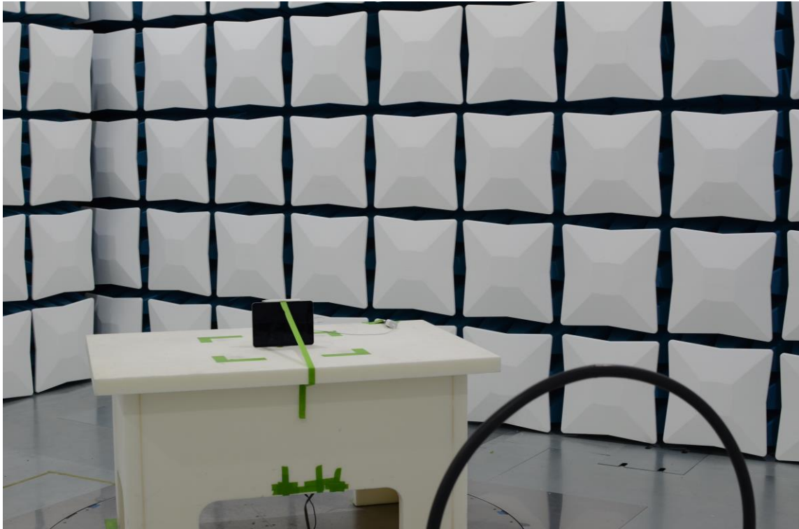
Figure 25: 9kHz-30MHz Test Setup (Front View)
