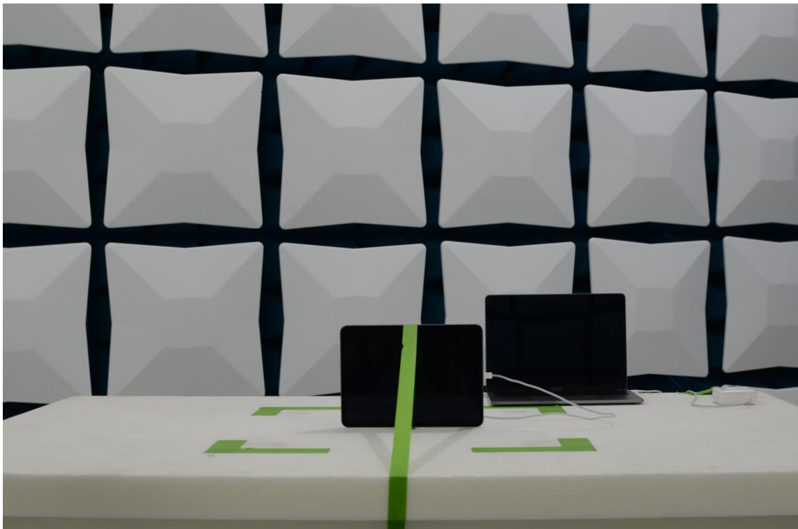
Figure 20: 30MHz-1GHz Test Setup (Front View)
