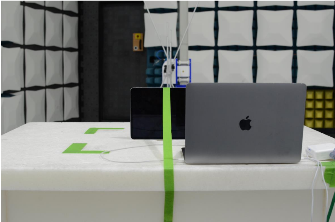
Figure 21: 30MHz-1GHz Test Setup (Rear View)
