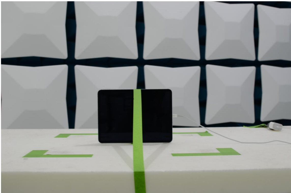
Figure 14: 30MHz-1GHz Test Setup (Front View)
