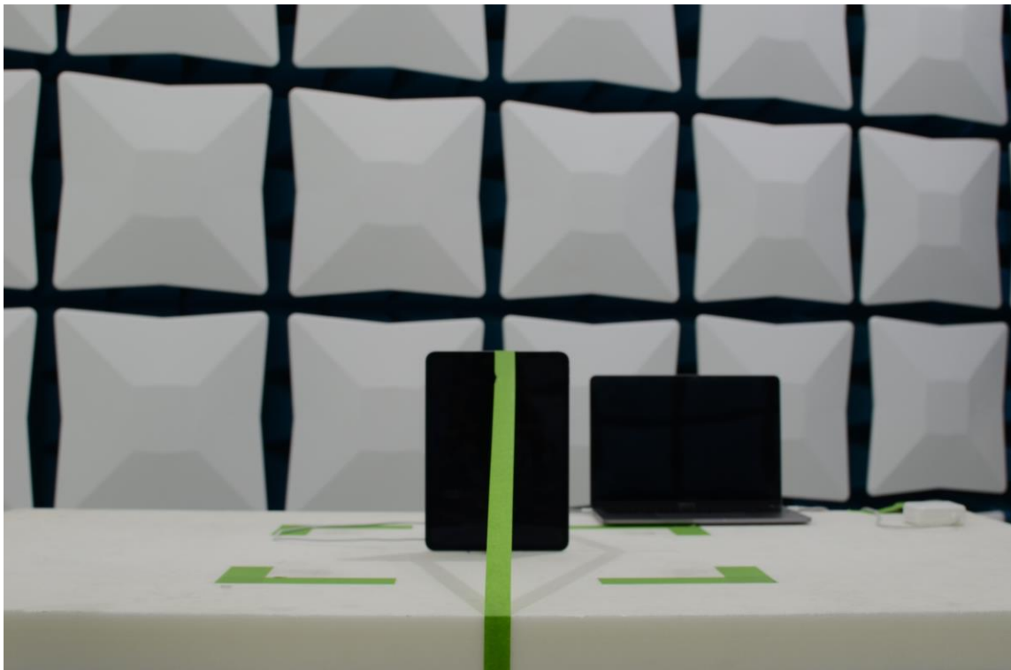
Figure 22: 30MHz-1GHz Test Setup (Front View)
