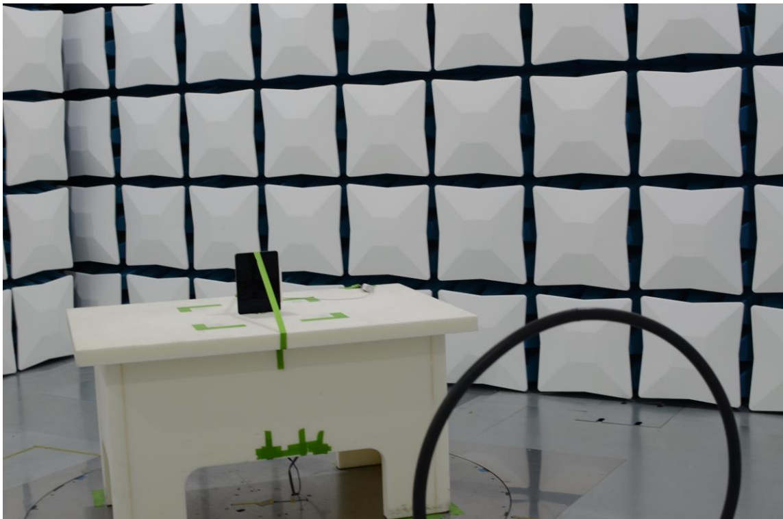
Figure 26: 9kHz-30MHz Test Setup (Front View)
