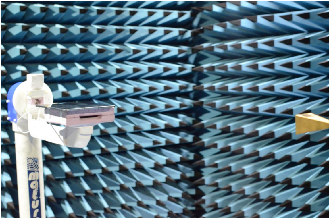
Figure 2: 40-60GHz Test Setup
