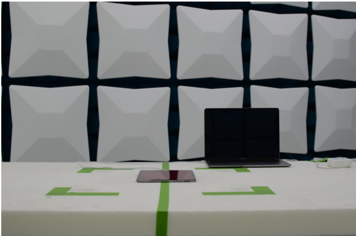
Figure 18: 30MHz-1GHz Test Setup (Front View)
