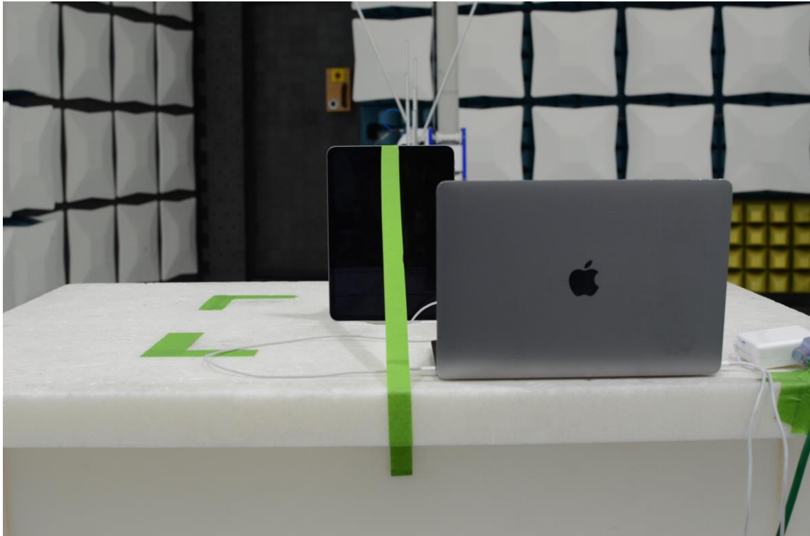
Figure 23: 30MHz-1GHz Test Setup (Rear View)
