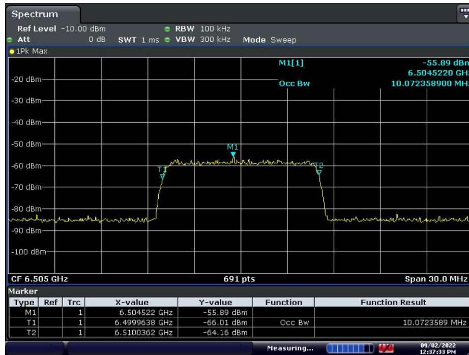
Plot 7-559. AWGN Signal – UNII 6 – 160MHz – Mid
