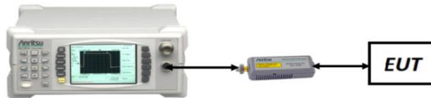
Figure 7-2. Test Instrument & Measurement Setup
