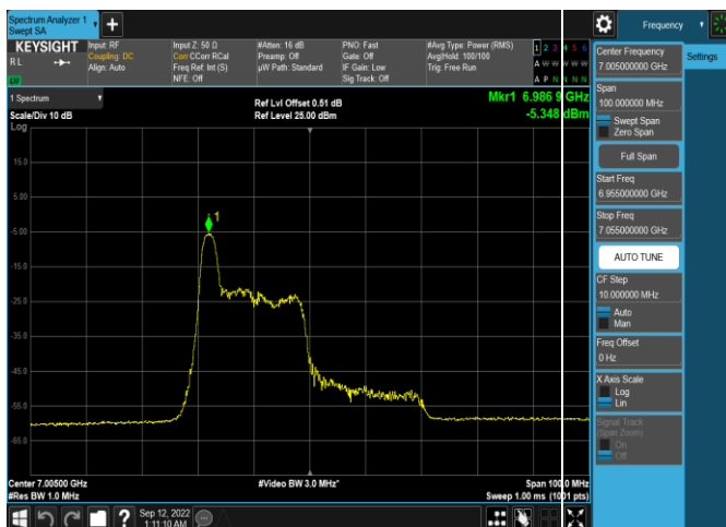
Plot 7-361. Power Spectral Density Plot SDM Antenna WF5b (40MHz 802.11ax RU26 (UNII Band 8) – Ch. 211)
