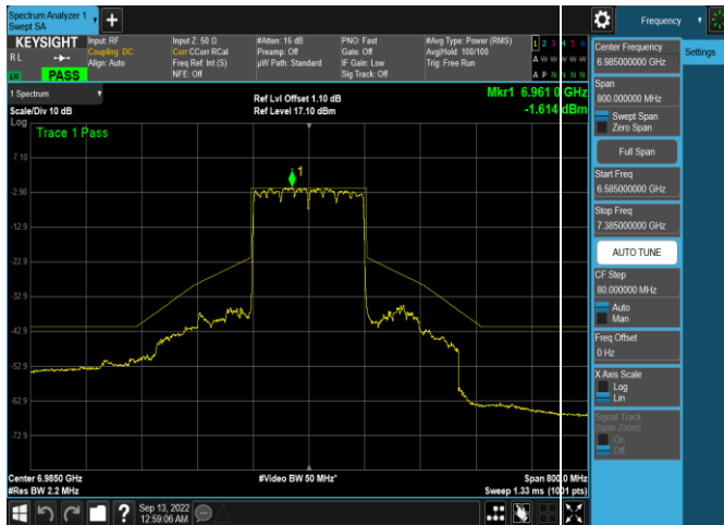
Plot 7-452. In-Band Emission Plot Antenna WF5b (160MHz 802.11ax (UNII Band 8) – Ch. 207, MCS11)
